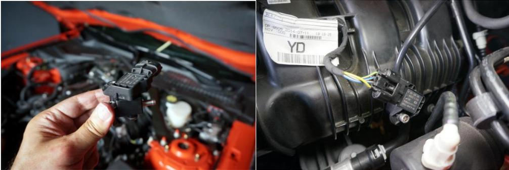
10. Using the posi locks provided attach them to the original wiring loom making sure the grey end is attached to the oe loom.
