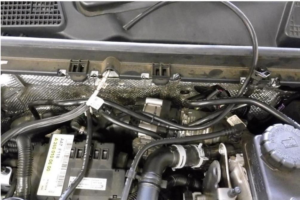
10. Mount the solenoid to the metal bracket with the M4 fasteners from the FMDV26 kit, use a 4mm Allen key to do this. Note the orientation of the solenoid when mounted to the bracket.
