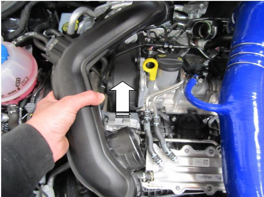
6. Remove the factory o-ring from the coupler on the OEM boost pipe and place into the Forge Motorsport billet throttle body coupler.
