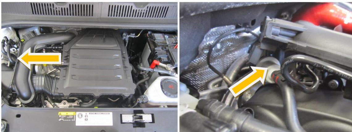
4. Unclip the couplers from the turbo inlet and throttle body while pulling them away from situ.
