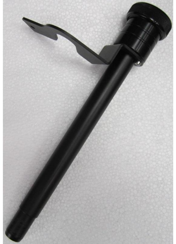
5. Carefully insert the small end of the tube (lubricate if required) in to the lower screen wash reservoir.
