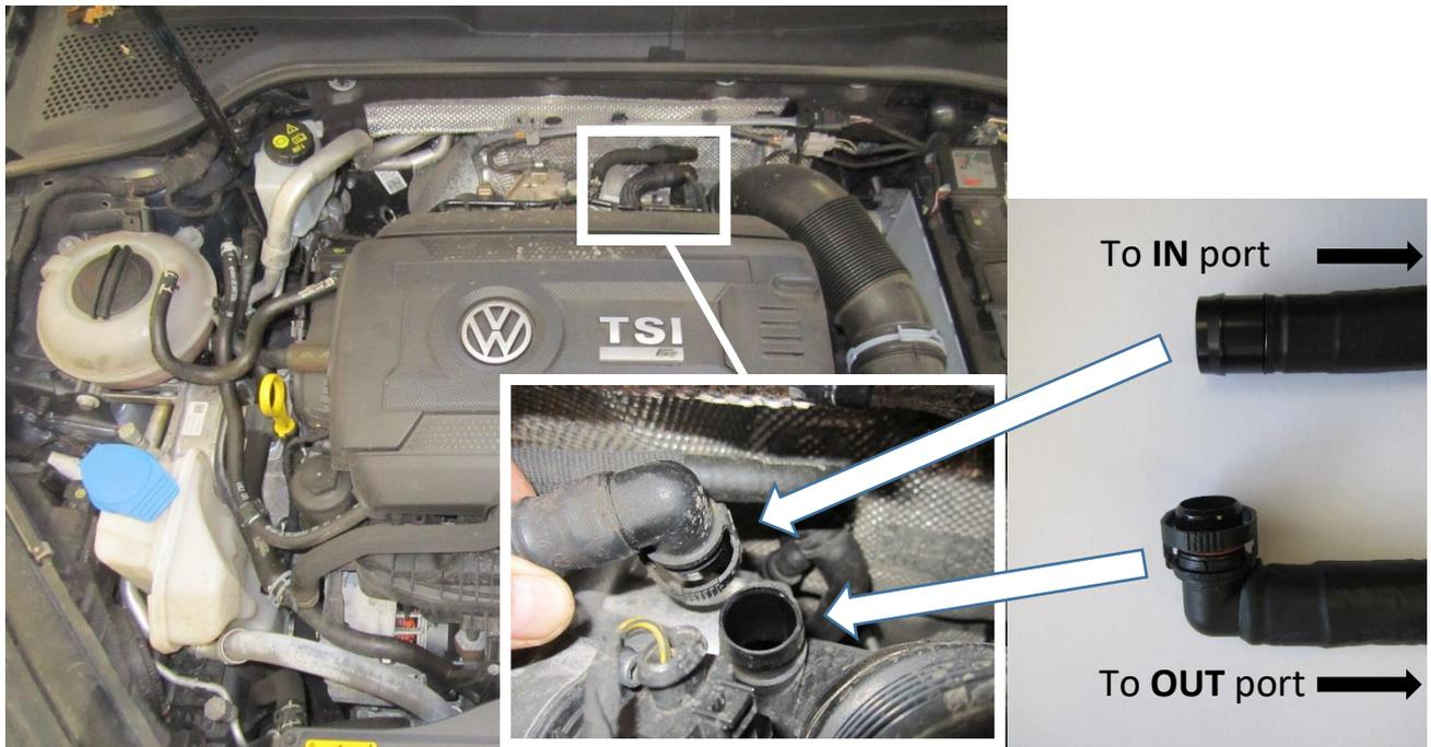
9. Once the hoses are neatly routed, attach supplied dual hose clamp and finally tighten bolts from Step 7. If you have fitted FMCTMK7WB then top up the screen wash fluid until visible in Forge bottle.
