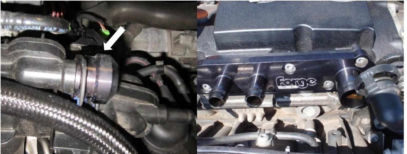
4. Remove the screw from the clamp (arrowed below), insert the lower catch can bracket and refit the screw.
