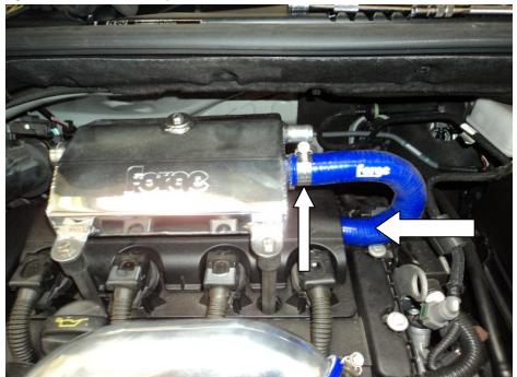
6. Now fit one end of the long silcon pipe to the rear outlet on the oil catch can and the other end to the turbo intake pipe. Use the number 30 hose clamp for the catch can end and hose clamp number 35 for the turbo intake end. Tighten both clamps with a hose clamp joiner.
