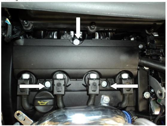
2. Fit the three long thread extension columns from where you removed the 10mm bolts in step 1. Place the smaller one of the three at the rear of the engine and the two longer ones at the front by screwing in and tightening gently using a 13mm spanner. Then screw the three rubber gromets onto those.
