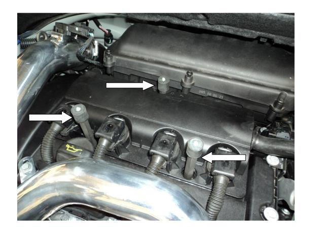
3. Place your new oil catch can onto the thread extension columns locating the three holes. Using the one longer bolt and washer, place that into the rear hole on the catch can. Now place the two small 10mm bolts and washers on the front of the catch can and tighten all three with a 10mm socket and matching ratchet.
