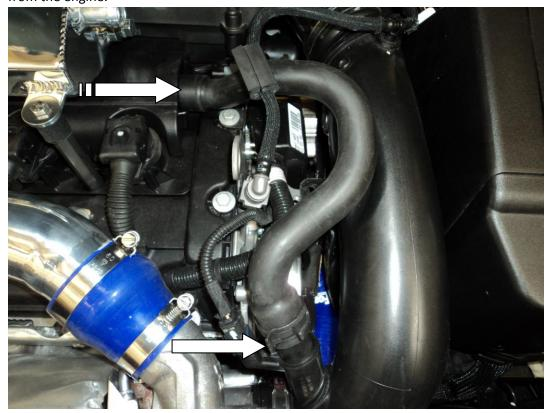
5. Place the small U-shaped silcon hose onto the breather port of the engine and the other end onto the front outlet on the catch can. Place the number 30 hose clamp over the pipe and tighten with a hose clamp driver.
