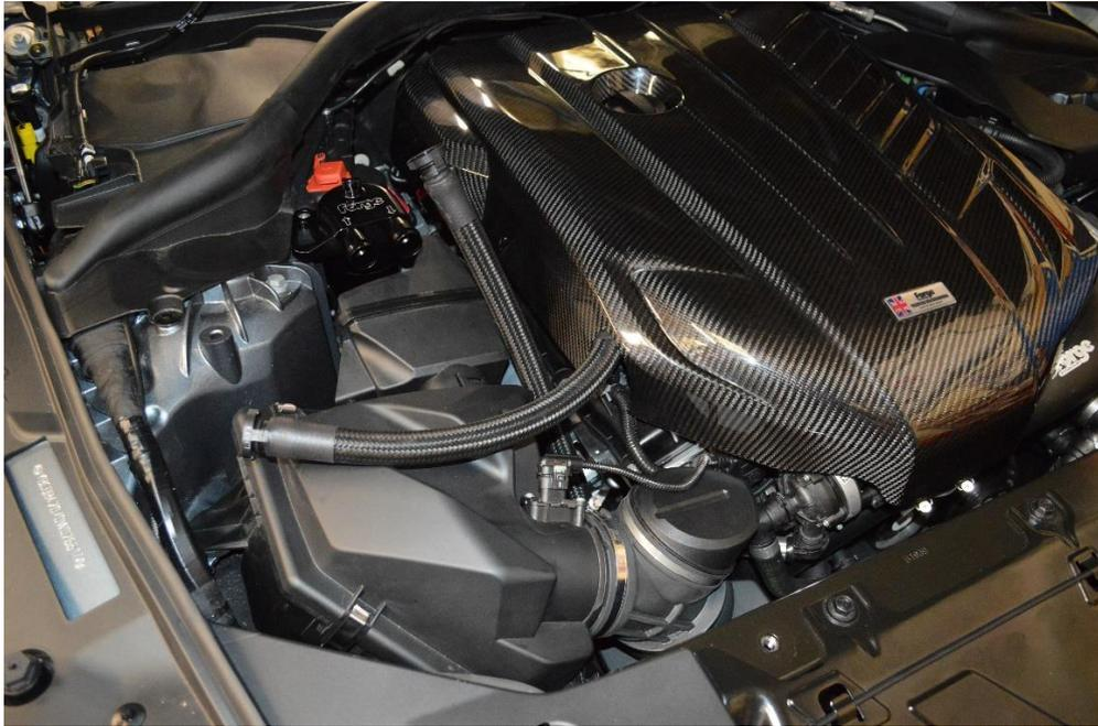
13. Fit the breather hoses to the catch can, the hose from the cam cover locates to the IN and the hose connected to the intake pipe locates to the OUT of the catch can.
