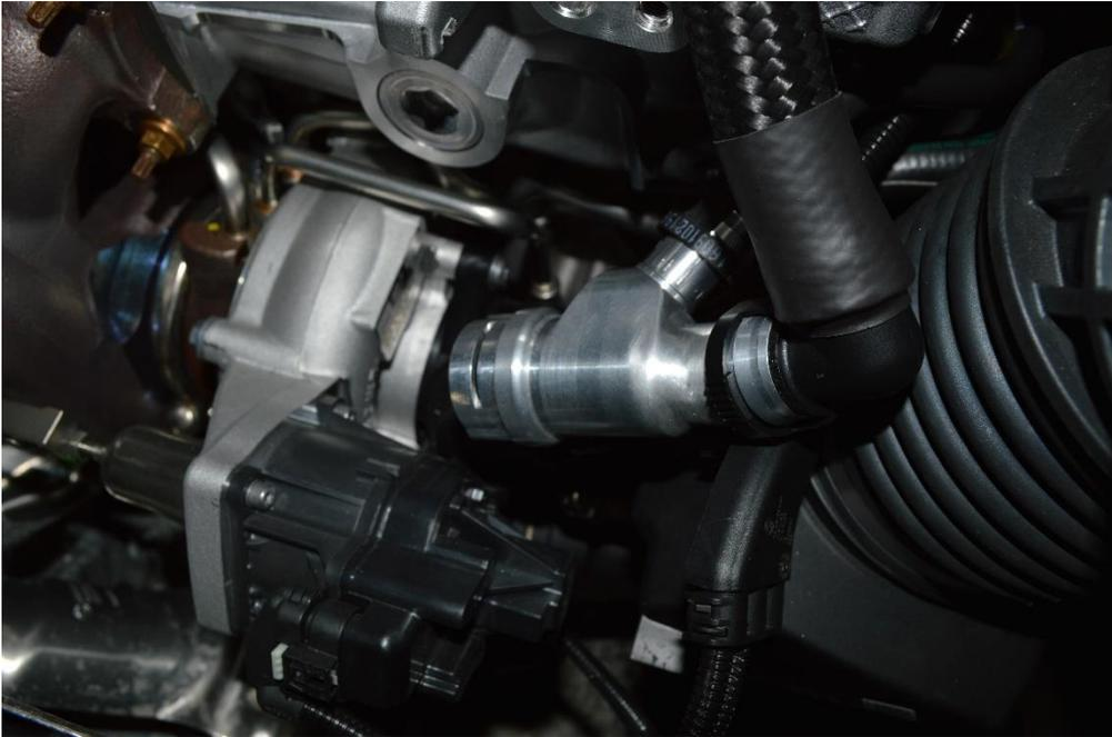
9. Insert the retaining clip removed in step 7, this will just slide into place.
