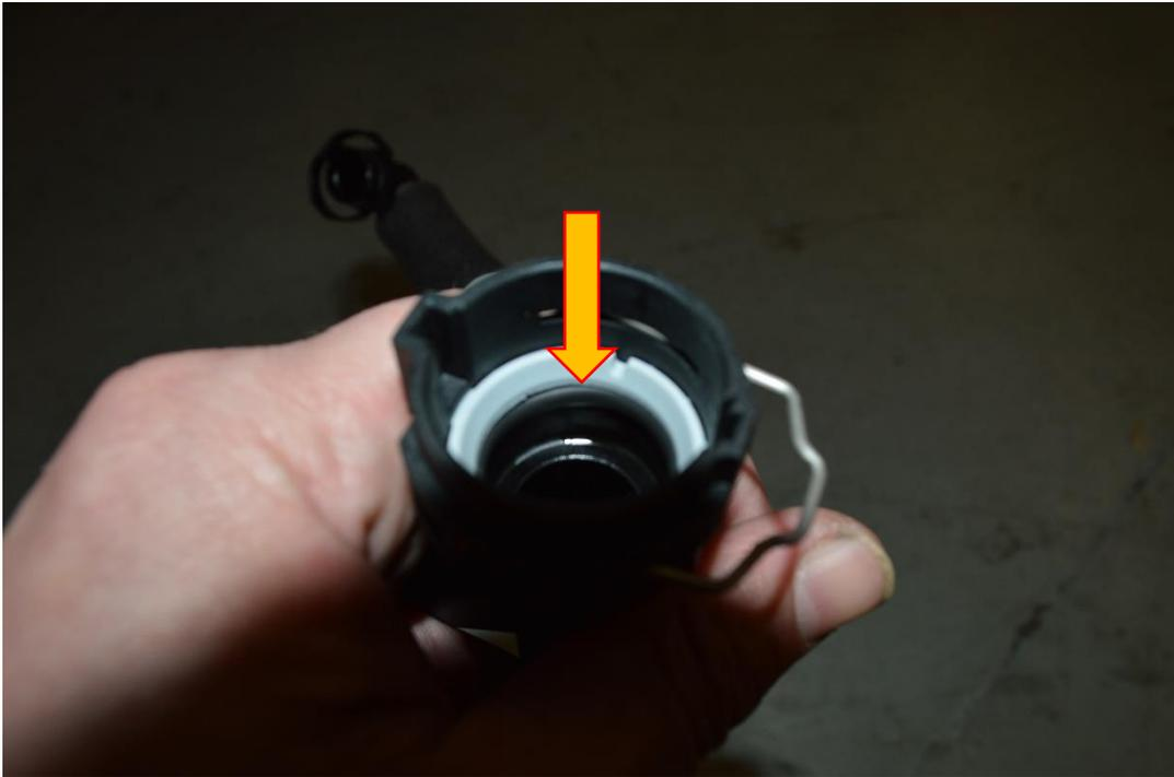
6. Insert the O-ring removed from the previous step into the O-ring groove in the Forge Breather adaptor.
