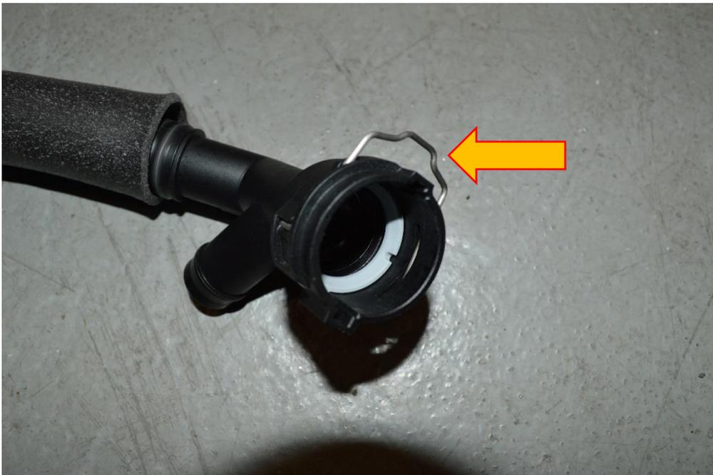
8. Insert the Forge machined breather adaptor onto the intake pipe, connect the small breather pipe to the smaller spout. Fit the LONGER hose from the FMCT6 kit with 45 degrees Norma fitting to the remaining spout.
