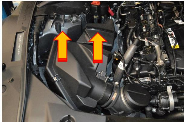
3. Locate the breather hose on top of the cam cover, squeeze the sides of the Norma fitting to release it.
