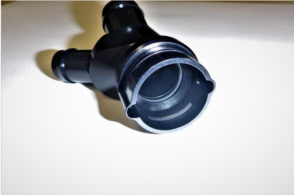
7. Remove the original retaining clip from the OE breather pipe, prise it out with the use of a flat blade screwdriver.
