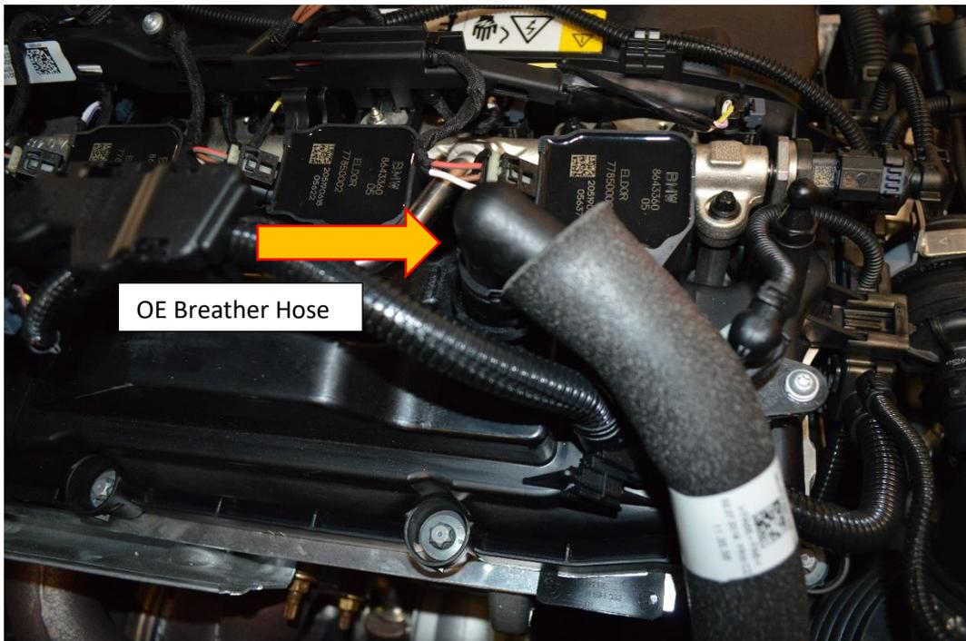
4. At the other end of the breather pipe you will see it has a Y fitting, disconnect the smaller breather pipe by releasing the Norma fitting as in the previous step. To remove the remaining breather pipe from the intake hose, release the retaining clip with the use of a flat blade screwdriver.
