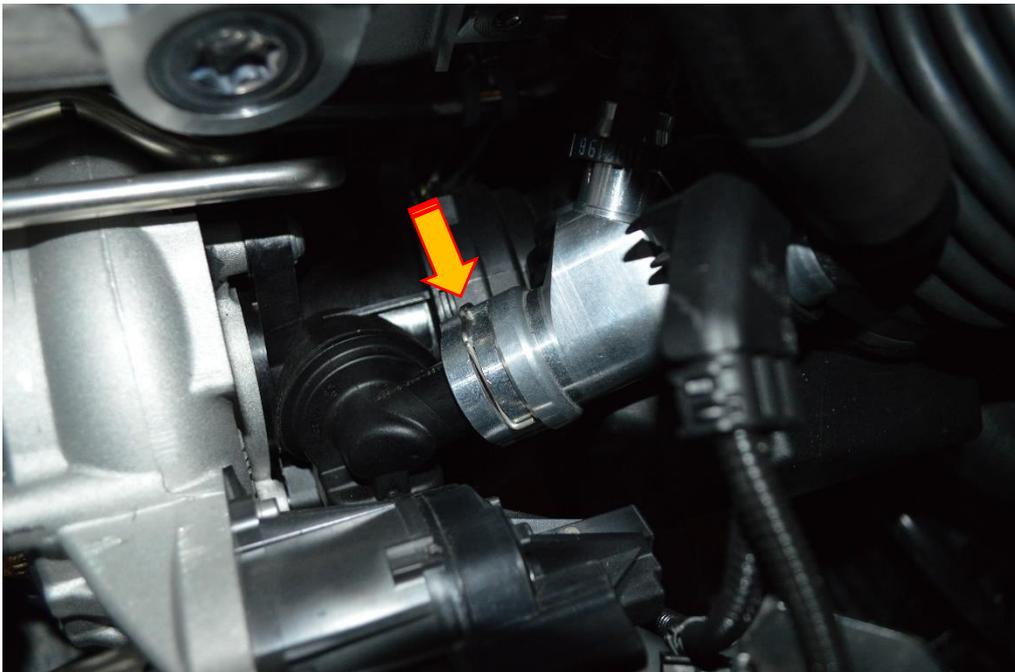
10. Fit the remaining shorter hose to the cam cover breather spout. Remove the fastener located next to the jump start point, use a T25 Torx drive to do this.
