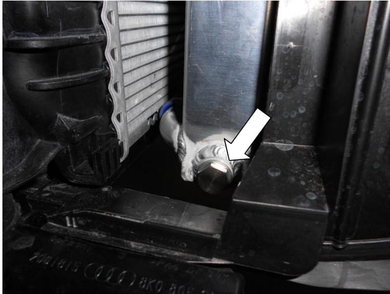
38. Undo the bleed screw located on the top R/H side of the charge cooler radiator. Fill the expansion tank with coolant until the coolant starts to appear at the bleed hole, then refit the bleed screw and sealing washer.
