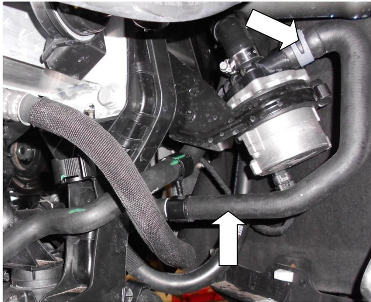
36. Using the remaining silicone hose in the kit, connect the top radiator outlet to the return from the charge cooler hard pipe and secure with suitable hose clips. Using the remaining 28mm P-clip, M6x12mm Allen head bolt and M6 washer to secure the silicone hose to the side of the radiator.
