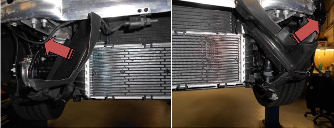
14. Unclip the other end of the charge cooler radiator and remove from the vehicle.
