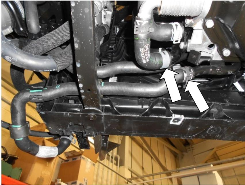
B) 2x Hoses on the pump inlet and outlet.
