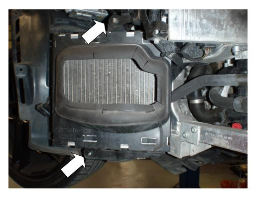
12. Using a Flat-blade screwdriver or panel clip tool carefully remove the plastic shroud from the outside of the OEM radiator. Take care not to damage any of the plastic clips.
