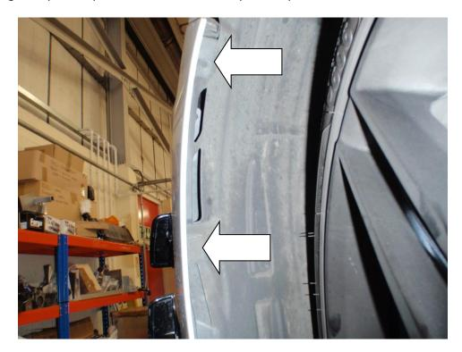
7. Undo 3x 8mm screws and remove air intake scoop.
