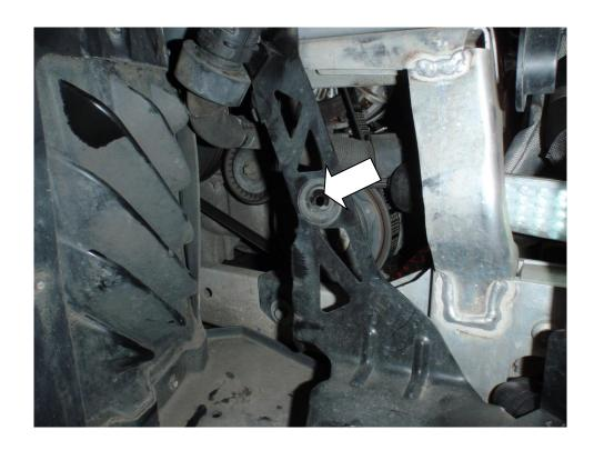
15. Mark the bracket in the position shown and trim off using a Hacksaw blade or similar tool.
