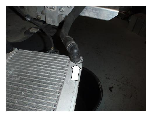
14. Undo hose clip and remove it from the metal bracket.
