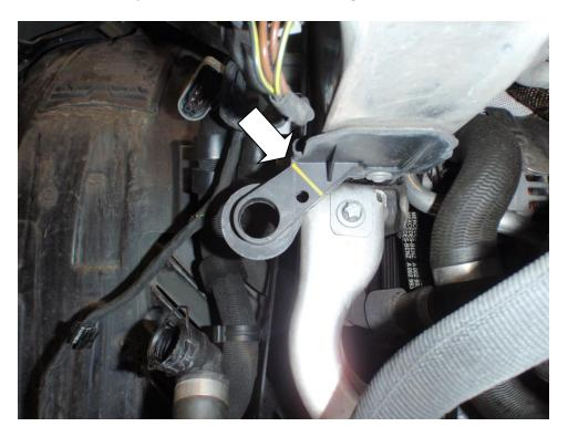
16. Fit the OEM plastic shroud to the Forge V-Mount radiator, ensuring that all the clips engage.
