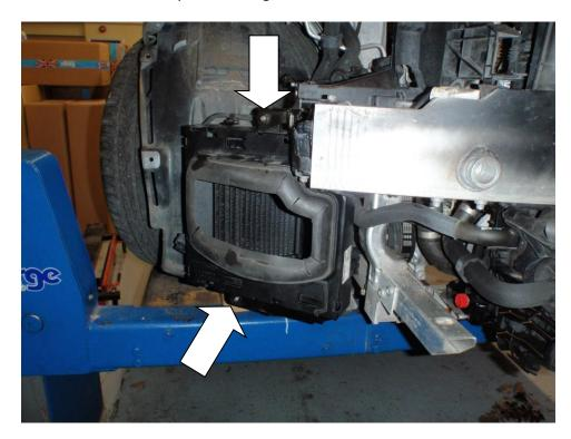
19. Refill the chargecooler reservoir tank with suitable coolant to the correct level and bleed the centre radiator before refitting the bumper.
