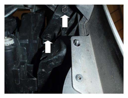
10. The next part requires two people to carefully pull the bumper away from the vehicle. While one person holds the bumper, the second person needs to reach inside and disconnect the temperature sensor and large electrical connector (located on the left-hand side of the vehicle viewed from the front).
