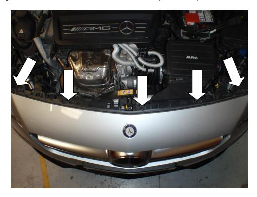
6. Using a flat panel-clip tool or similar remove 2x plastic clips from each arch liner.
