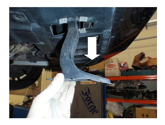
8. From the underside of the vehicle, undo 7x 8mm screws.
