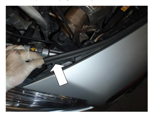
5. Using a T25 Torx driver undo the 5x screws across the top of the bumper.
