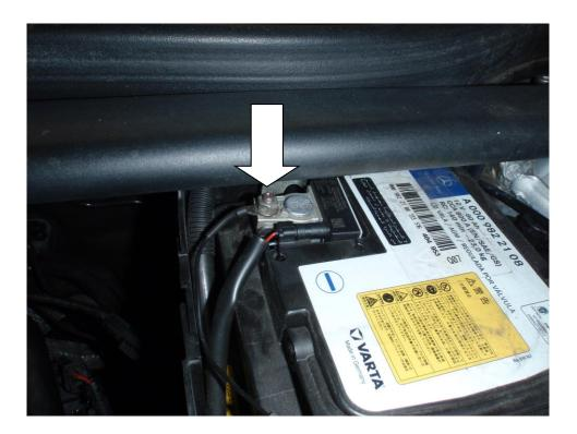
Note: Failure to correctly disconnect the battery may cause issues with the crash protection system (SRS) and the ECU.
