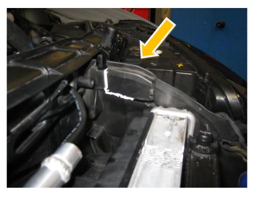
**22.** Where the lower Forge Motorsport charge cooler radiator lower pipe sits, a 40 mm hole must be drilled in the cowling as per the picture below .
