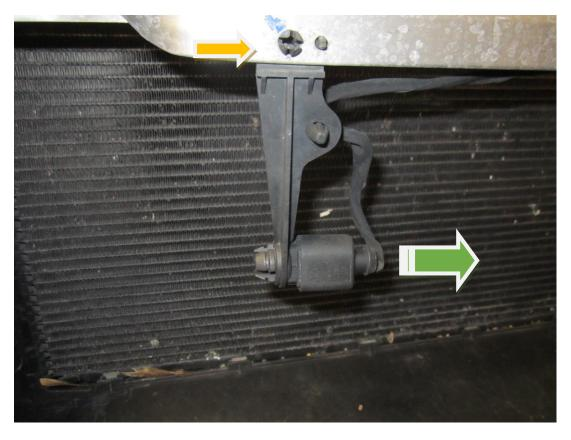
**16.** Using a 13mm spanner and socket remove the 13mm bolts either side of the crash bar that hold it in place, then fully remove.
