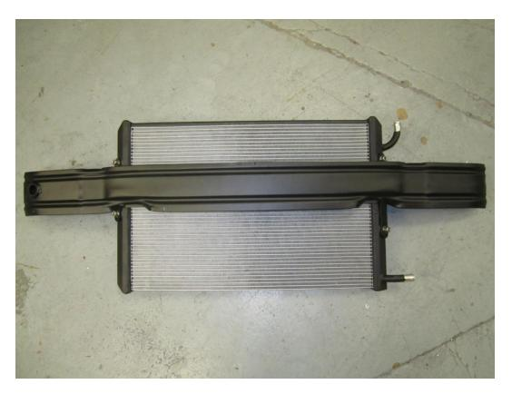
**19.** We found it helped to pry the crash bar mounts open slightly before loosly mounting your new Forge Motorsport charge cooler radiator in place.
