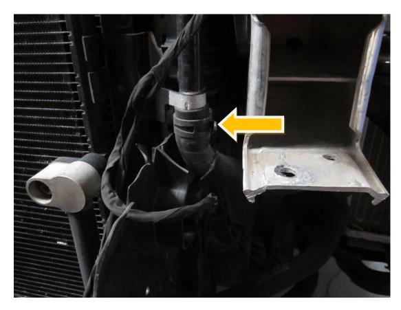
**21.**Trim part of the cowling with a sharp knife as per the picture below. This is to enable space for the new silicon charge cooler pipe .
