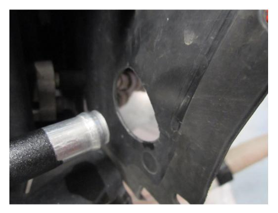
**23.** Fit the new Forge Motorsport silicon lower charge cooler hose into position and tighten the hose clamps both ends .
