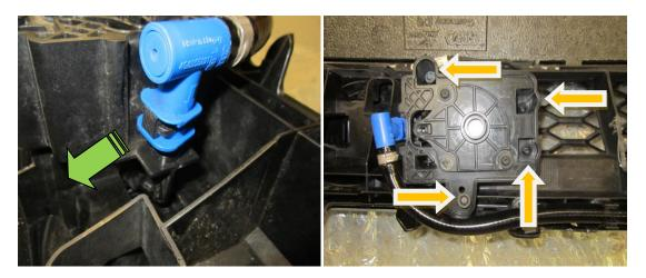
**28.** Taking care, with a sharp knife cut the washer jet pipe as pictured below then insert the 10mm blanking plug and secure in place with the hose clamp provided.
