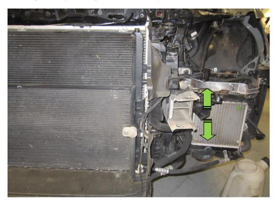
**20.** Remove the lower charge cooler hose arrowed in the picture below. You WILL lose the coolant within your OEM charge cooler radiator so a clean container is advisable to catch this in, then you can either re-use or dispose of correctly.
