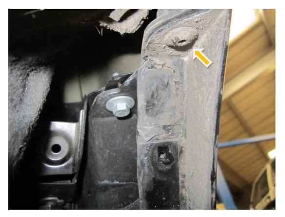
**8.** Pulling the arch away from the wing and towards the front of the car and unclip the sides of the bumper .
