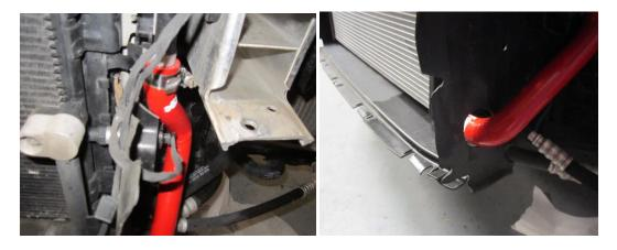
**24.** Now remove the upper chargecooler hose fully ,this is arrowed and pictured below.
