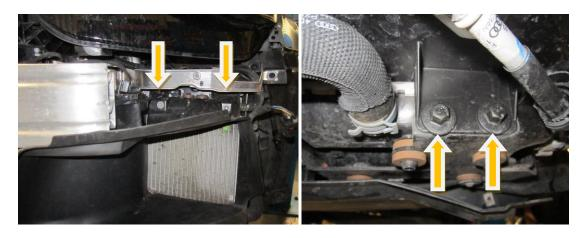
**13.** Using a T30 torx drive, loosen the fasteners that hold the headlight in place.
