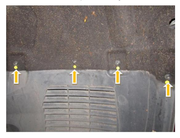
**6.** Again with your T25 torx drive remove the 7 fasteners that hold the lower arch spoiler in place to your undertray and arch liner.
