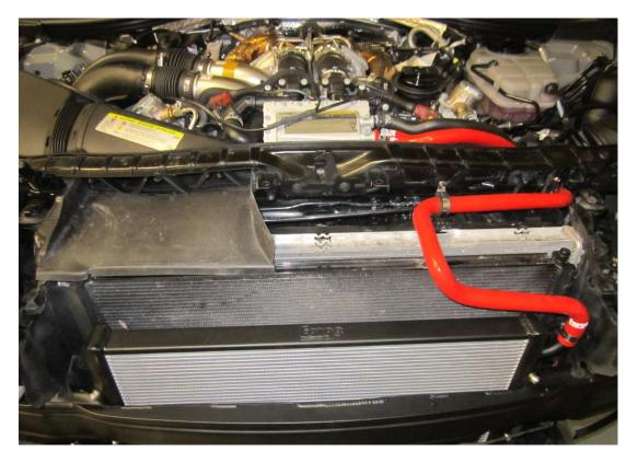
**26.** Fit the 25mm p-clip provided to hold the silicon hose in position.
