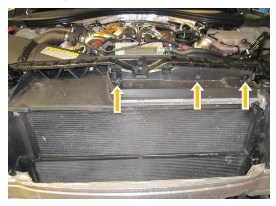
**12.** Remove the auxillary radiator ducting on the right hand side of the vehicle (when viewed from the front )using a T30 torx drive and a 10mm socket.
