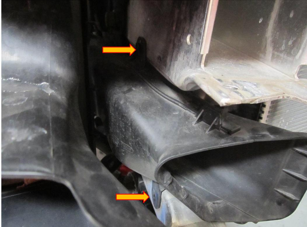
21. Place a drain pan or bucket under the offside hose going to the OE charge cooler in order to catch the coolant.
