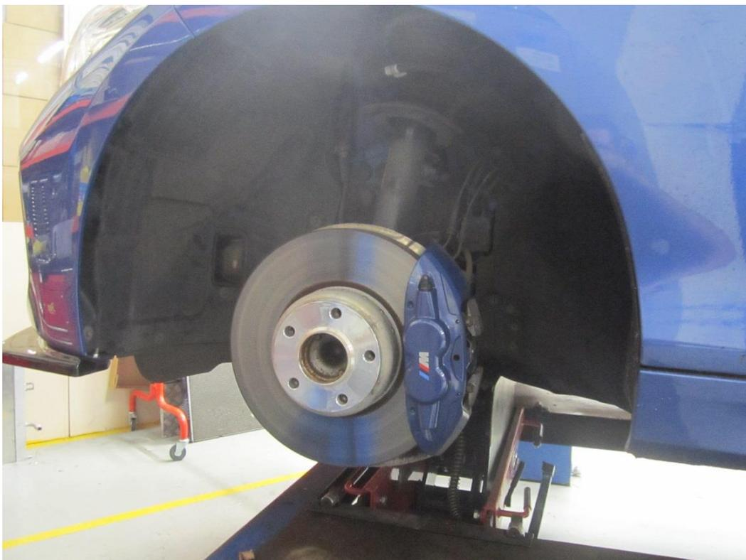
4. With the wheels removed, first locate all ten 8mm fasteners that hold the inner splash guard in place and remove them like before with the use of an 8mm socket and ratchet or spanner. The splash guard will now pull away from the vehicle. This also needs to be repeated on the opposite side of the vehicle.
