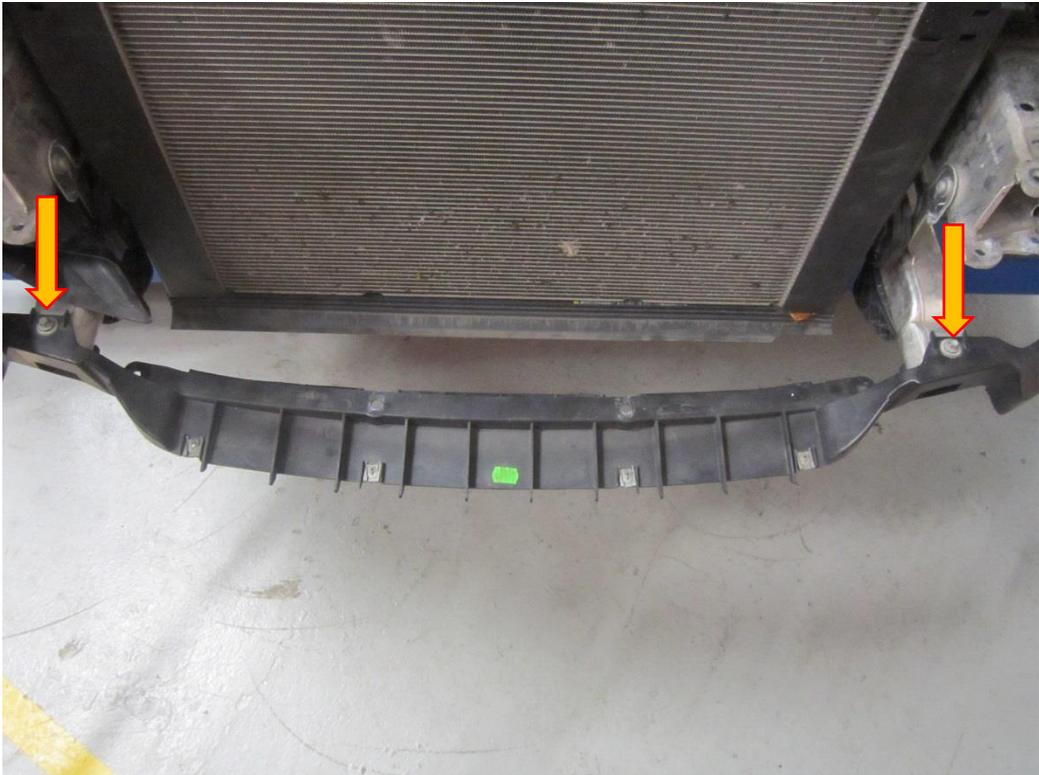
17. Undo and remove the two T27 Torx fasteners at the top of the radiator frame. There are two more T27 Torx fasteners at the bottom of the radiator frame on the underside, these also need removing, this bottom panel can be removed once you have un-clipped it from the coolant hose.
