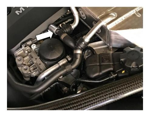
17. Using the 8mm I/D silicone x 750mm hose provided connect one end to the 8mm overflow pipe on the side of the expansion tank and secure with a suitable hose clamp. Route the other end of the pipe through to the underside of the car.
