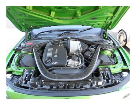
2. Pull the engine cover upwards to remove it from its mounts.
