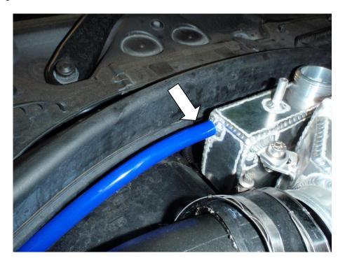
18. Using the remaining 8mm I/D Silicone x 170mm hose and 2x hose clamps connect the radiator neck to the expansion tank.
