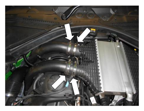
4. Disconnect the wiring to the MAP sensor and then use a 6mm socket or hose clamp driver to undo 1x hose clamp.
