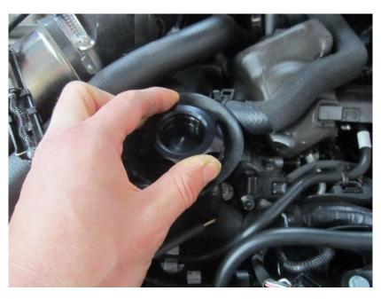
2. With the cap in place, either spray it with water or moisten it with a wet sponge to lubricate the cap. This will make fitting the insert much easier.
