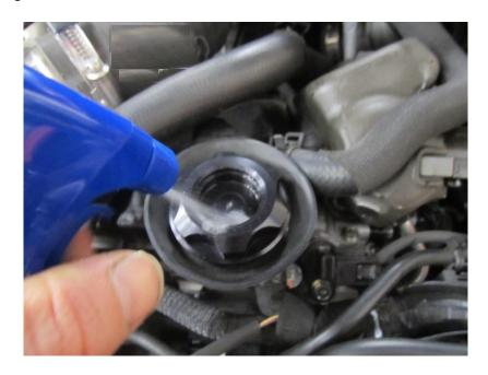
3. Now you will be ready to fit the cap insert. Below is a diagram on how the cap locates. Make sure that the rubber O-ring is in place.
