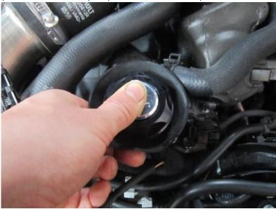
6. This is how you cap should look once you have fitted the insert into position. Note how the insert sits flush and is not raised in any way! Please be sure to tip the cap to the side with a small hole in so that any excess water will be removed.
