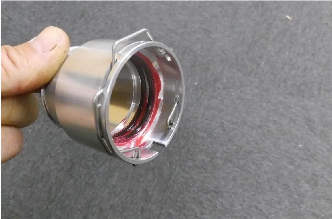
5. Fit the coupler to the turbo, it is a very tight fit so you may want to use a rubber mallet to tap it into place. Fit retaining clip from OE boost pipe once in place, as this will keep the coupler securely in position.
