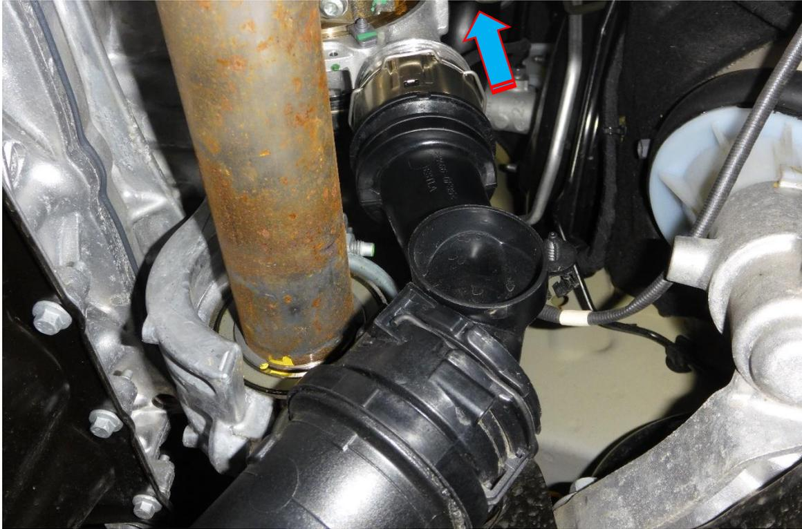
4. Remove the retaining clip from the OE boost pipe. Take the coupler from the FMBP6 kit and lubricate the O-rings as this will make fitment easier.
