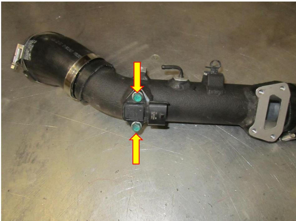
11. Take the FMBP4 hard pipe and attach the two silicon hoses as shown in the picture below. Do not tighten the hose clamps up as you may need to adjust the positioning of the hoses. Fit the map sensor using the OE M6 fasteners.
