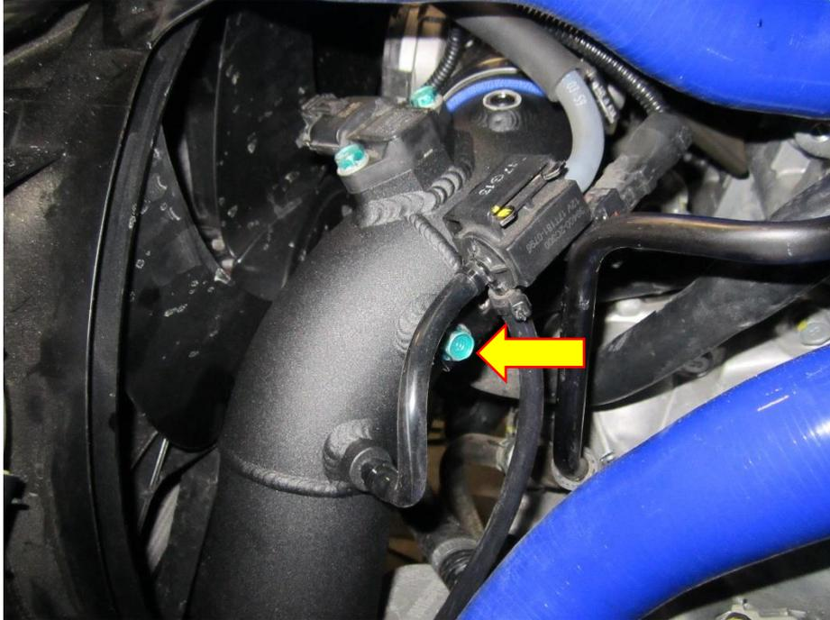
14. Re-fit the diverter valve and connect the vac hose, use the large cable tie to secure this vac hose to the lower radiator hose. Do not over tighten this as it can pinch the vac line.
