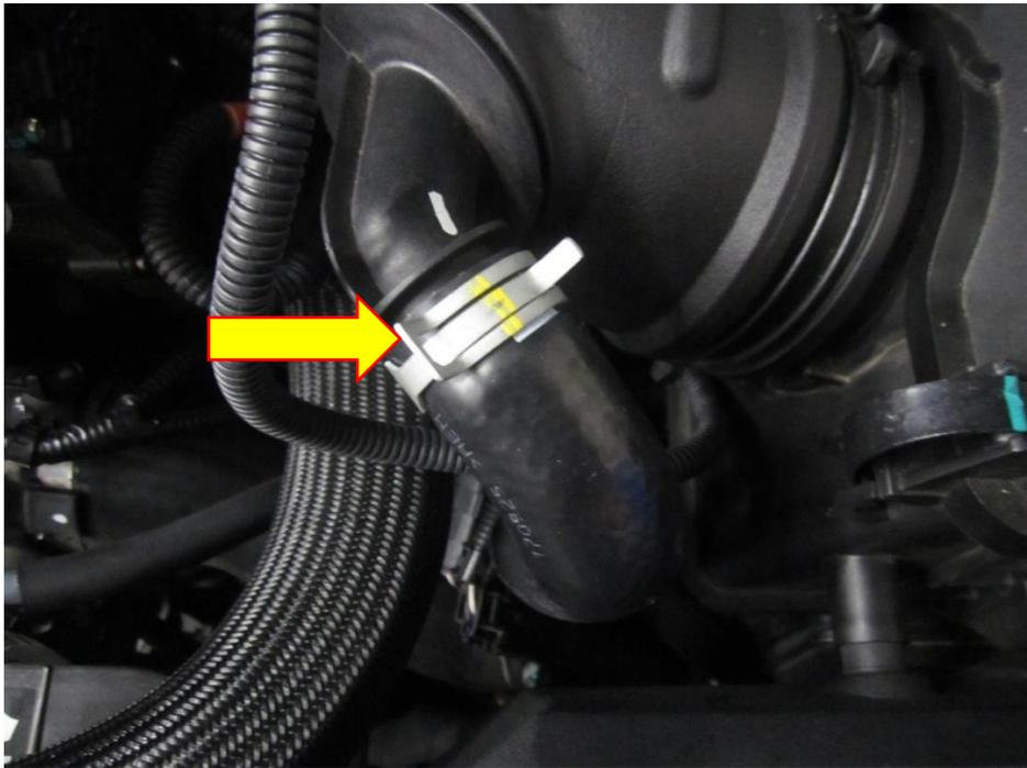
4. Moving to the other end of the OE intake Pipe there are two breather hoses that need to be removed, these too have spring hose clamps that just need to be compressed like step 3 to remove the hoses. Once this is complete undo the 10mm hose clamp attaching the intake hose and joiner to the turbo elbow, you will now be able to remove the air box and intake pipe together as one part.
