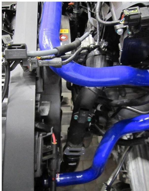
9. Release both hose clamps that attach the boost pipe to the vehicle, there is one which holds the rubber joiner hose to the throttle body and one which holds the 90 degrees joiner hose to the intercooler. Use an 8mm socket and ratchet or a flat blade screwdriver to undo both hose clamps. Some clamps may have a cover over the worm drive, this can be removed with plyers.
