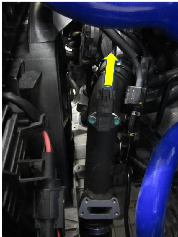
7. The short vacuum hose from the solenoid needs disconnecting from the OE boost pipe, like in previous steps release the spring clip and pull the vacuum pipe free. Remove the M6 fastener holding the solenoid to the OE boost pipe, use a 10mm socket and ratchet to do this.
