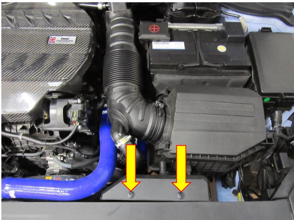
3. The spring clip holding the diverter valve return pipe to the intake hose needs to be removed. Using a spring clip removal tool or long nose pliers compress the spring clip so that you can slide it down the hose and remove from situ.
