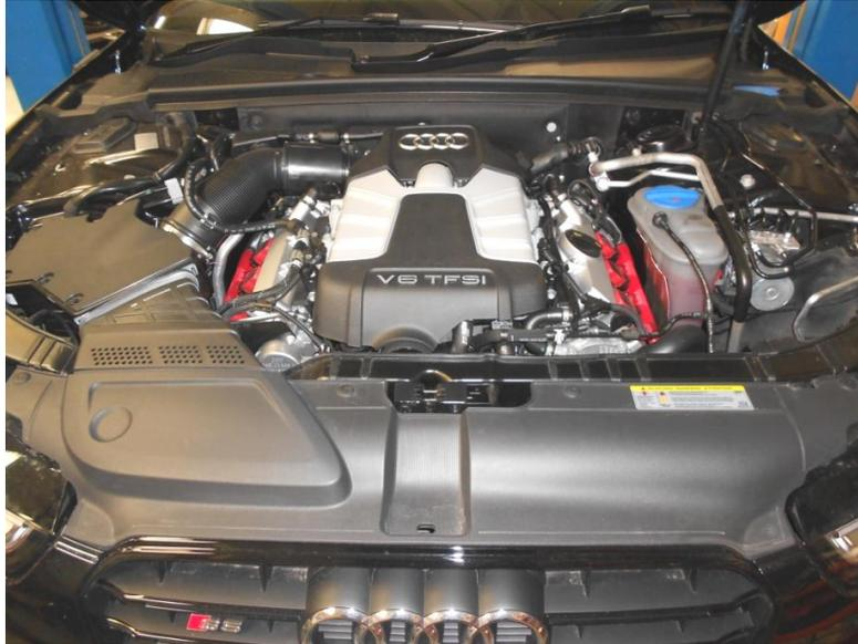
2. At the back on the engine carefully pull the plastic cover upwards.
