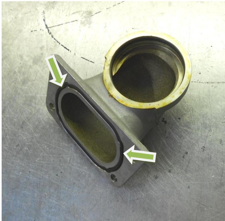
9. Test fit the cast elbow and boost tap without bolts to correctly align the holes in the cast elbow and billet boost tap.
