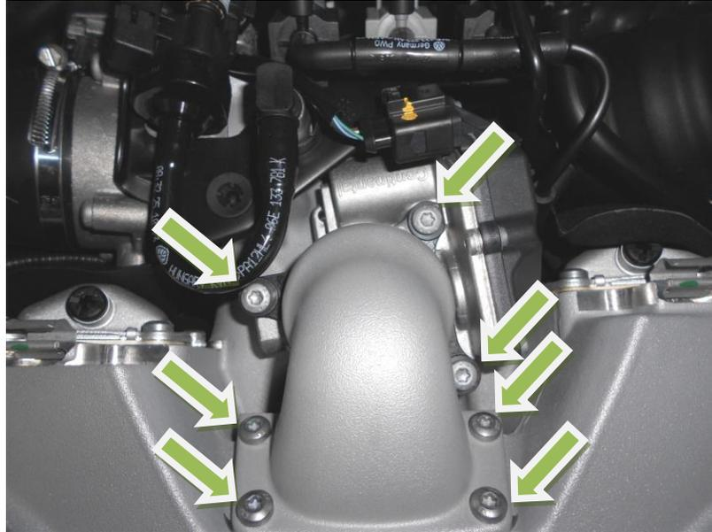
4. Carefully remove the cast aluminium elbow and plastic flange. Cover both openings to prevent foreign objects from falling in to the engine.
