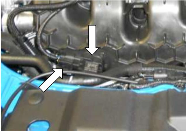
Lift and secure the bonnet and begin by removing the engine cover, this will give better access while carrying out the installation. Disconnect the wiring to the sensor.
