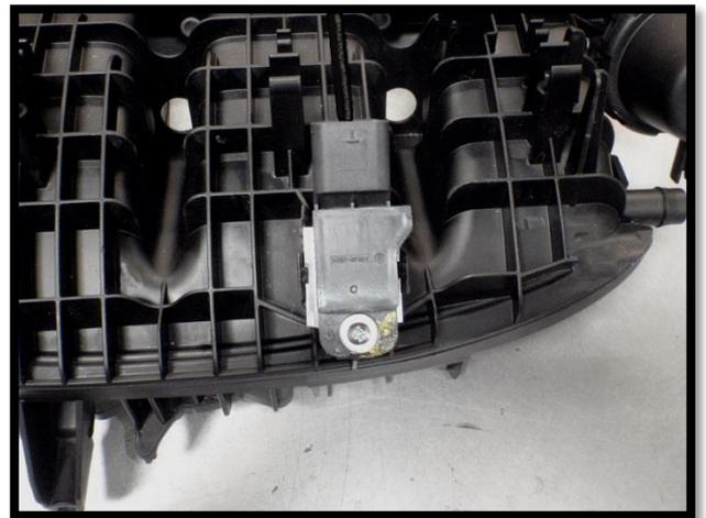
Step 4. Push the MAP sensor into the boost tap and using the screw and washer supplied in the kit tighten down.
