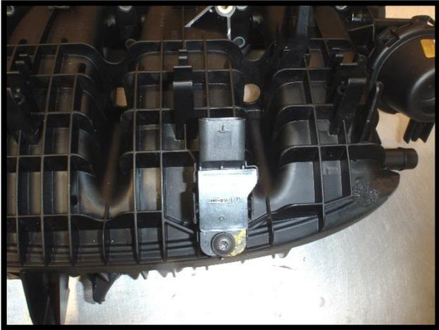
Step 1. Remove the MAP sensor from the inlet manifold.
