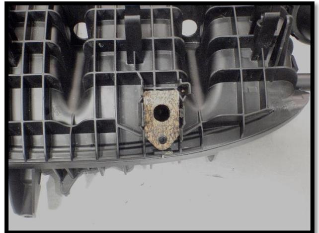
Step 2. Place the cork casket onto the inlet manifold.
