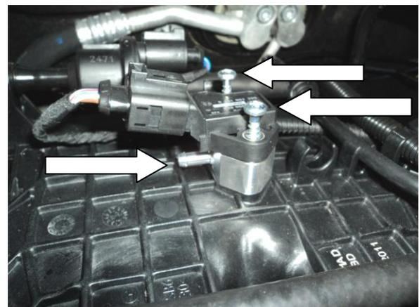
Fit the boost gauge take off using the longer screws provided. (Allen head bolts TTRS)
