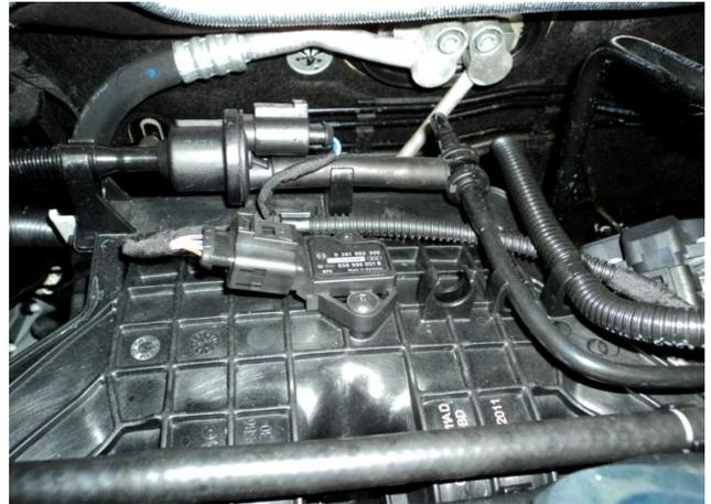
Remove the two T25 Torx head screws (Allen head bolts TTRS) and remove the map sensor
