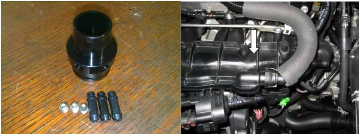
At the front right (transverse engines) you will see the OEM vacuum hose connector. By squeezing the sides of the OEM connector the locating clips are released so that the connector can be withdrawn.
