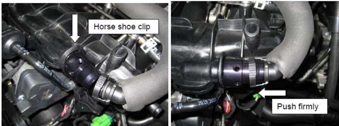
The Forge vacuum take-off adaptor is installed as shown. It is necessary to push the adaptor onto the spigot so that the retaining horse-shoe type clip can be slid into place fully (shown above with vacuum nipples removed for clarity).
