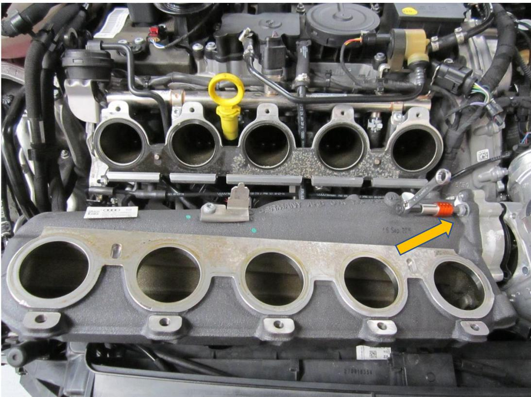
5. Remove the OEM throttle bodie spacer and fit the Forge Motorsport water meth and boost adaptor into position.
