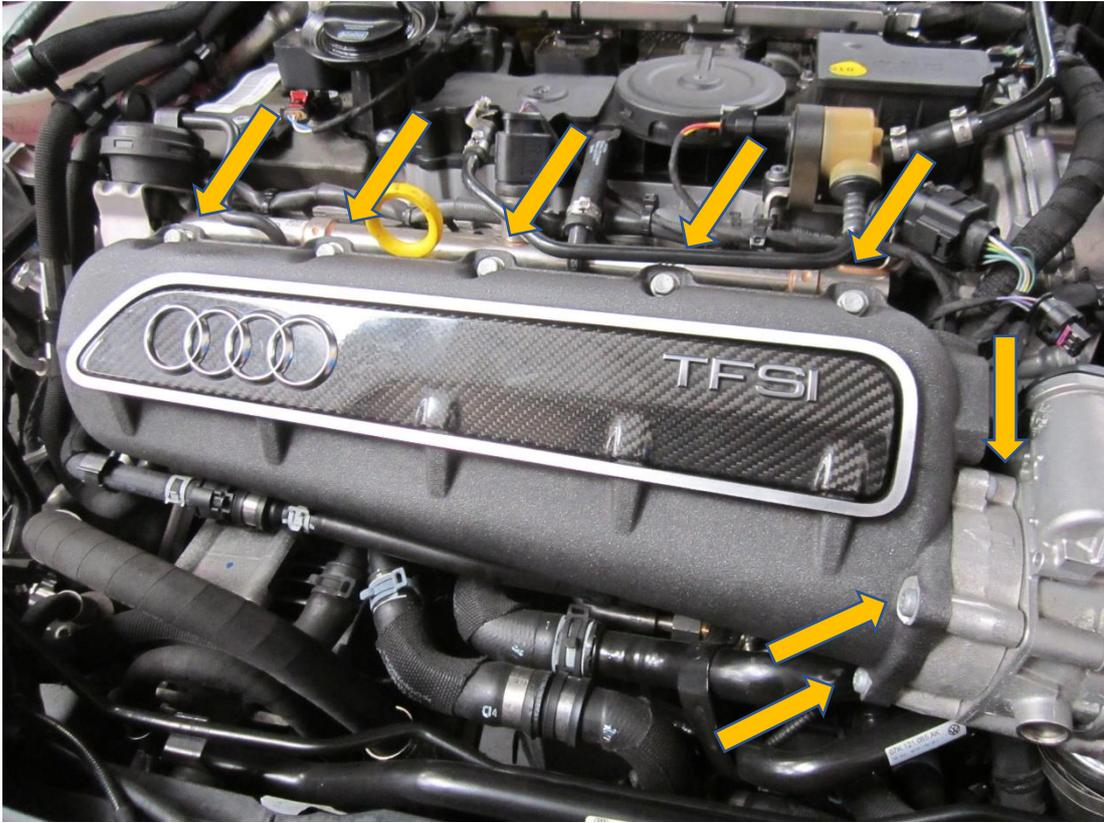
4. Split the inlet manifold to remove the last T30 fastener that holds the throttle body to the inlet manifold.
