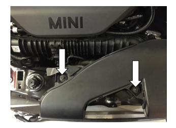
Lift the bonnet and begin by removing the intake scoop, this will give better access while carrying out the installation. Undo 2x 10mm nuts and unclip at the airbox.
