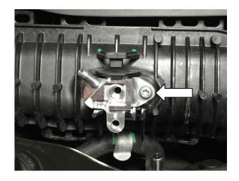
Ensure the O-ring supplied is fitted to your boost tap. Lubricate with a silicone spray before fitting to the manifold. Push the boost tap firmly into position and secure with the OEM screw.
