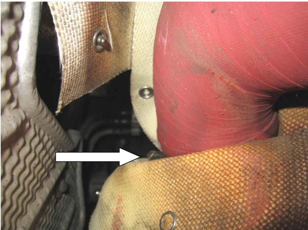
5/ Refit the new de-resonated charge pipe fitting the turbo end first then twisting it so that it fits perfectly in the locating brackets.
