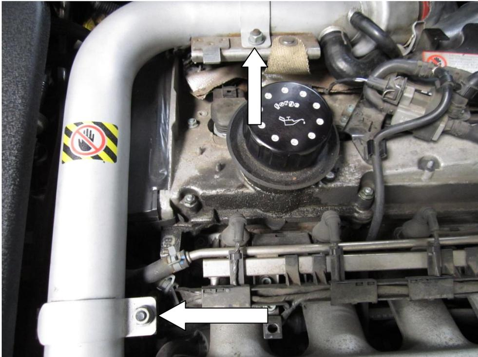
4/ Loosen off the hose clamp on the turbo hose **so that the hose can freely move round**. You may need to open the poppers on the heat shield.
