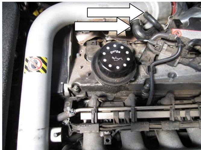
3 Undo the two 13mm nuts shown and remove the brackets.
