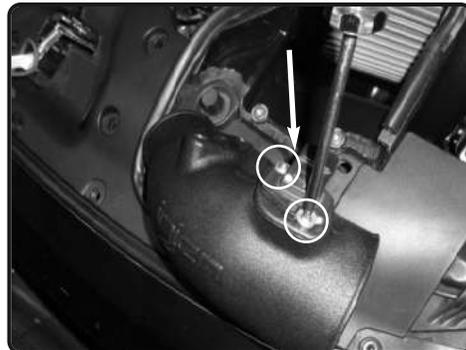
**26.** Now install to the new injen intake tube and secure using original screws. Secure and tighten.
