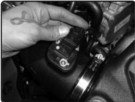
**29.** Re-connect the MAF sensor harness. Secure and tighten.
