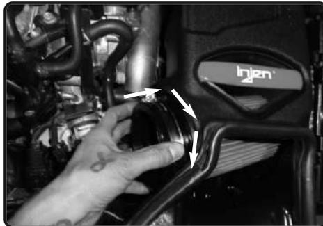
**22.** Once the twist lock filter is seated correctly rotate in either direction 1/4" turn until filter locks into place.
