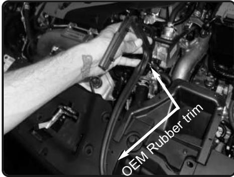
**13.** Remove the OEM rubber trim from the scoop using pliers. carefully pull out the clips holding in the rubber trim.
