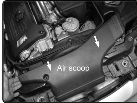
**25.** Re install the air scoop and secure from step 7.
