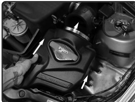
**17.** Install the air box assembly into position and connect the filter to the intake tube. Adjust and position if necessary.
