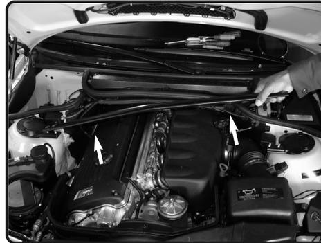
**2.** Once you have removed all four m12 flange nuts, continue to remove the strut tower bar.
