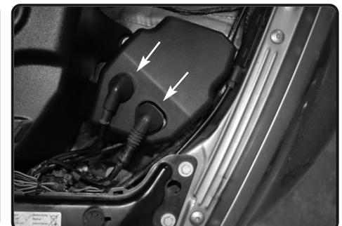
**23.** Re-install ballast cover, and reconnect both harness.
