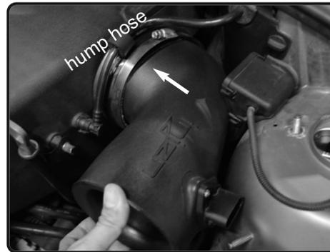
**14.** Install the intake tube and position the tube to the hump hose on the plenum. Do not tighten.
