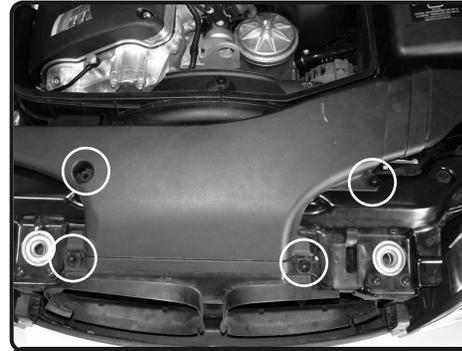
**7.** Removing the air scoop: Use a screwdriver to raise the center locking pin in the located on the clip. Remove all four plastic clips from the air scoop. Once you have removed the plastic clips, continue to remove the air scoop from the radiator shroud.
