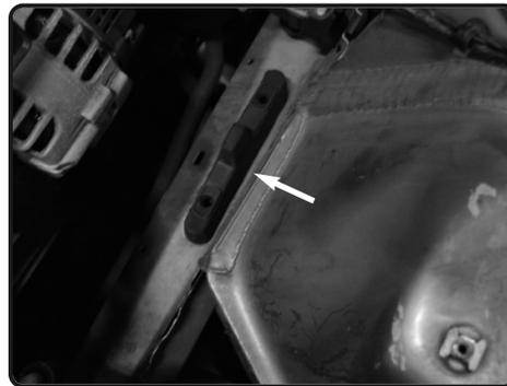
**13.** Make sure the rubber airbox isolator is installed on the vehicle frame, and is seated properly.
