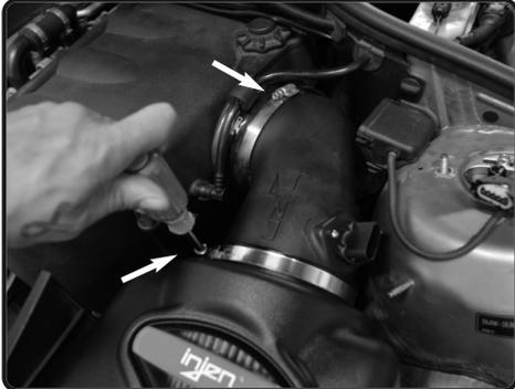
**24.** Tighten all clamps on the intake tube using 8mm nut driver.
