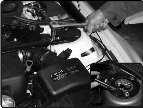
**1.** Loosen and remove two m12 flange nuts from each side of the strut tower bar. Remove the lower plate also, this will allow for more clearance.
