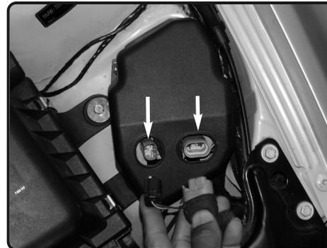
**6.** Press upper tabs on the electrical harness clips that connects to the Zenon ballast. Once you have disconnected the electrical harness clips, continue to remove the ballast cover.
