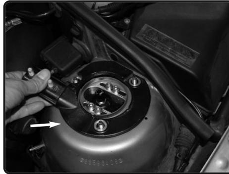
**26.** Re-install the strut tower plate.
