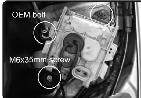
**22.** Install the ballast and position. Secure using OEM bolt on top and nut, for bottom near headlight, use provided M6x35mm socket cap screw. Secure and tighten using Allen key.
