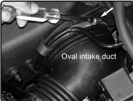
**4.** Loosen the clamp on the oval air intake duct located on the throttle body.
