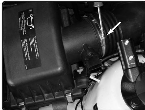
**5.** Loosen the clamp located on the lower air intake duct connected to the mass air flow sensor.
