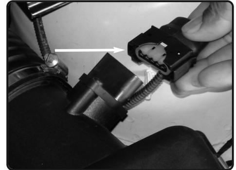
**3.** Press the side tabs on the electrical sensor harness and pull the harness away from the mass air flow sensor.
