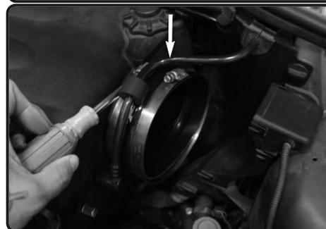
**10.** Install the provided hump hose with clamps provided to the intake plenum.
