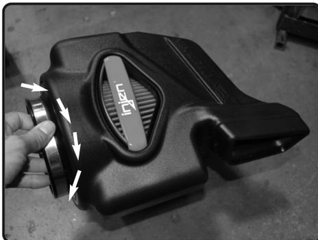
**16.** Once the twist lock filter is seated, rotate in either direction a 1/4" turn. Filter will lock into place.
