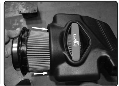
**15.** Install the twist lock filter to the air box.
