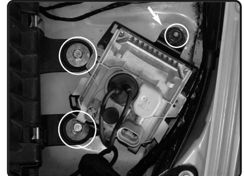
**7.** Loosen and remove the two m10 bolts and the m10 flange nut. Lift up and remove the Zenon ballast out of the way, this will allow you to remove the air box cleaner. Set Ballast to the side. Save 1 bolt and nut for later install.
