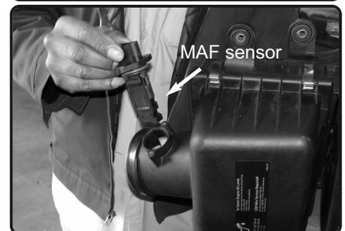
**11.** Loosen and remove the two screws on the mass air flow sensor. Pull the mass air flow sensor out of the sensor housing as shown above.
