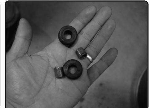
**19.** Remove the OEM grommets and crush washers from the stock air box. This will be used on the new Injen air box.
