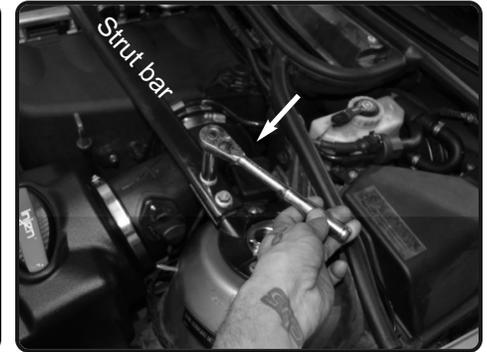
**27.** Re-install the strut bar and secure and tighten the complete strut bar assembly.
