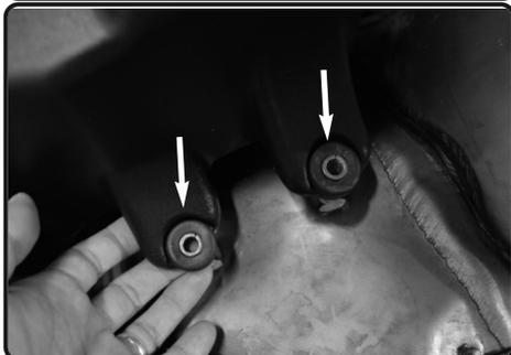
**20.** Install the grommets with crush washers to the new Injen air box.
