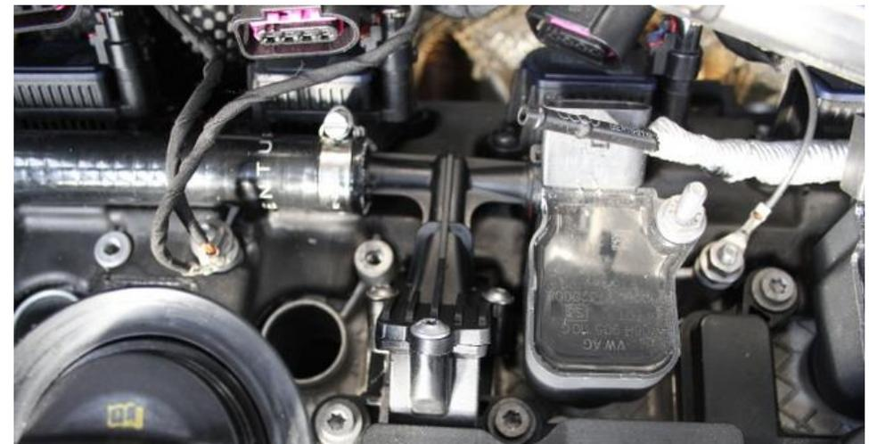
24. Once lined up – secure the plastic breather adapter into place with the 3 torx screws. Also tighten the hose clamp around the silicon tube at this adapter end only. Do not over tighten.
