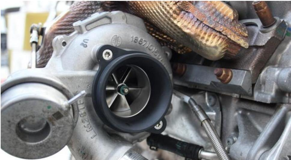
10. Secure the flange to the turbo using the supplied screws – we recommend to also use a thread lock such as Loctite 246. (Photo shown with engine out for clarity).
