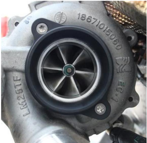
12b. **CORRECT** – the flange is concentric with the turbo inlet.
