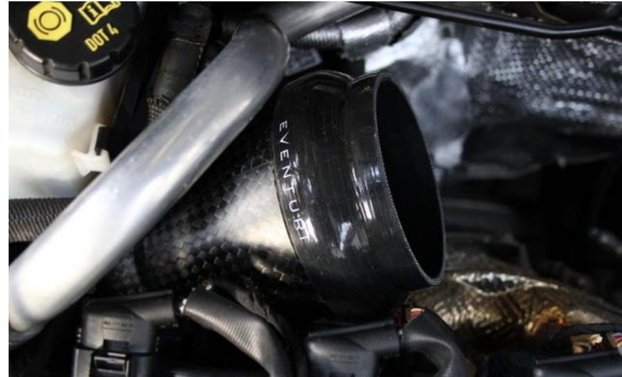
34. For the 3.5" intake, attach the reducer silicon as shown.
