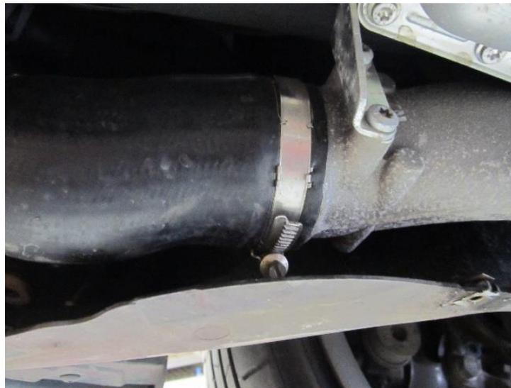
4. Loosen the hose clamp around the rubber boost hose which is connected to the metal tube.
