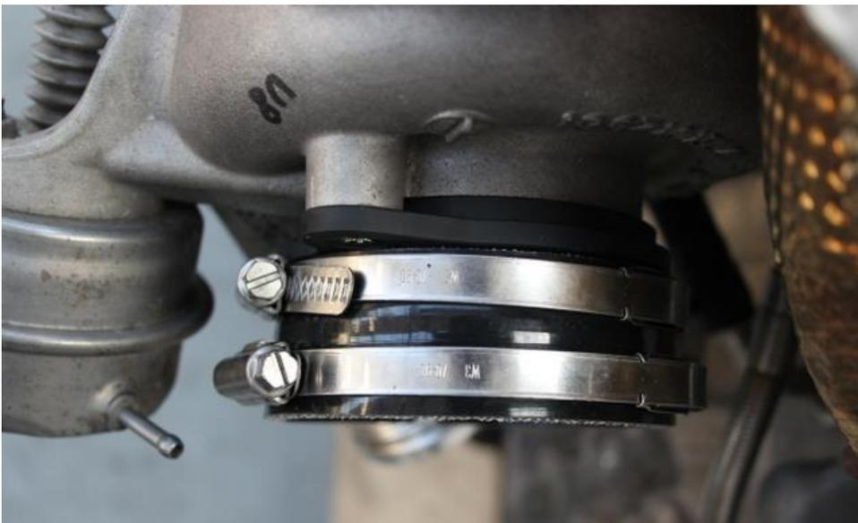
15. Take the 2 x 70-90 clamps and position them as shown. Tighten the one around the flange. Leave the other one very loose. Position the heads so that they are reachable from the top.
