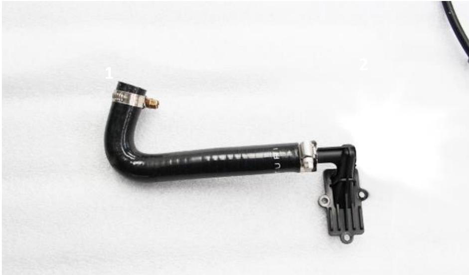
21. Take the Hook shaped silicon tube and attach it to the breather adapter as shown. Use the 2 small hose clamps as shown but don't tighten yet.
