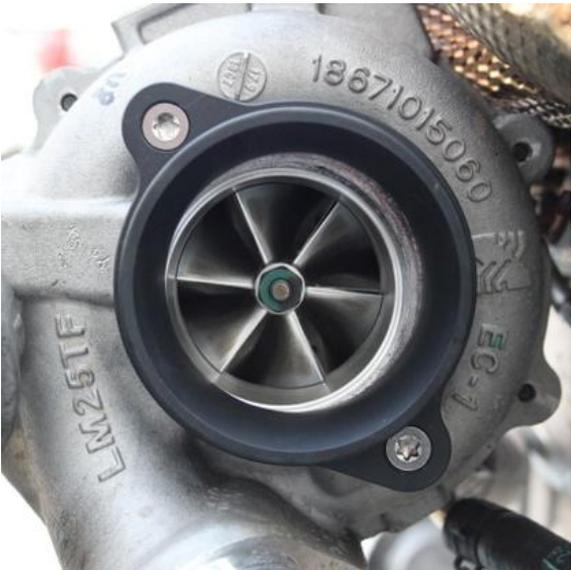
12a. **INCORRECT** – the flange is not concentric with the turbo inlet. Rotate the flange 180 degrees.
