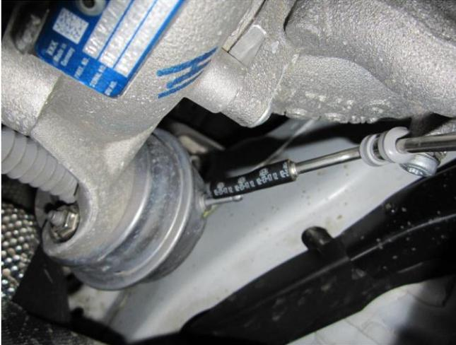
5. Remove the vacuum tube from the actuator.
