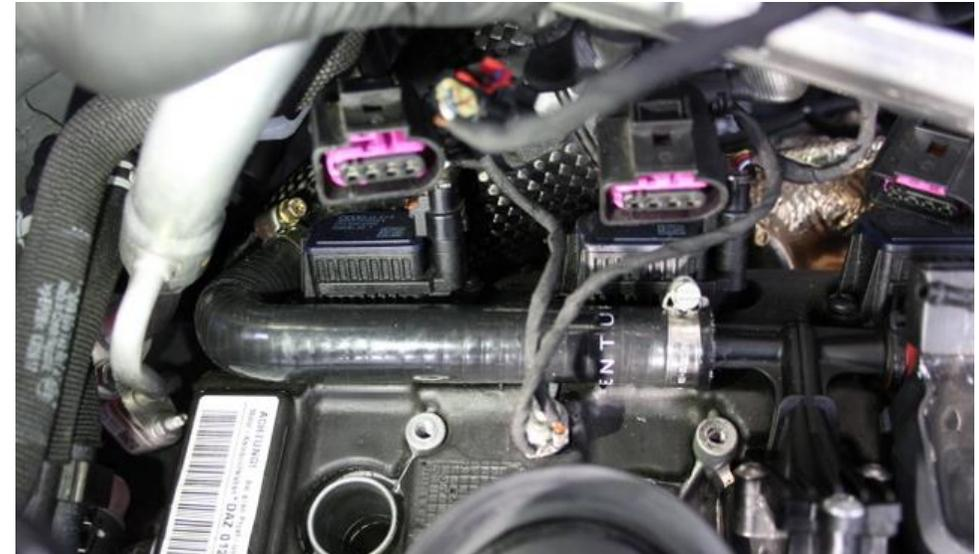
22. Place the adapter and hose into position, push the silicon onto the carbon tube breather inlet. Rotate the carbon tube towards the engine to get the breather assembly into position. The breather adapter should line up with the fixing position on the engine. You may need to trim the silicon tube if it does not.
