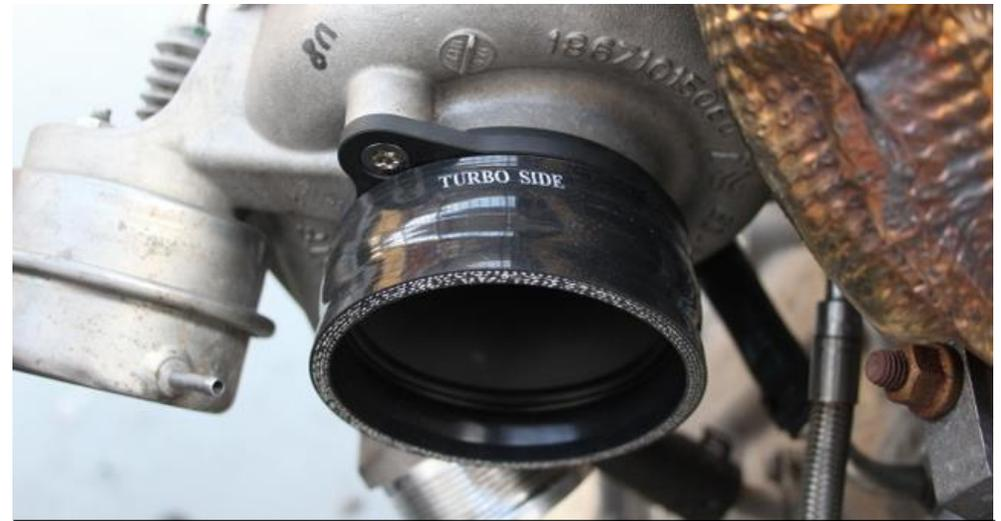
14. Push the silicon onto the flange so that the “TURBO SIDE” writing is closest to the turbo. The silicon will be tight to push on but will snap into place as the bead around the flange locks into the groove inside the silicon.
