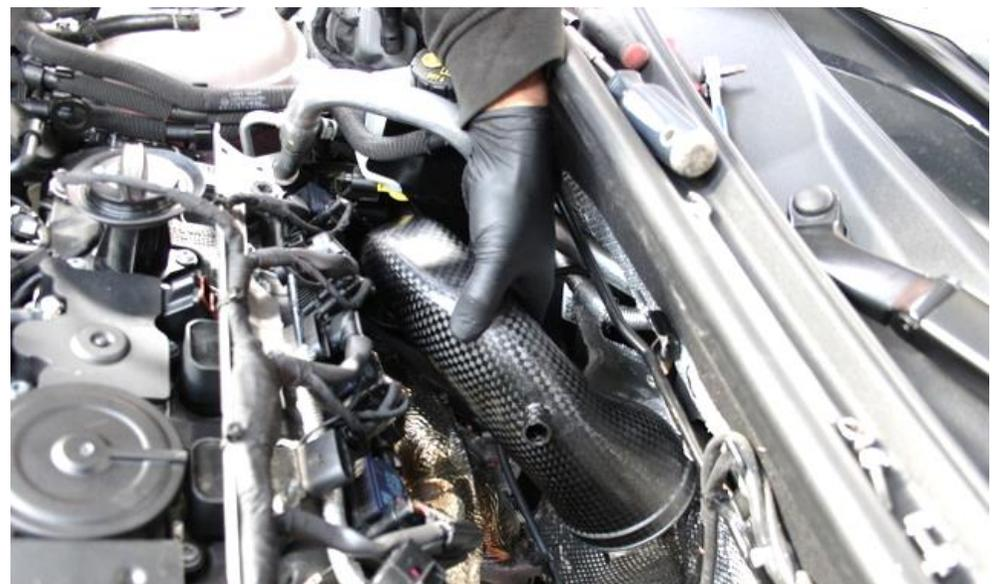
16. Insert the inlet tube from the top by rotating it in as shown.
