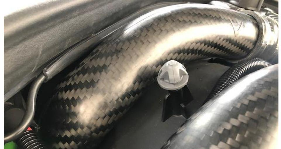
18. It can be easier to install the engine cover by putting the rubber mount onto the holder first.
