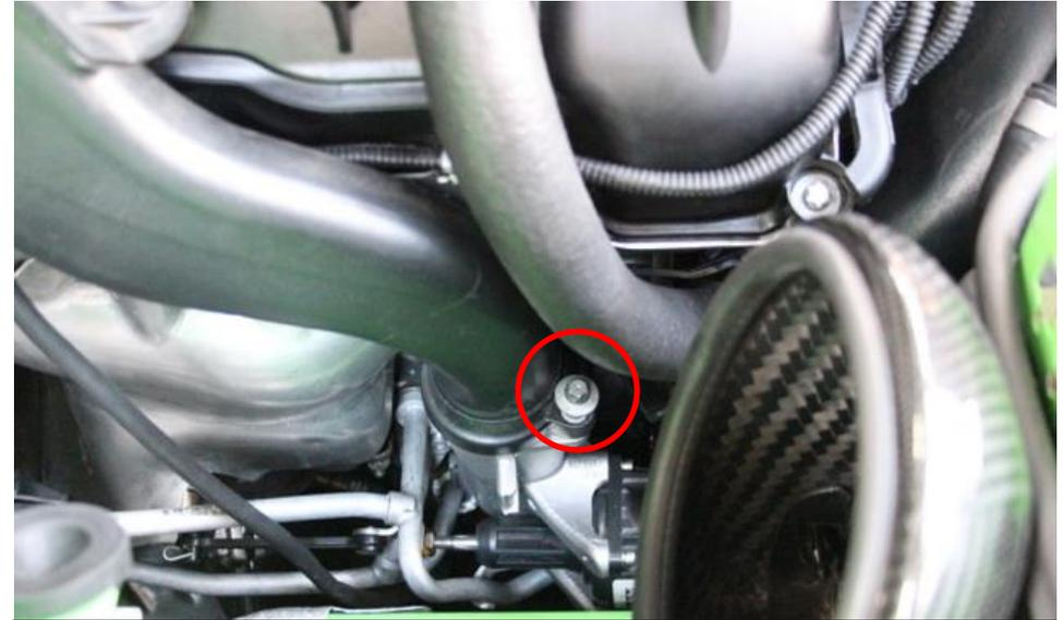
2. Remove the screw holding the front chargepipe on the turbo outlet pipe.
