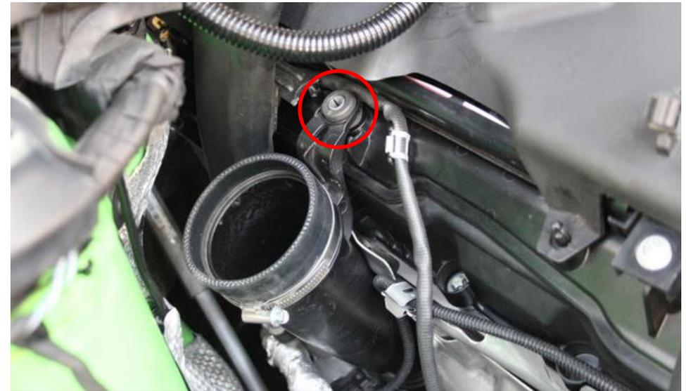
4. Remove the plastic turbo inlet pipe by removing the retaining screws and then pulling out the pipe.
