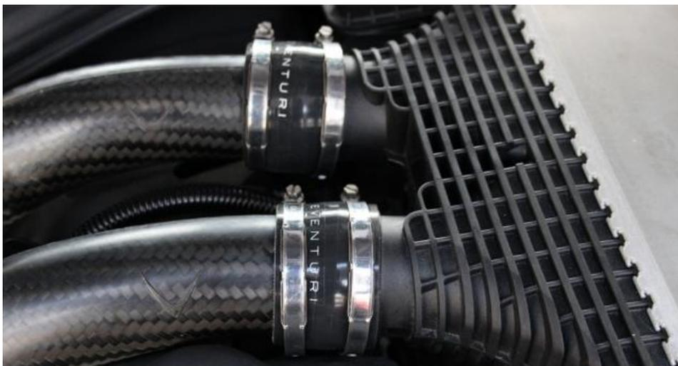
15. Install both chargepipes and tighten all clamps.
