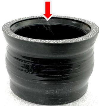
9. Use the smaller silicons for the flanges. One side of the silicon has a tapered edge as shown. This side must face down onto the flange and the non-tapered edge should face upwards for the carbon pipe.
