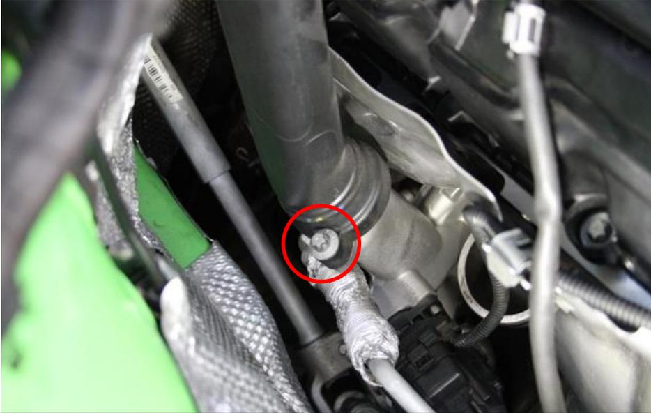
5. Now remove the screw holding the rear chargepipe in place and remove the chargepipe completely.
