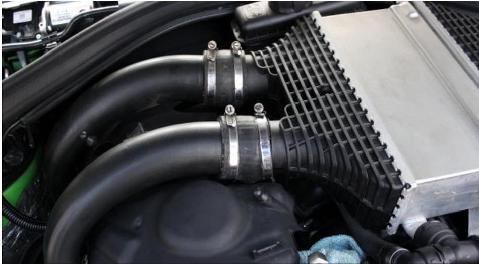
1. Remove the intake system on the left side for easier access to the chargepipes. Start by loosening the hose clamps on the top side of the chargepipes.
