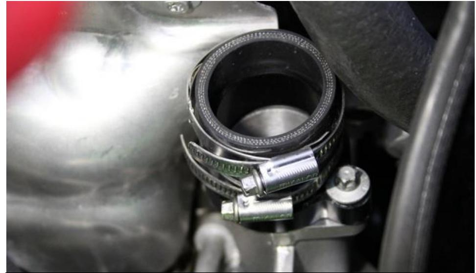
10. Push the tapered side down onto the flanges all the way down. Install the smaller hose clamps (40-60mm) onto the silicons. Make sure the clamps do not interfere with the screw - face them away as shown. Tighten the clamps around the flange.
