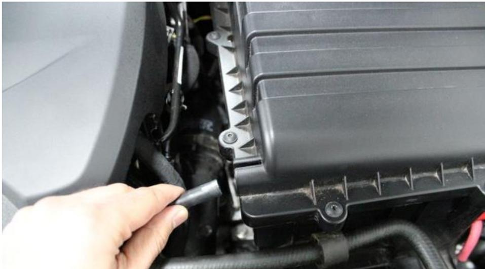
3. Remove the vacuum tube from the airbox – it will pull out.
