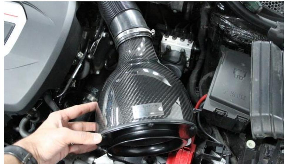
16. Push the intake into the stock plastic inlet tube – use the provided hose clamp instead of the stock spring clamp around the tube. Do not tighten yet.
