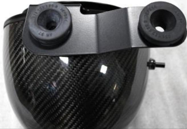
5. Install the rubber mounts into the new bracket as shown.
