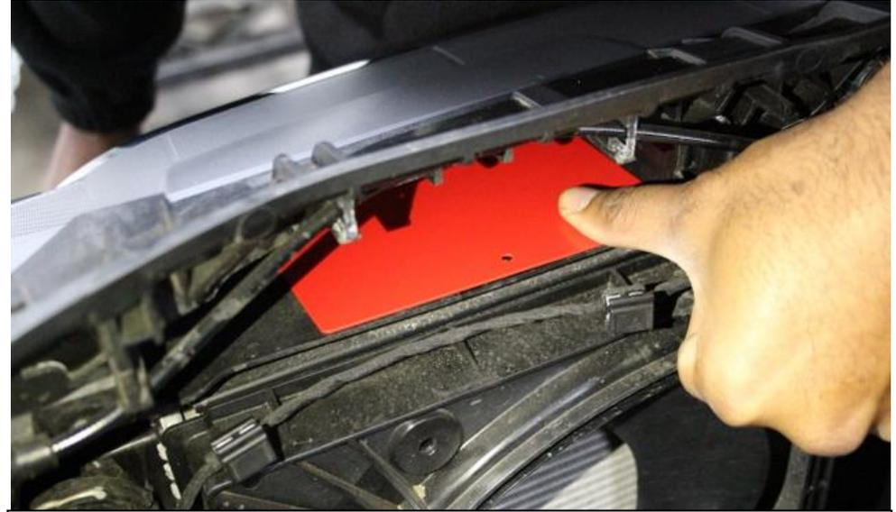
10. Put the scoop into position as shown and secure with the 2 panel clips as shown in next step.
