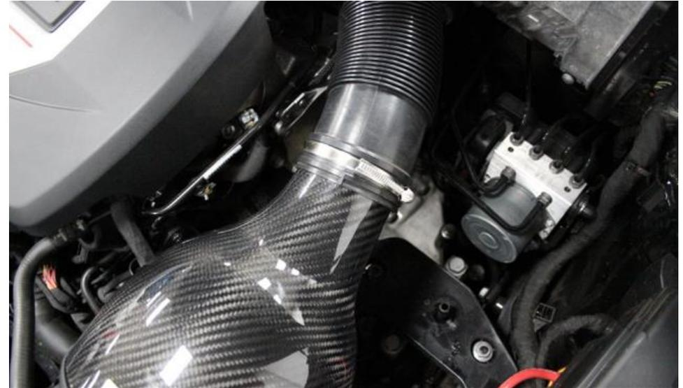
18. Now tighten the hose clamp around the tube.
