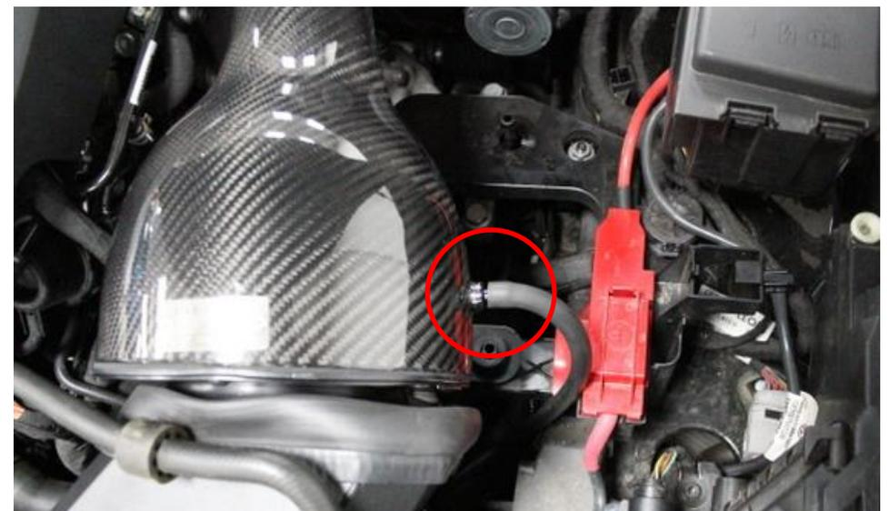
20. Route the extension tube around the bottom of the intake and push into the connector on the side.
