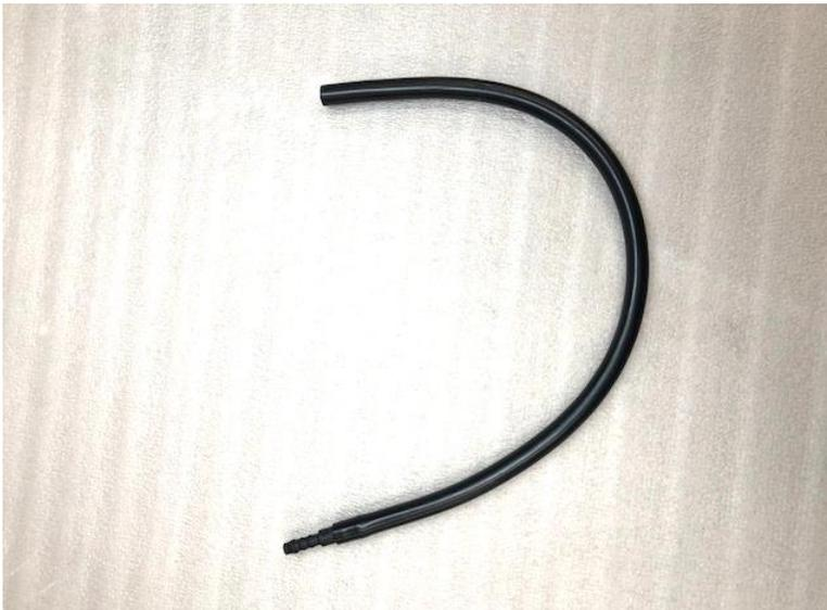
19. Take the vacuum tube extension and push the plastic connector side into the stock vacuum tube removed in step 3
