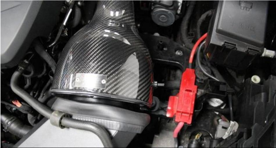
21. Ensure the rubber edging is on the outside of the intake all the way around – it does not need to seal with the intake since the scoop forces air to the filter. A small gap also de-restricts the intake path.
