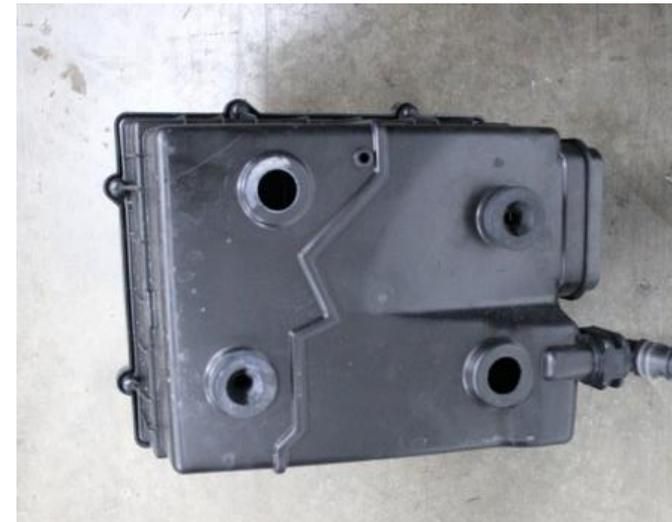
4. Remove 2 rubber mounts from the base of the airbox. We will use them in the new bracket.
