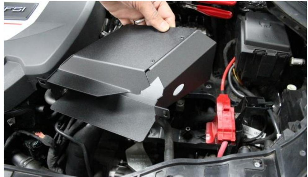
12. Take the new duct – it will be positioned in the orientation shown. Lower the duct into place.
