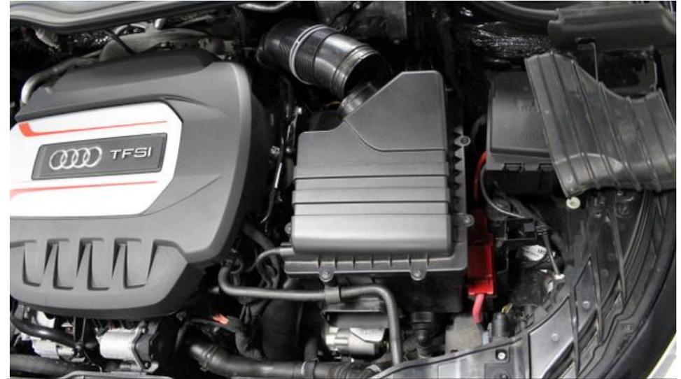
2. Loosen the clamp around the intake tube at the back of the airbox and remove the tube from the airbox. (Use appropriate spring clamp tool). Also remove the rubber duct attached to the front of the airbox. It will simply pull out.
