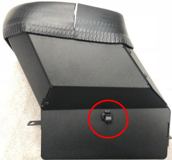
13. On the base of the duct there is a clip – push the wire from step 7 into this clip.
