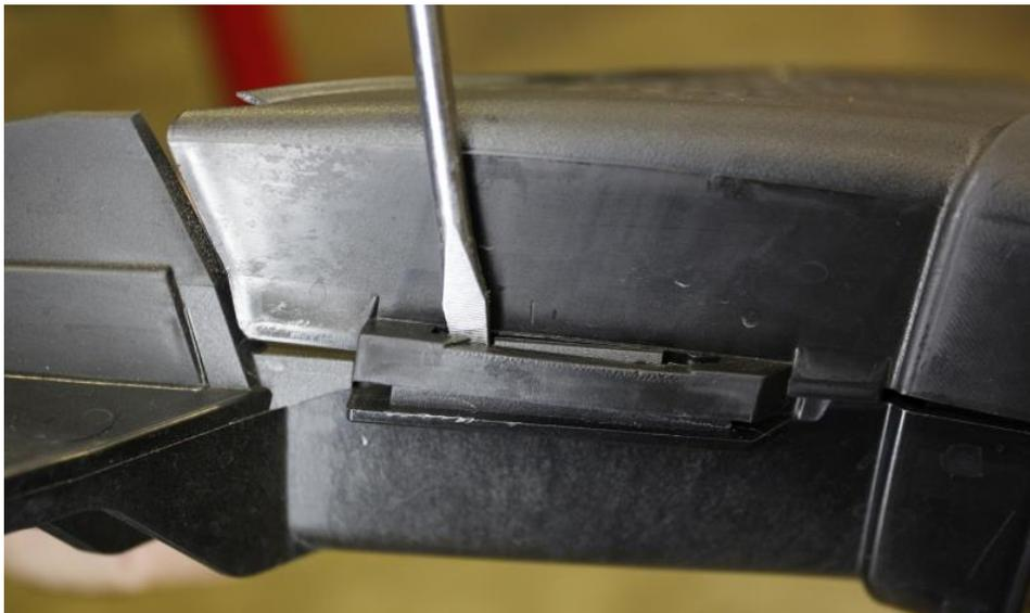
15. Now do the same on the other side – pull the cover upwards as you prise open the tab. The sides of the top cover should now be free.
