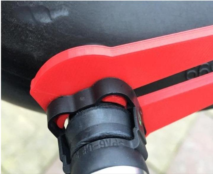
5. Make sure all 4 extrusions are FULLY inside the locking ring.
