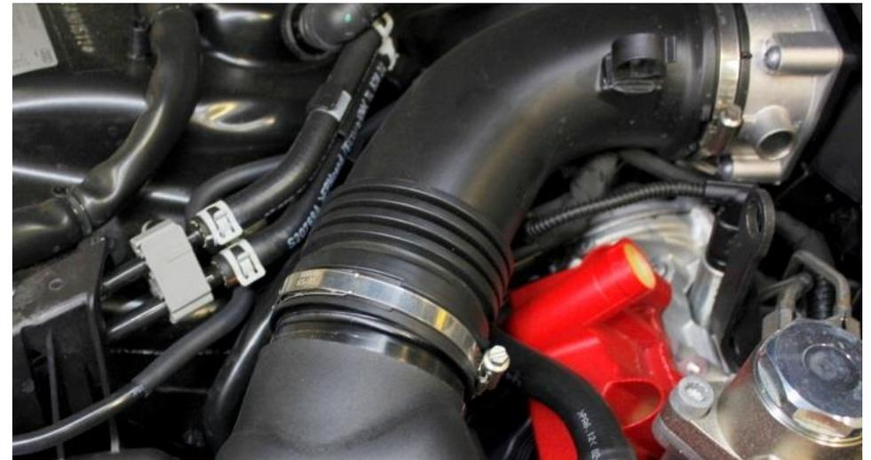
8. Loosen the hose clamp between the inlet hose and the airbox. Push the inlet hose off the airbox.
