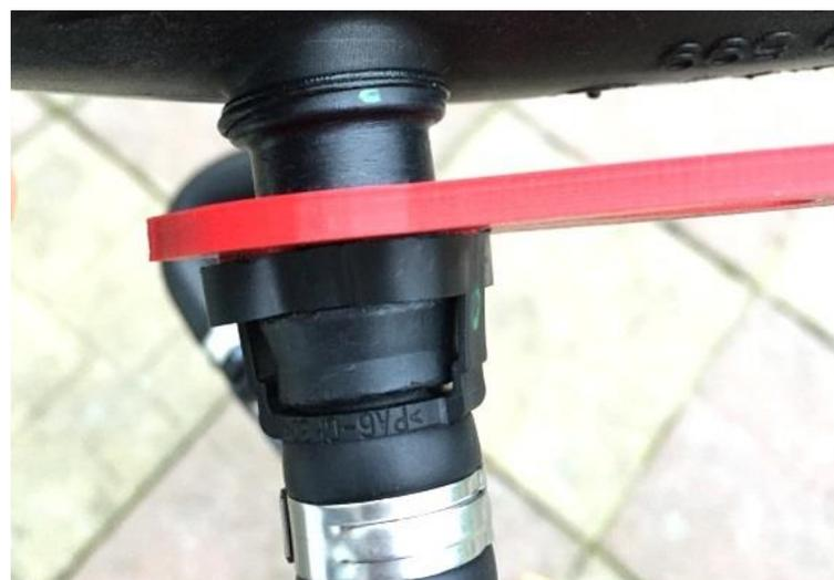
4. Push the tool down so that the 4 extrusions go into the 4 openings of the locking ring fully.
