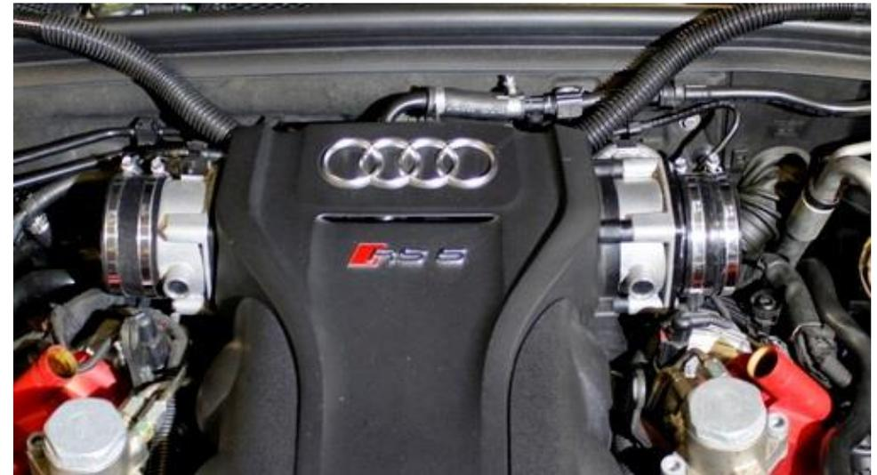
33. Take 2 of the silicon couplers and install onto the throttle bodies. Push them on fully and tighten the clamp over the throttle body. Leave the other clamp loose.
