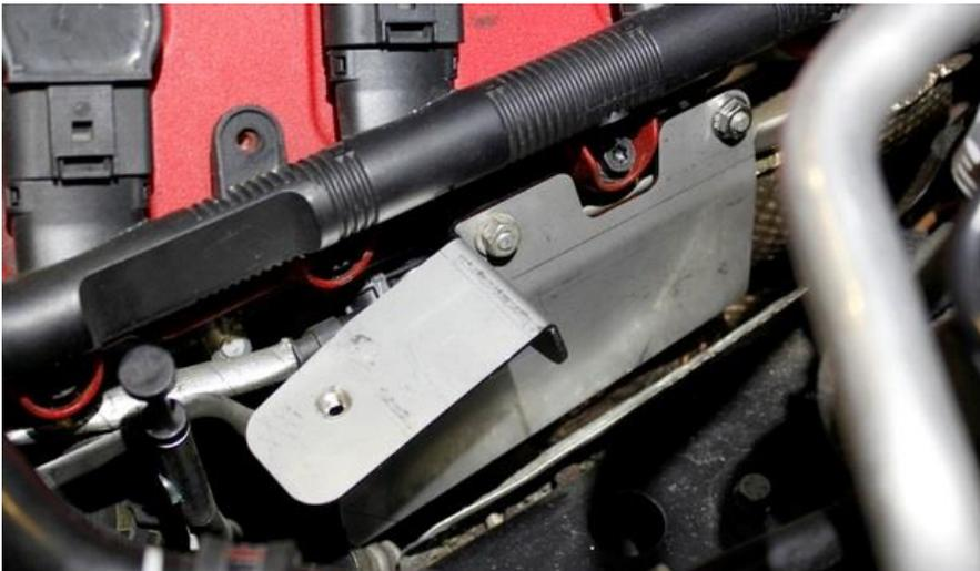
32. Take the RHS heat shield and install into the right side where the airbox mount was located. Secure again with the 2 provided 10mm nuts. Heat shield shown in silver for illustration purposes.
