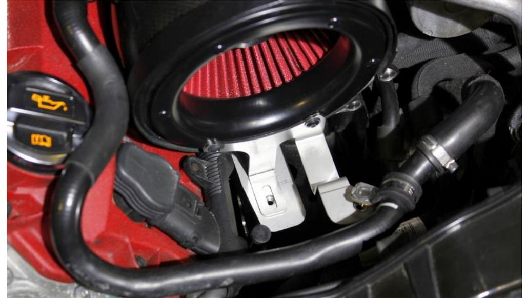
59. The bracket on the air hose should go on top of the housing bracket as shown.
