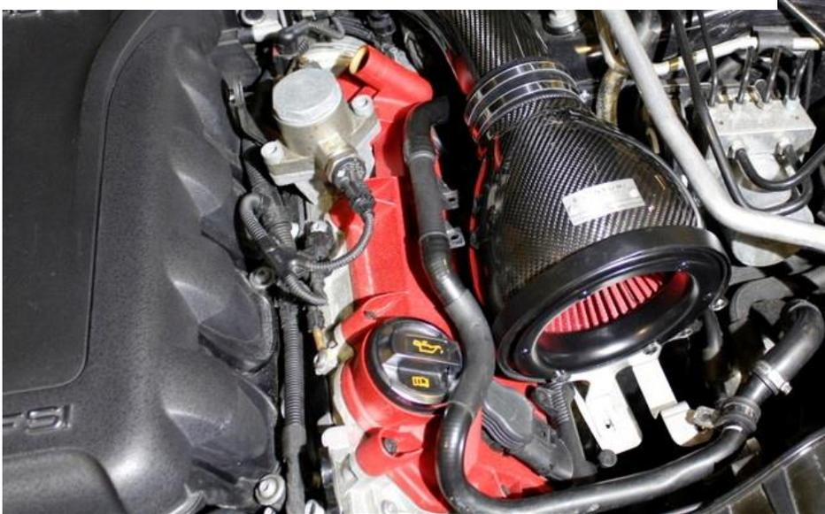
58. Push the RHS housing into place and lower the intake down to rest the bracket onto the heat shield. Lift the secondary air hose over the oil filler cap for more clearance.
