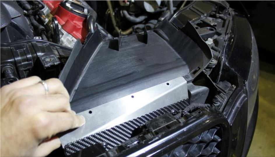
23. Place the edge of the plate onto the edge of the duct (highlighted previously) and hold the plate flat onto the duct. Now line up the scoop so that it touches the inside of the grill and isn't obstructed by anything else. Please note – the scoops shown here are an older version. Your scoops are updated but still follow the same procedure.
