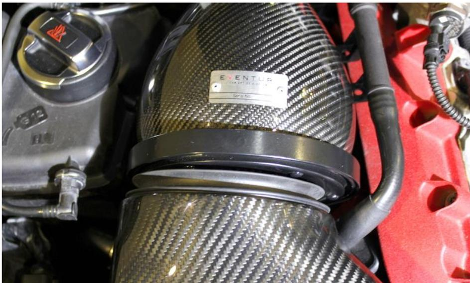
49. Check the alignment between the rubber seal on the duct and the housing. Here you can see the housing needs adjustment.
