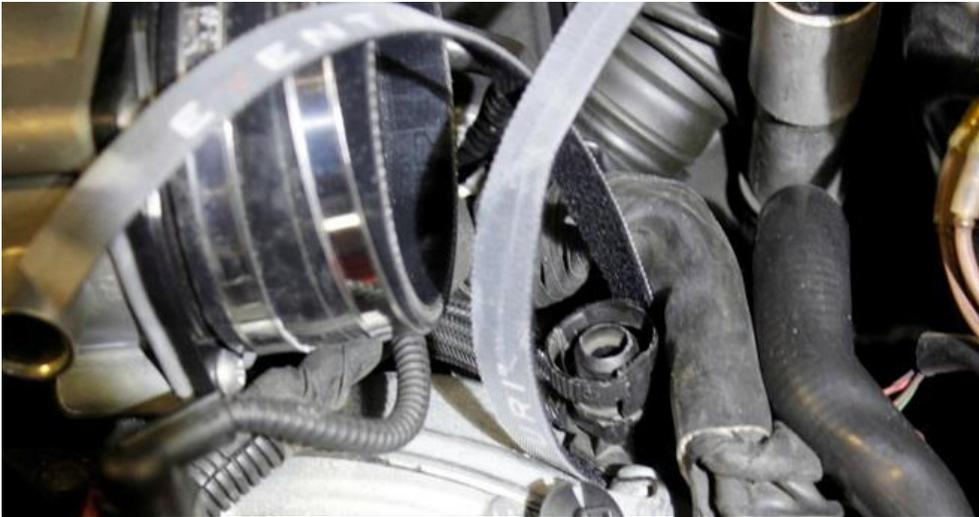
55. A tricky process on this side is getting the breather hose back into place on the tube as it doesn't have much slack. An effective way of doing this is to take one of the longer Velcro straps from the packaging and run it underneath the hose connection.
