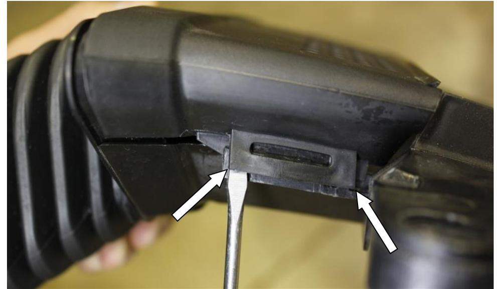
14. Using a flat head screwdriver, carefully prise open the tab on one side of the cover from the 2 edges. These tabs are easily broken so take your time doing this.
