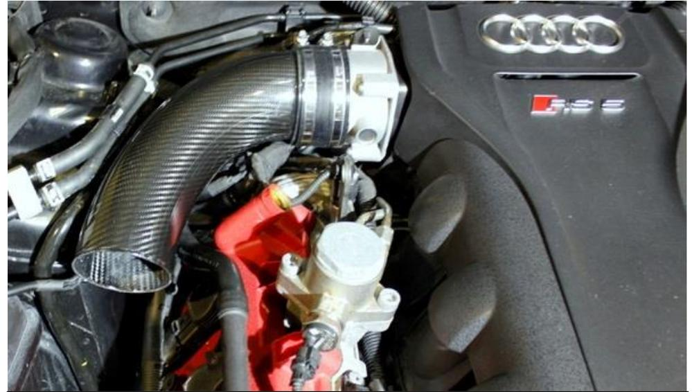
44. Push the tube into the silicon coupler – do not tighten the hose clamp yet.
