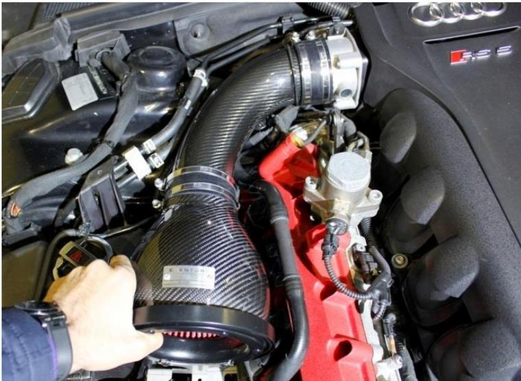
45. Take the LHS Housing and push the silicon on the back of the housing into the carbon tube. Lower the tube and housing onto the heat shield.
