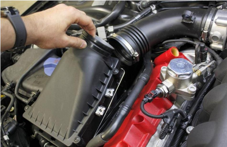
9. Pull the back of the airbox upwards to release it from its mount – then remove the airbox completely from the engine bay.
