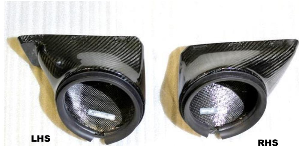
37. Identify the LHS and RHS Carbon Ducts as shown.
