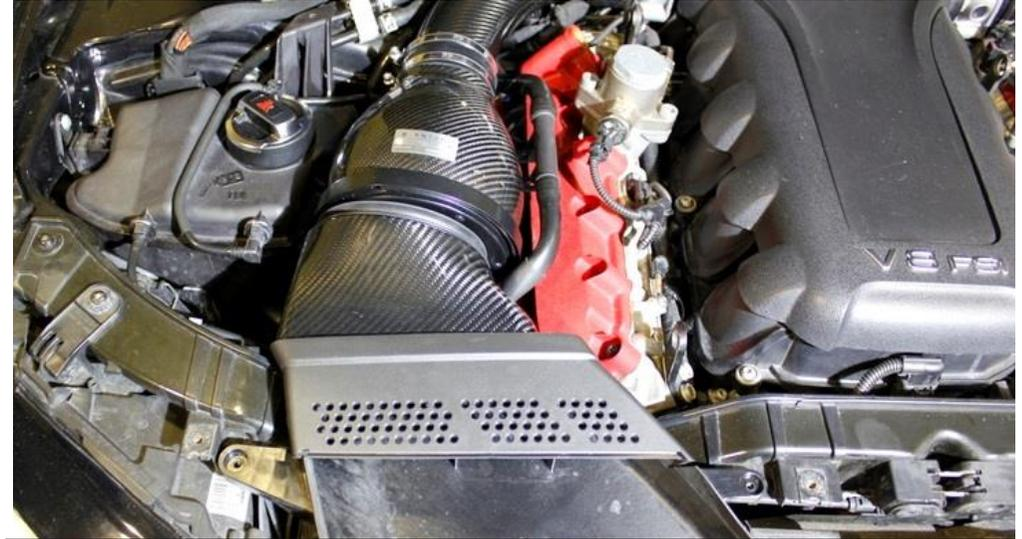
48. Take the LHS duct assembly and put it into place – the scoop goes in first then lower the duct and move it forward towards the housing. Line up the securing holes on the sides of the stock duct – do not secure yet.
