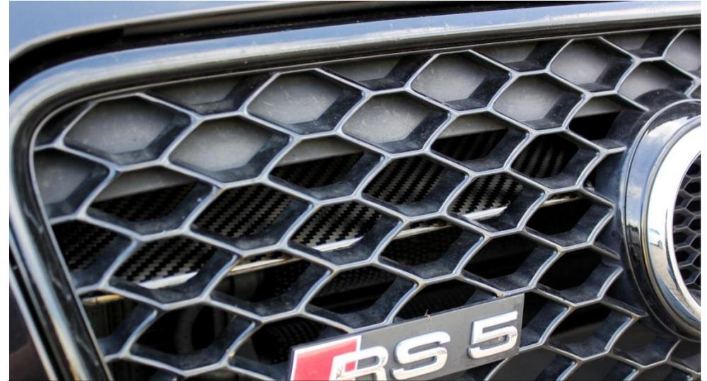
24. Scoop should sit just behind or touch the grill unobstructed. LHS scoop shown for illustration. Once lined up – mark the 3 holes onto the stock duct through the holes on the metal plate.
