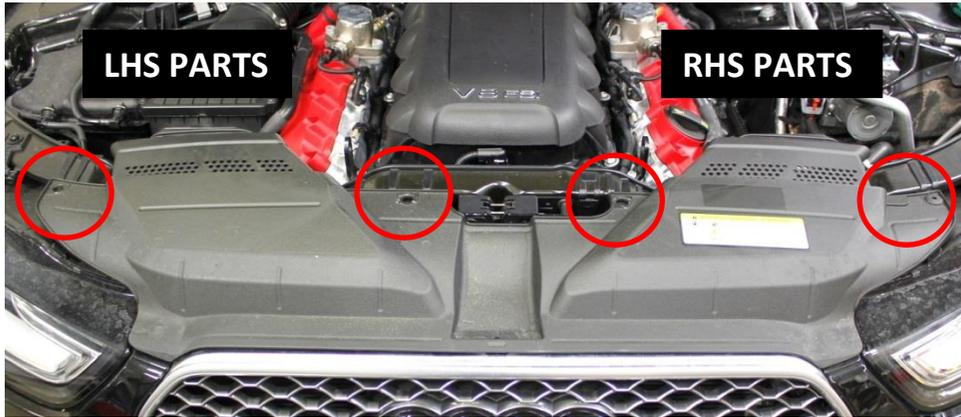
1. Remove the 4 Plastic Rivets as circled (or torx screws for earlier models) securing the duct cover in place. We will refer to the left hand side and right hand side parts as indicated above.
