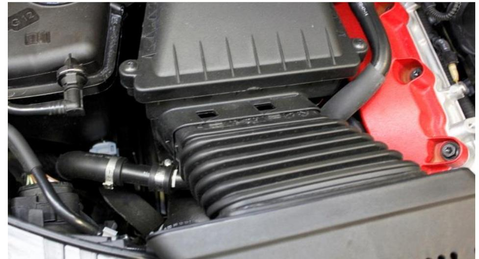
4. Pull the corrugated duct feeds out of the airboxes. Push the fronts down to release the tabs holding them into the airboxes on both sides. Once removed from the airboxes, remove the ducts completely.
