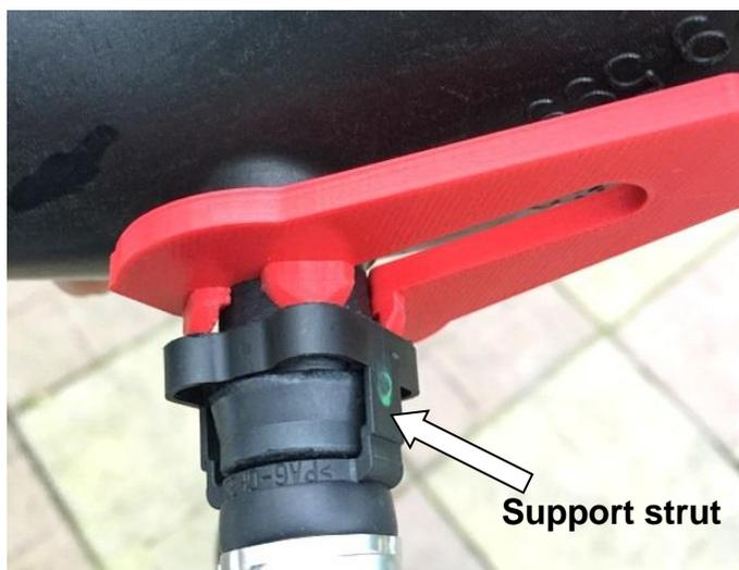
3. Push the tool onto the breather inlet – it will snap into place. Make sure it is positioned with the support strut of the breather facing the back/front of the tool as shown.
