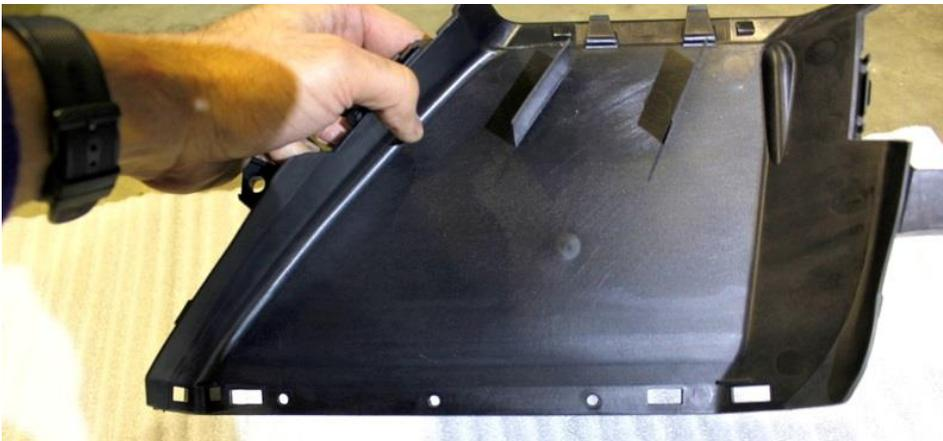
25. Remove the duct and use a 5mm drill bit to make the 3 holes. Once done, secure the scoop to the duct with another 3 black flanged bolts and lock nuts.
