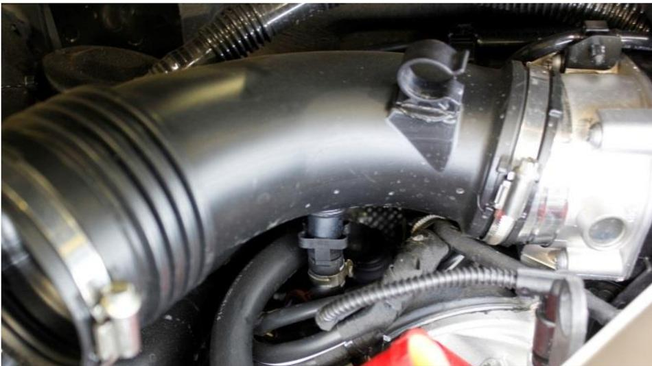
11. Loosen hose clamp around the inlet tube and throttle body. Pull the tube out of the throttle body to give you more room to access the breather hose underneath.
