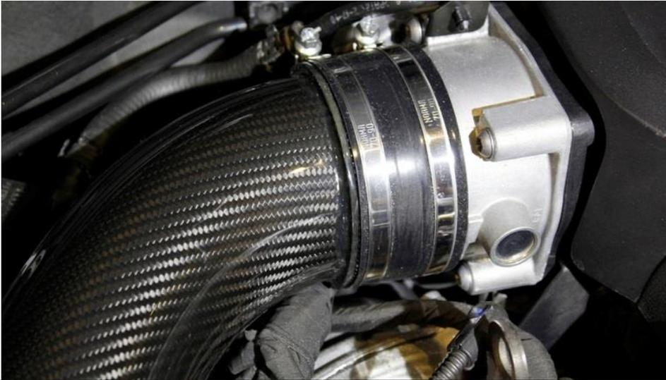
47. We will now adjust the positioning of the housing to be straight with the duct. Firstly, ensure that the carbon tube is fully inside and the carbon flange is square with the silicon on the throttle body. Now tighten the clamp to fix the carbon tube in place. Do not overtighten.
