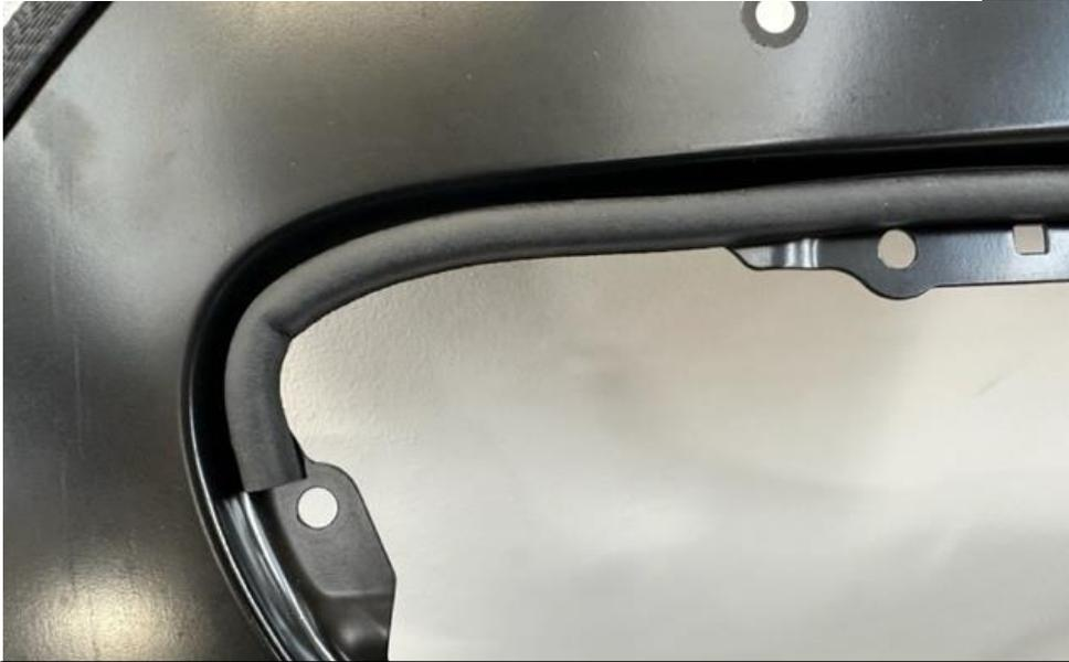
29. Close up of one side of the location for the strip. Make sure to avoid covering the holes.
