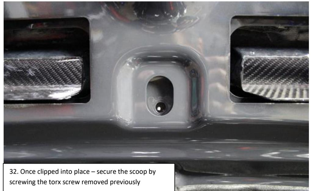
32. Once clipped into place – secure the scoop by screwing the torx screw removed previously
