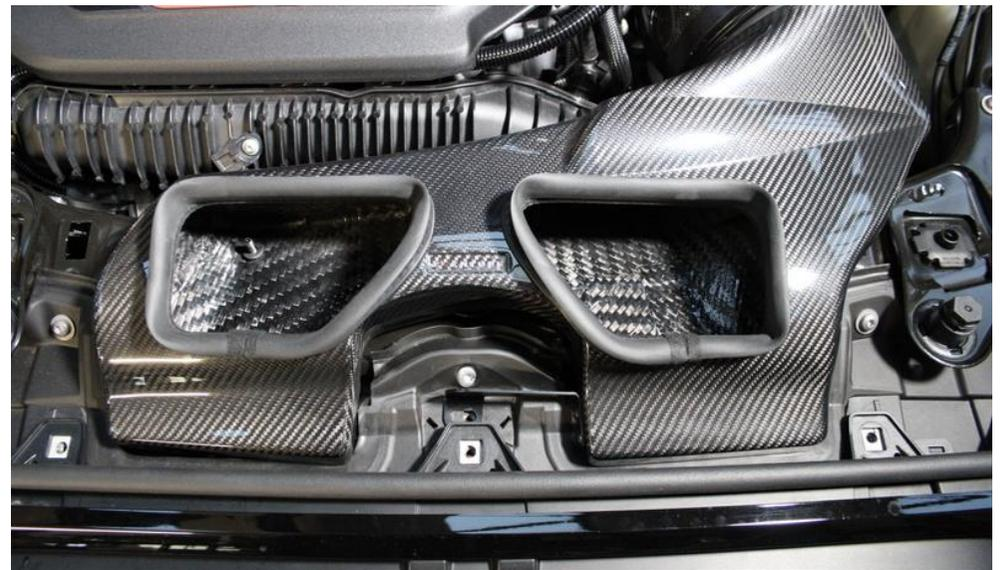
12. Push the duct into place and ensure the studs in step 8 go through the rubber grommets in step 9.
