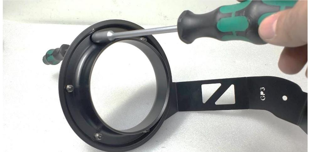
4. Once the housing bracket assembly has been removed unscrew the housing bracket from the cowl with an 8mm socket and 3mm Hex screwdriver.
