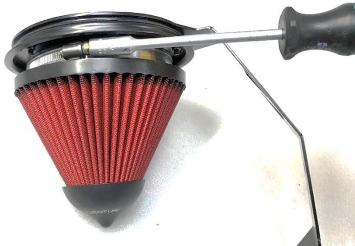
13. Secure the filter to the housing bracket assembly with a 7mm socket
