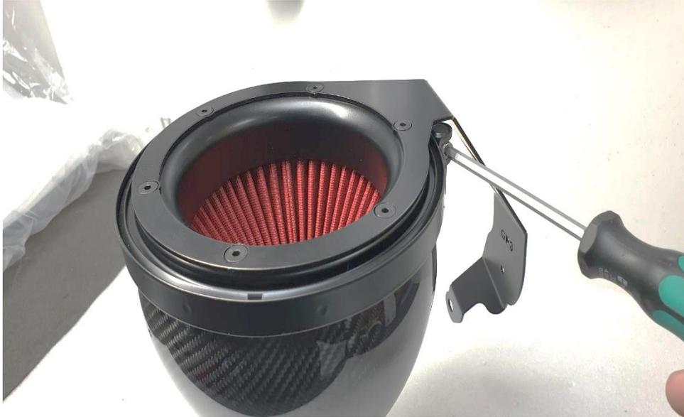
2. Unscrew and remove the V-band which is holding the filter to housing with a 4mm Hex screwdriver
