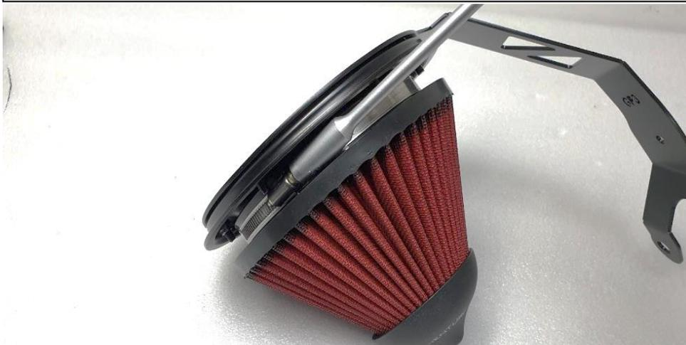
3. Once the filter assembly has been removed unscrew the screw clamp from the filter with a 7mm socket and remove the housing bracket assembly from the filter.
