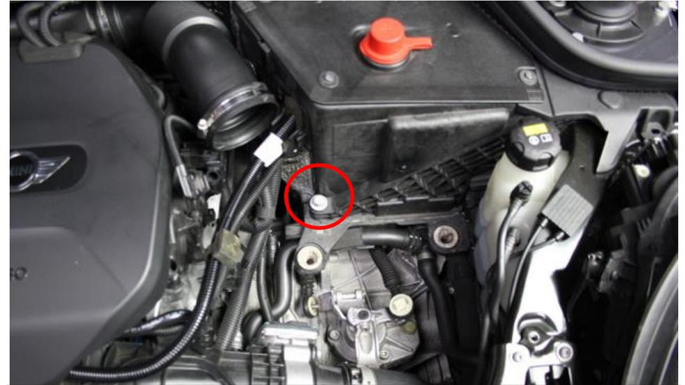
6. The airbox can now be lifted out of the engine bay. Also remove the bolt at the base of the battery tray as circled. This will be required to secure the intake later.
