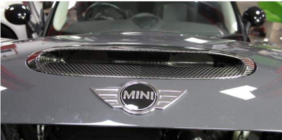
31. Once the clips are in position firmly push the scoop down in all 6 clip positions and ensure they click into place. The clips are firm so please make sure by checking from the underside that they are fully engaged.
