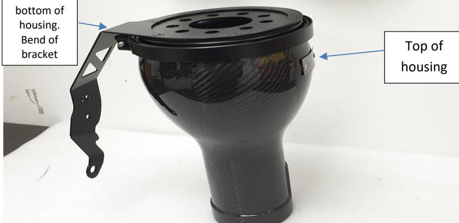
15. Insert the filter assembly into the housing make sure that the bend of the housing bracket is at the bottom of the housing. (The side where the Eventuri plaque is located is the Top of the housing, so it should be opposite this)
