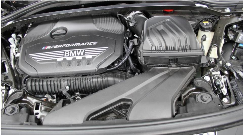
1. We will start by removing the stock airbox and duct. BMW 135i engine shown which is the same.
