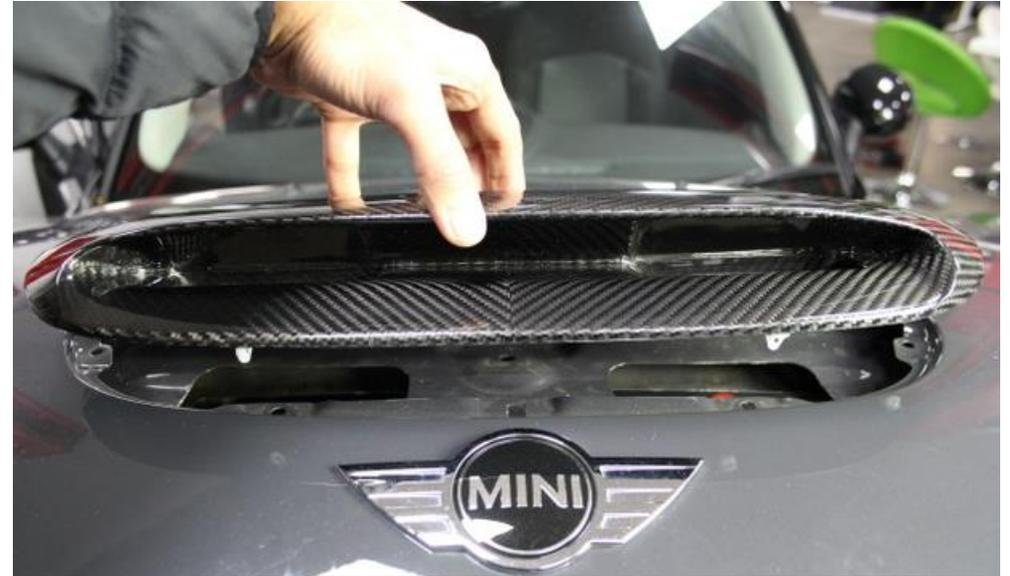
30. Carefully lower the carbon scoop into position – make sure the 6 clips are already installed on the back of the scoop.
