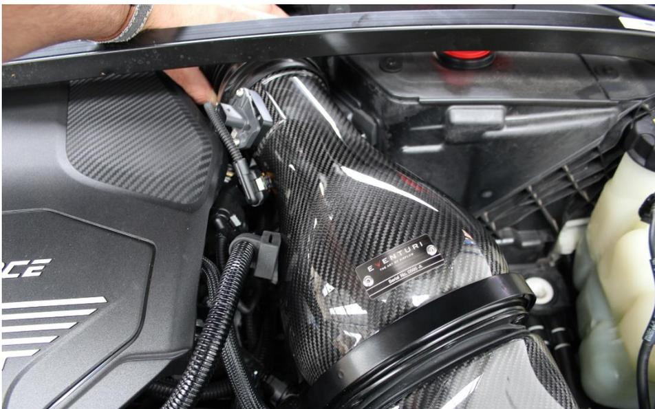
19. Line up the filter housing with the duct and then secure the bracket with the Bolt removed previously. See next step.
