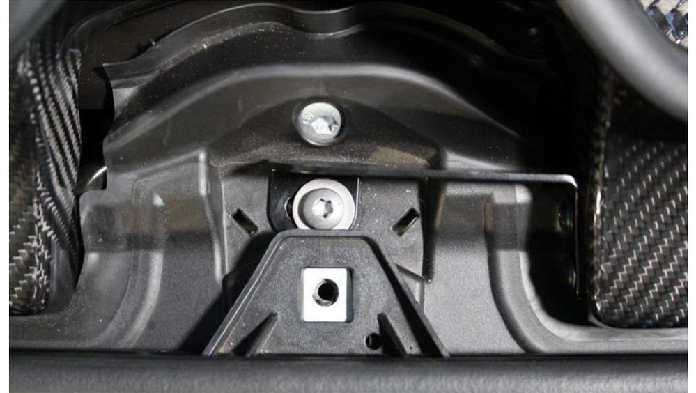
14. Secure the middle bracket with the Torx screw removed previously.
