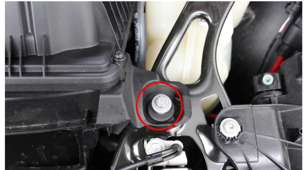
4. Remove the M6 Bolt on the right side of the airbox which holds it in place.
