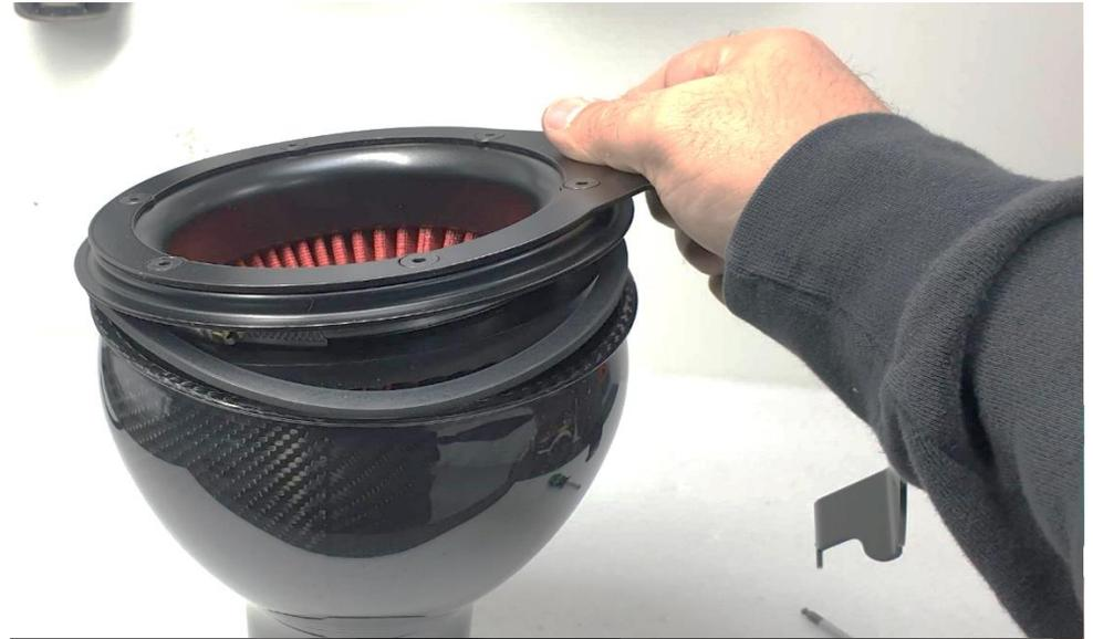
2. Remove the Filter assembly and the gasket from the housing.
