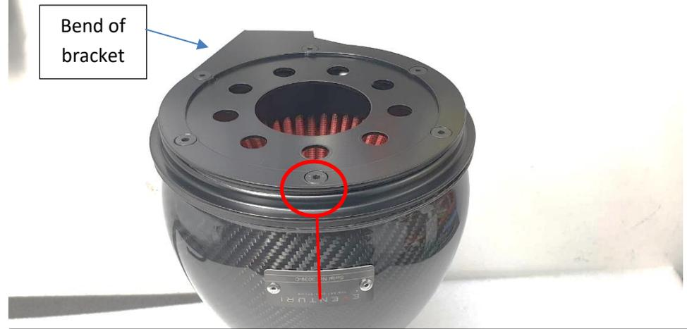
16. Once the filter assembly has been inserted into the housing make sure that the screw circled in RED is in line with "N" in Eventuri. Notice the bend of the bracket is at the opposite side of the plaque
