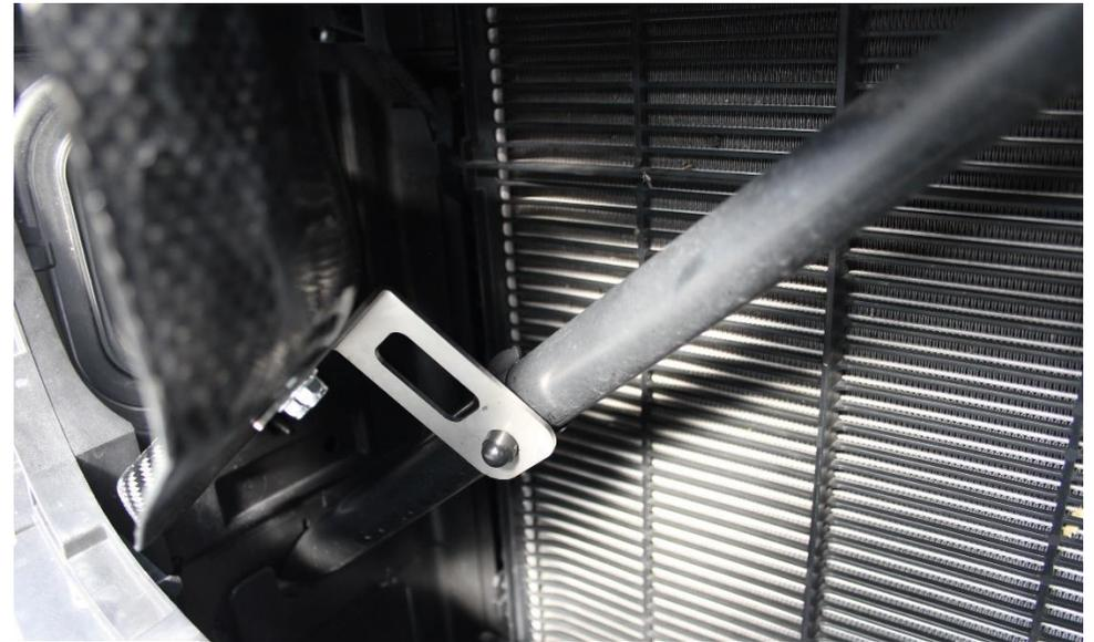
18. Push the clip onto the strut brace.
