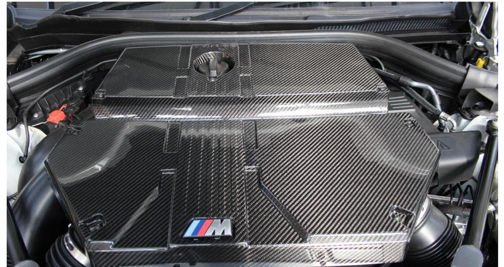
12. Use the supplied plastic washers with the OEM screws and install the lid. Re-install the Strut Brace.
