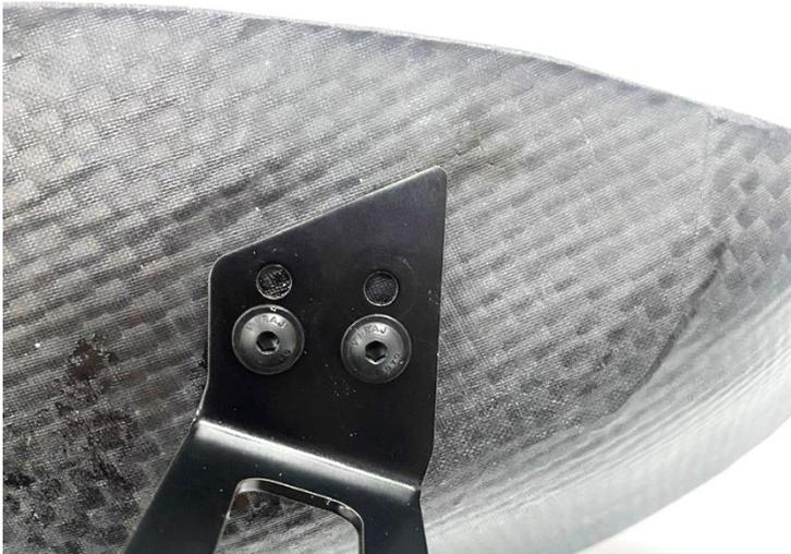
4. LCI – Secure the bracket to the scoop using the lower holes as shown.
