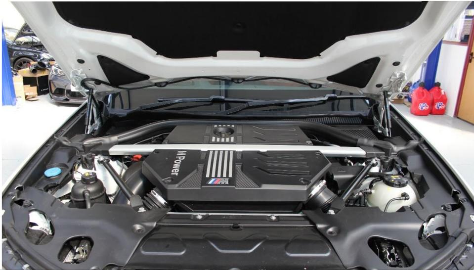
1. Start by removing the strut brace.
