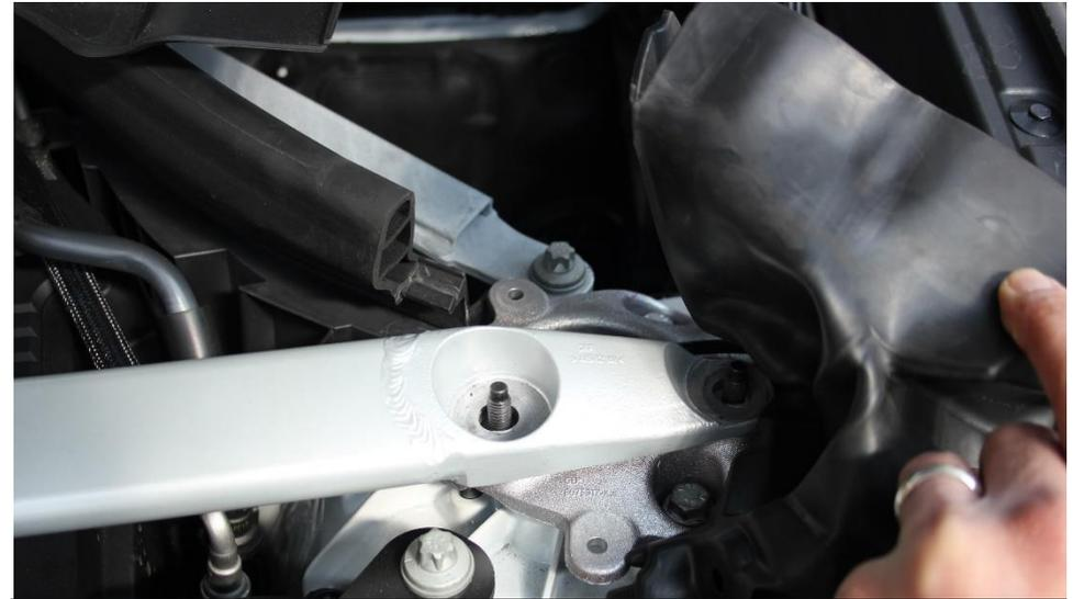
2. Underneath the rubber end covers on each side of the brace there are 2 nuts to remove.
