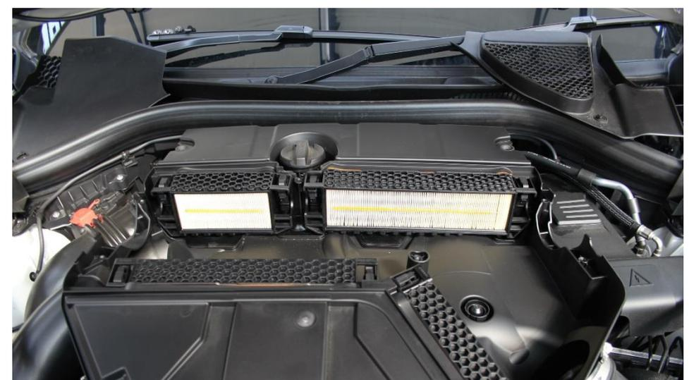
4. Loosen the screws on top of the airbox lid and lift the lid off to expose the filters.
