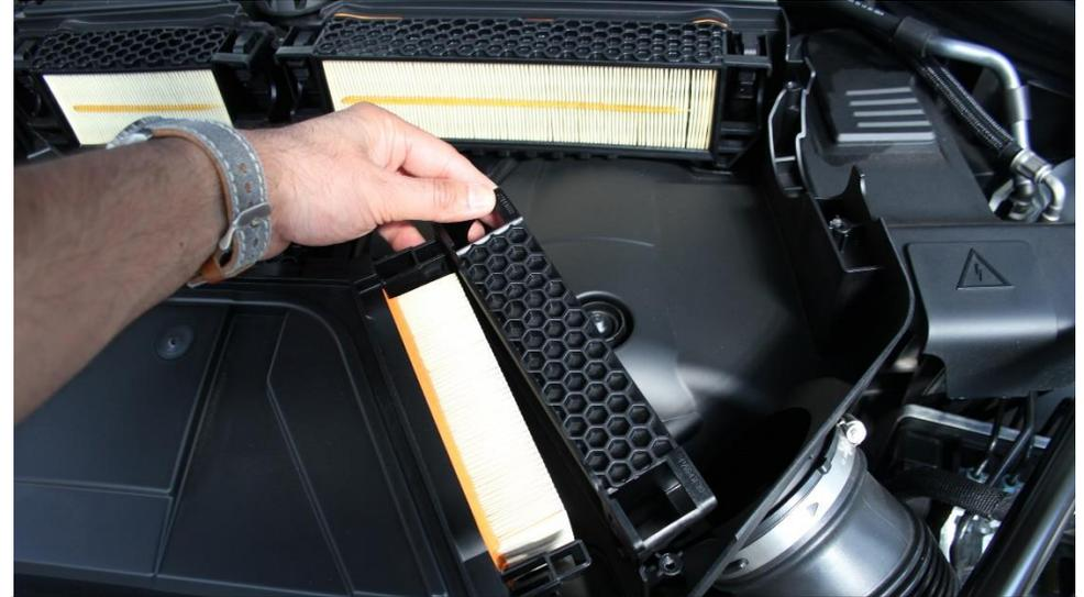
6. With the clips removed, the frames can be removed as well. Take out all the filters. If you also have grey charcoal filters behind the paper filters, you may also remove these.
