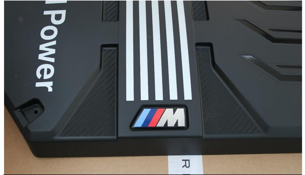
10. Remove the M Badge from the cover – it is held in place with tabs on the reverse – these can be carefully bent back and the badge can be removed.
