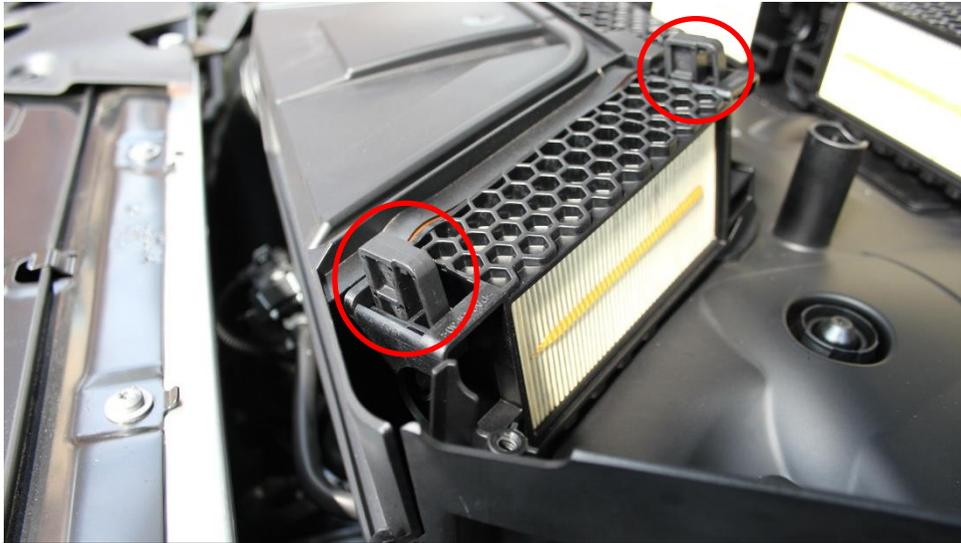
5. The filters are held in place with plastic frames which are secured with clips on each side. Lift up the clips by pressing them in the middle.
