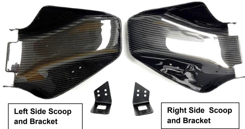
1. Arrange the Left and Right scoops as shown with the brackets which are also shown here as Left and Right.
