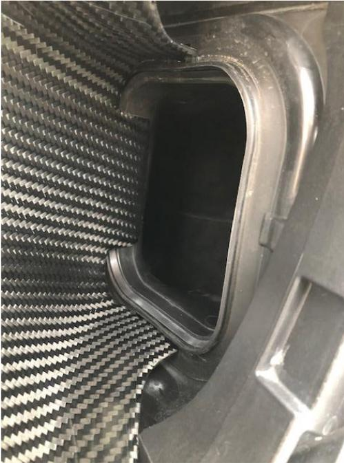
21. The end result should look like this. The inside duct panel should be secure with the scoop clips and the scoop should sit flush against the duct entry. Re install the front grills.
