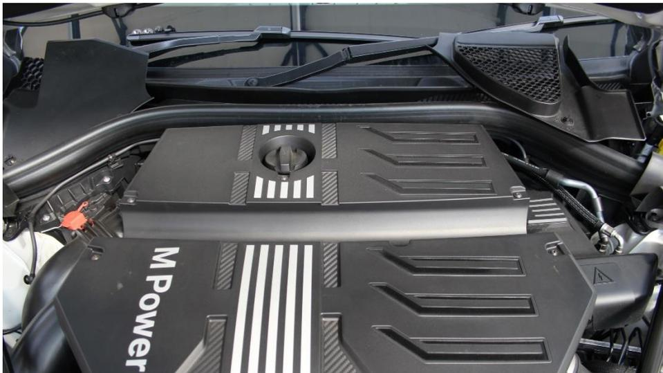
3. Remove the nuts on both sides and remove the brace.
