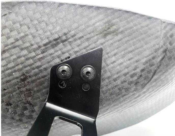
3. NON LCI – Secure the bracket to the scoop using the top holes as shown.
