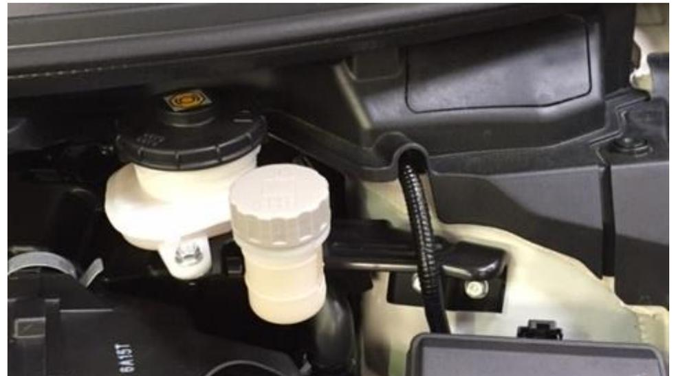
8. Now we will relocate the brake and clutch fluid reservoirs.
