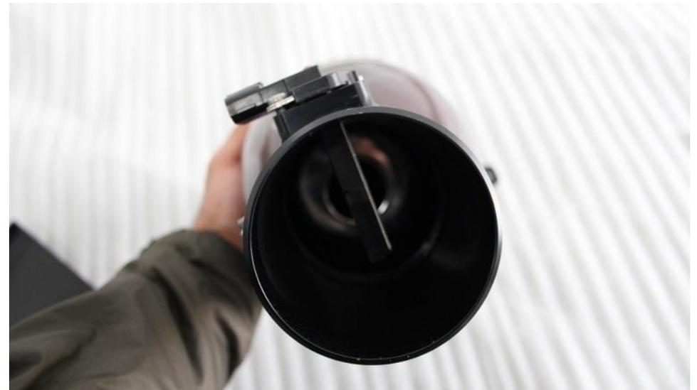
32. Orientation of the MAF sensor with the metal badge on the housing facing upwards.
