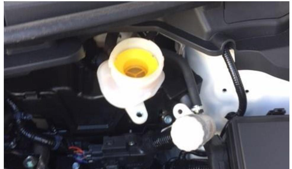
12. Empty the brake fluid reservoir using a pump or simply pouring into a container. Wipe away any spillage in the engine bay.
