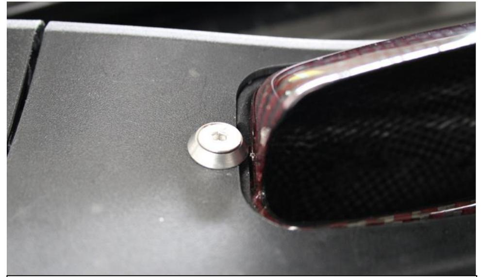
28. Be careful with the left side screw, push the washer away from the duct as you tighten to avoid scratching the carbon.
