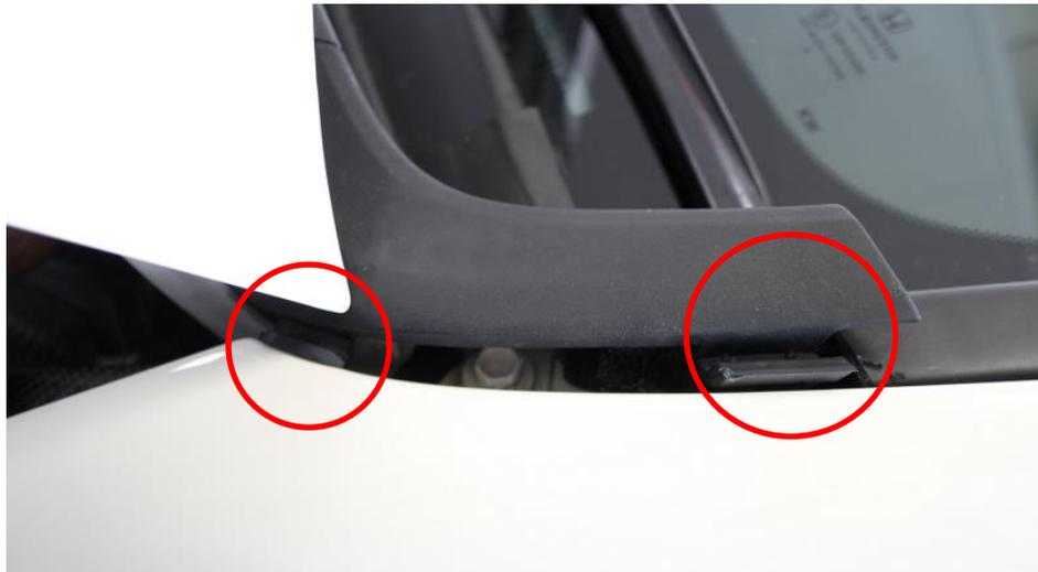
23. Now take the supplied plastic panel which has been pre-cut and install by firstly clicking the side tabs into place.
