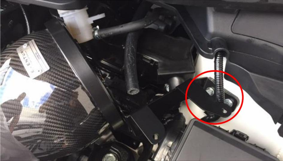
33. Position the bracket which is attached to the housing over the 2 threaded holes on the arch DO NOT secure with the supplied bolts yet. Duct and brake fluid reservoir removed for illustration purposes.
