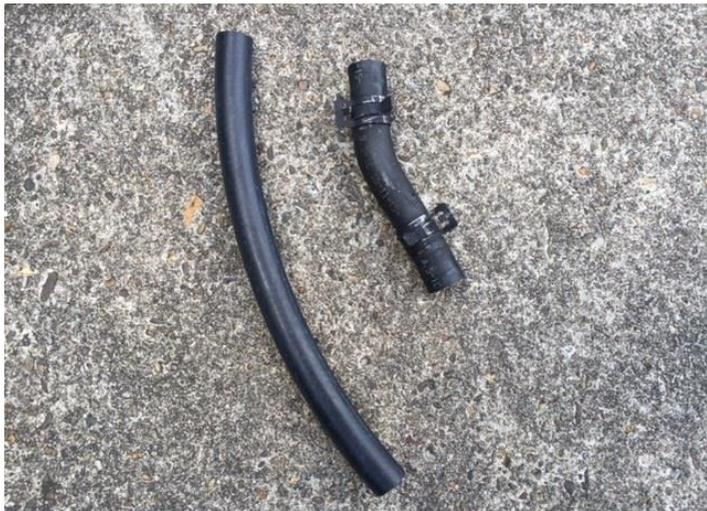
15. Remove the hose completely. Now transfer the spring clamps to the new longer brake hose supplied.
