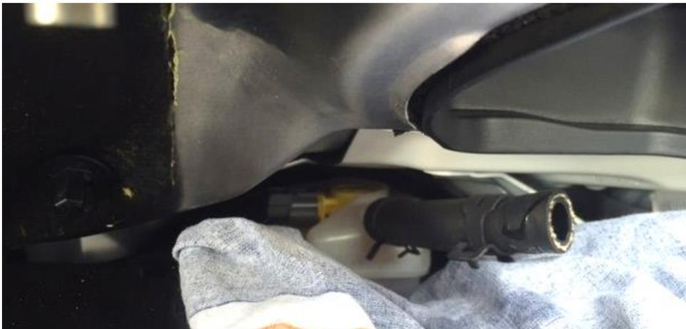
14. Place a cloth under the assembly to catch any fluid and carefully remove the reservoir from the hose. Now compress the other clamp near the cylinder and pull it away to allow removal of the brake hose.
