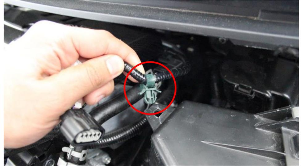
2. Remove the sensor wiring harness from the airbox – push the green tabs inwards to allow you to pull the clip out. Unplug the MAF Sensor plug.
