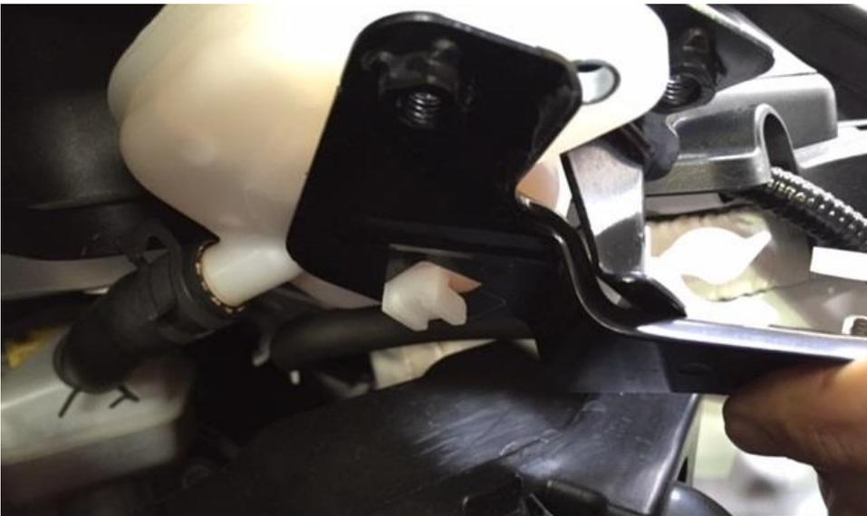
11. Remove the brake fluid reservoir from the bracket – it is hooked into the bracket from underneath.
