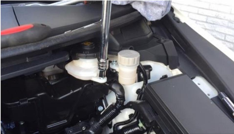
9. Remove the bolts holding both reservoirs to the bracket.
