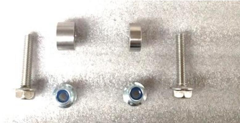
37. identify the 2 spacers, lock nuts and bolts which will now be used for the reservoir relocation. The thicker spacer will be used for the brake fluid reservoir.
