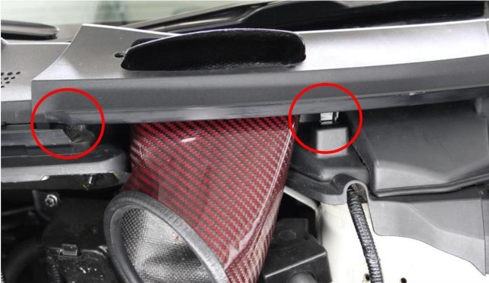
25. Now click all the tabs into place – make sure they go into the correct positions. There are tabs at the back too. Push the panel down all around to click into place.
