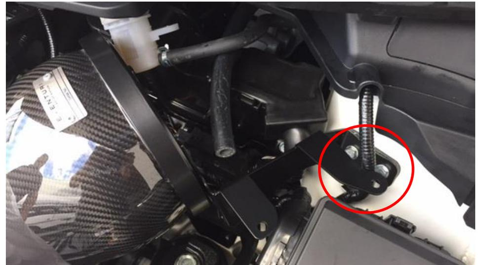
36. Now secure the intake using the 2 supplied M6 bolts. Duct and brake fluid reservoir not shown for illustration purposes.
