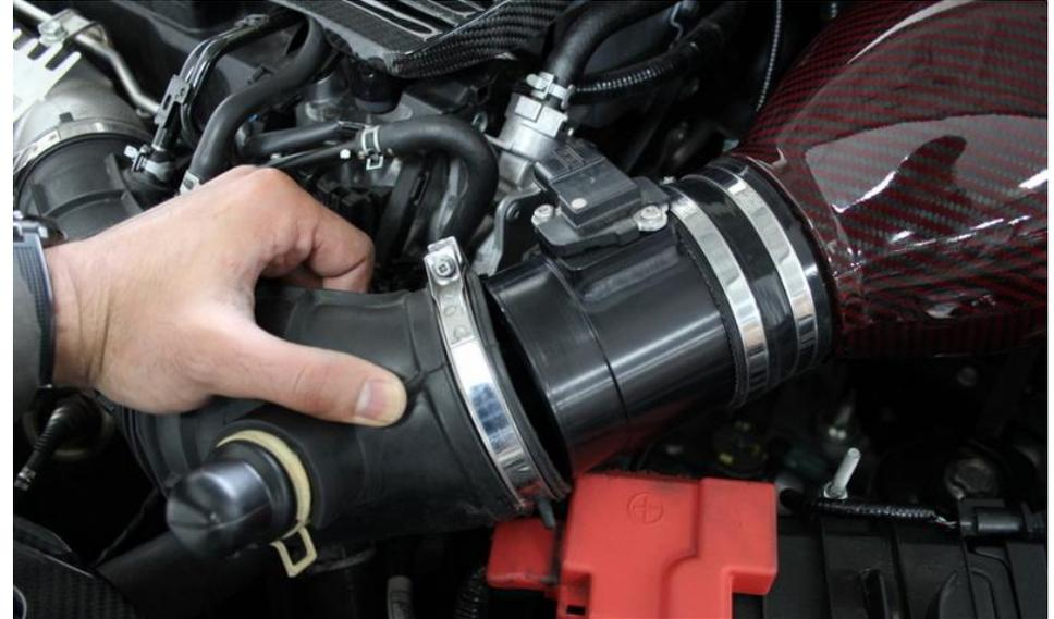
34. Push the stock rubber hose onto the MAF tube – make sure the clamp is loose. Support the housing while pushing the hose on.
