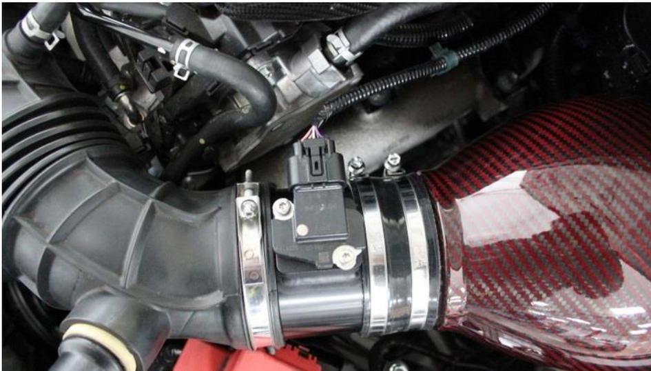
35. Tighten the hose clamp around the rubber tube. Click the MAF sensor plug into place. If the MAF sensor wire is tight, loosen the hose clamps around the silicon coupler and rotate the MAF tube further to give the wire slack.
