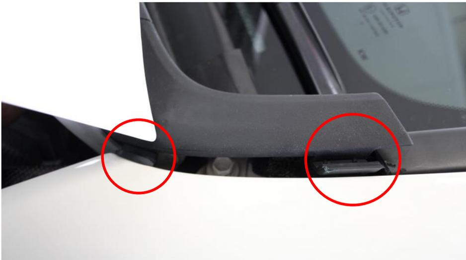
19. Unclip the 2 tabs holding the panel into the wing. Push the panel down to unclip them.
