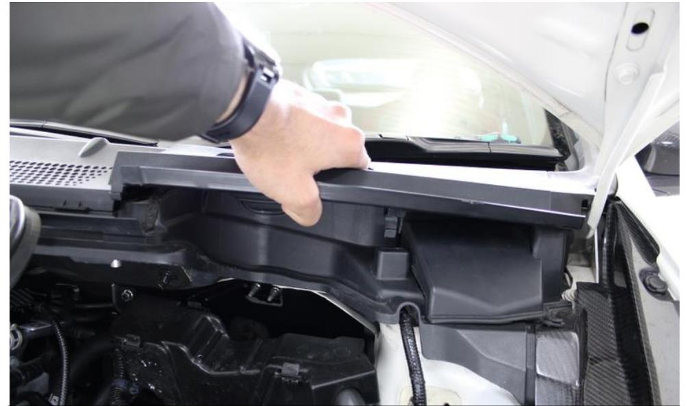
18. Pull the plastic panel upwards to unclip it.
