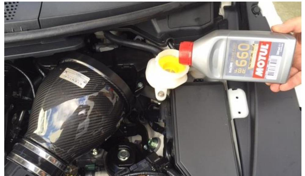
40. Fill the brake fluid reservoir with DOT 4 fluid. Do this slowly to allow the fluid to flow down the new hose. Continue to top up until fluid settles at the top of the yellow chamber. Secure the cap back onto the reservoir.
