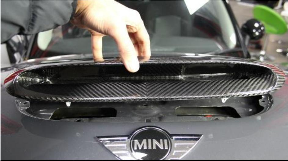
29. Carefully lower the carbon scoop into position – make sure the 6 clips are already installed on the back of the scoop.
