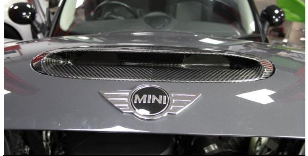
30. Once the clips are in position firmly push the scoop down in all 6 clip positions and ensure they click into place.
