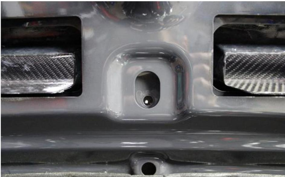
31. Once clipped into place – secure the scoop by screwing the torx screw removed in step 24. IF your scoop came pre-assembled with a new screw in this position from step 28 – use the new screw to secure the scoop.
