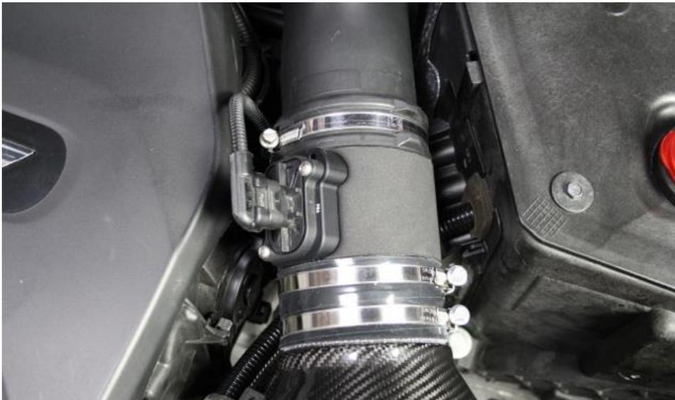
19. Re-connect the MAF sensor – ensure is fully clipped back into the sensor. Now tighten the remaining hose clamps.
