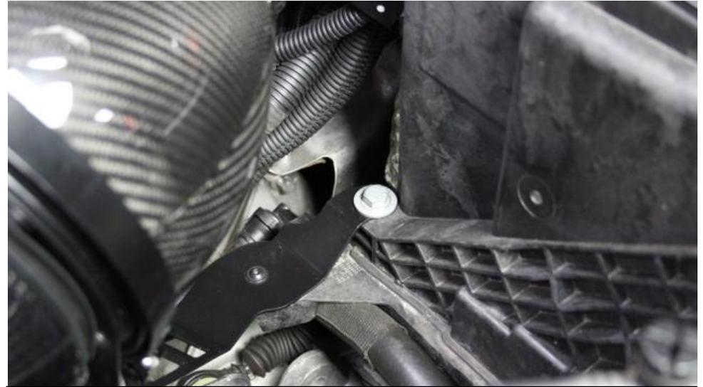
18. Once the duct and housing are aligned – secure the bracket with the bolt removed in step 5.
