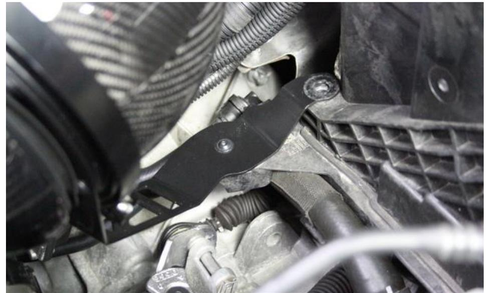
16. Once inserted the bracket should sit like this. Do not secure yet.
