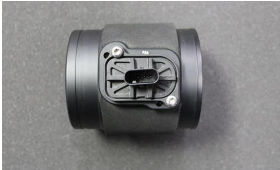
7. Insert the MF sensor into the new tube and secure with the 2 x supplied torx screws. DO NOT use the OEM screws for this. LCI version shown in next step.
