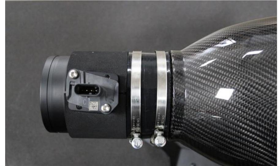
10. Similarly here is the LCI version. Assemble the MAF tube to the filter housing using the silicon coupler and 2 hose clamps. The tube must be inserted into the silicon as shown here. It is VERY IMPORTANT to get the sensor direction correct. You can see the arrow on the sensor indicating flow direction.
