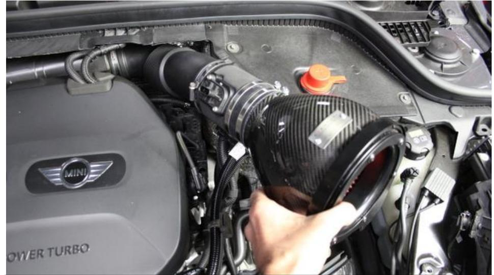
14. Push the filter housing and MAF tube into the stock intake tube.
