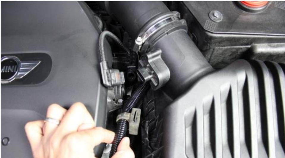
3. Disconnect the MAF sensor and remove the rubber holder from the airbox.
