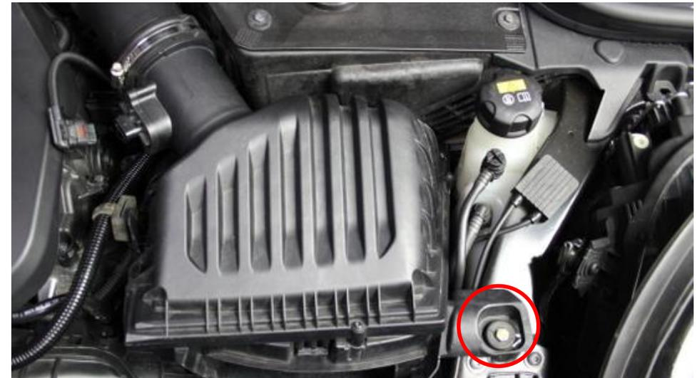
4. Loosen the hose clamp around the tube at the back of the airbox and remove the 10mm bolt as circled.
