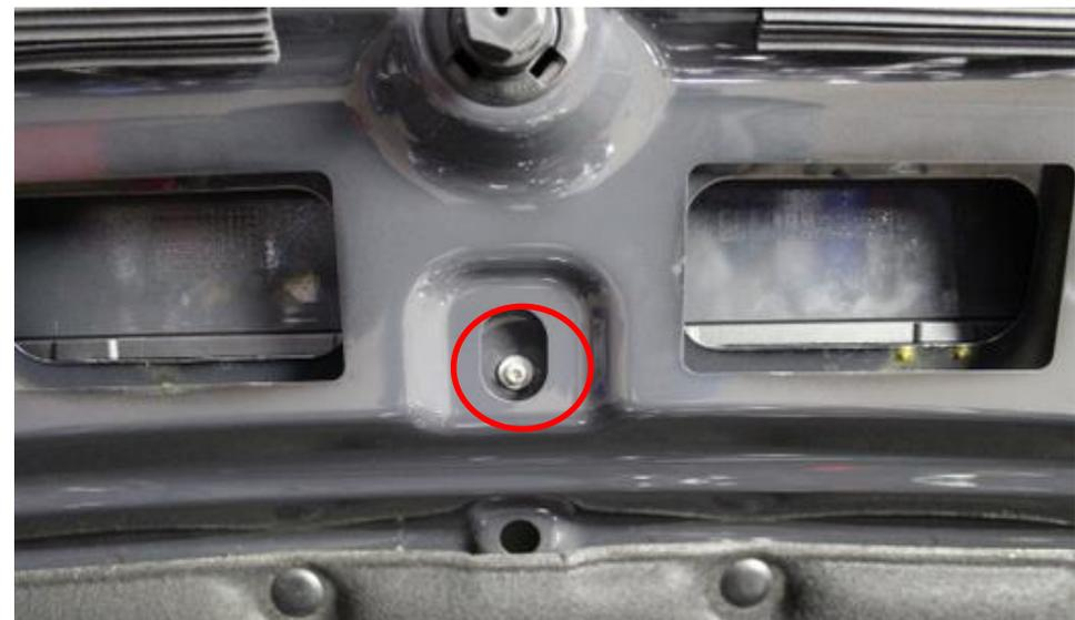
24. Now we will remove the bonnet scoop. Start by removing the torx screw shown.
