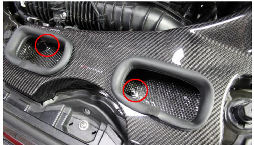
20. Now secure the duct with the 2 x M6 nuts.
