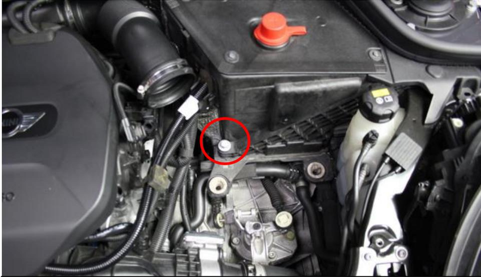
5. The airbox can now be lifted out of the engine bay. Also remove the bolt at the base of the battery tray as circled. This will be required to secure the intake later.
