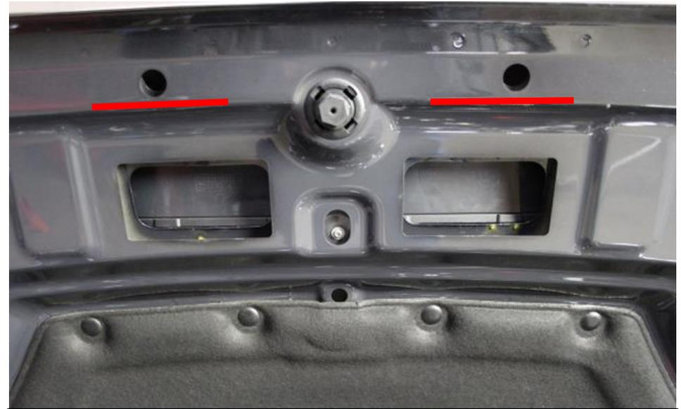
22. Remove the adhesive backing from the strips and apply them as shown by the red lines under the bonnet. The next photo shows how they should look once applied.
