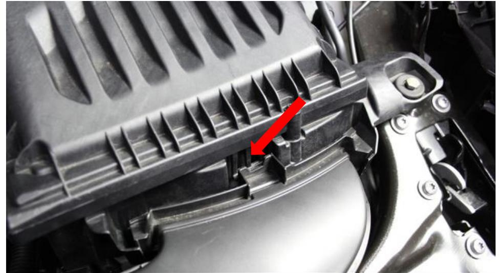
2. Release the front of the duct by pushing in the clip on the airbox.
