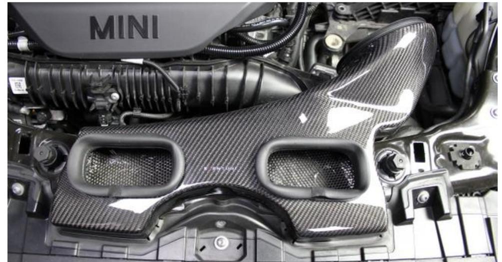
12. Insert the carbon duct into place – the 2 threaded studs should go through the holes in the base of the duct – see the next photos.
