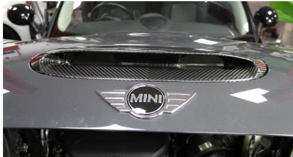
33. Once the clips are in position firmly push the scoop down in all 6 clip positions and ensure they click into place.
