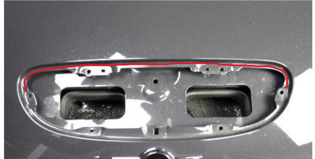
30. Stick the sealing strip to the scoop area marked in red. It should go between the 2 holes on each side. See next photo. Do not cover the holes.
