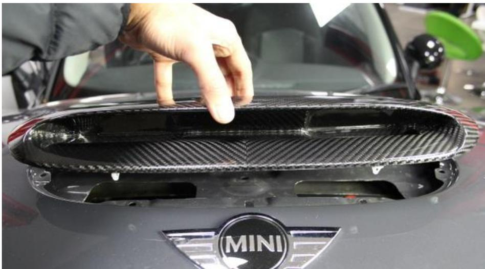
32. Carefully lower the carbon scoop into position – make sure the 6 clips are already installed on the back of the scoop.
