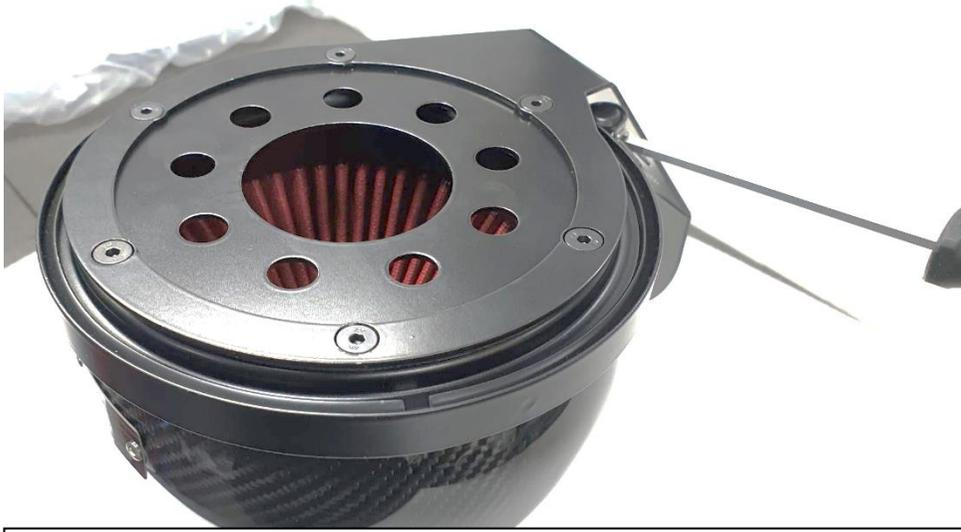
17. Place the V-band around the housing the latch of the v-band must be under the bend of the housing bracket. Secure with 4mm Hex screwdriver
