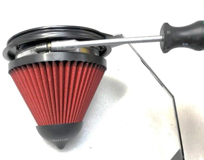
13. Secure the filter to the housing bracket assembly with a 7mm socket
