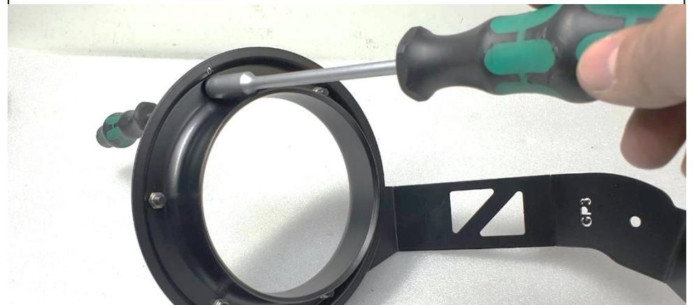
4. Once the housing bracket assembly has been removed unscrew the housing bracket from the cowl with an 8mm socket and 3mm Hex screwdriver.
