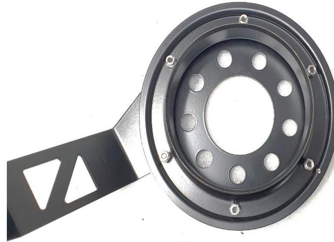
10. On the other side of the housing bracket screw on the M5 Aero Nuts on to the M5x16 screws
