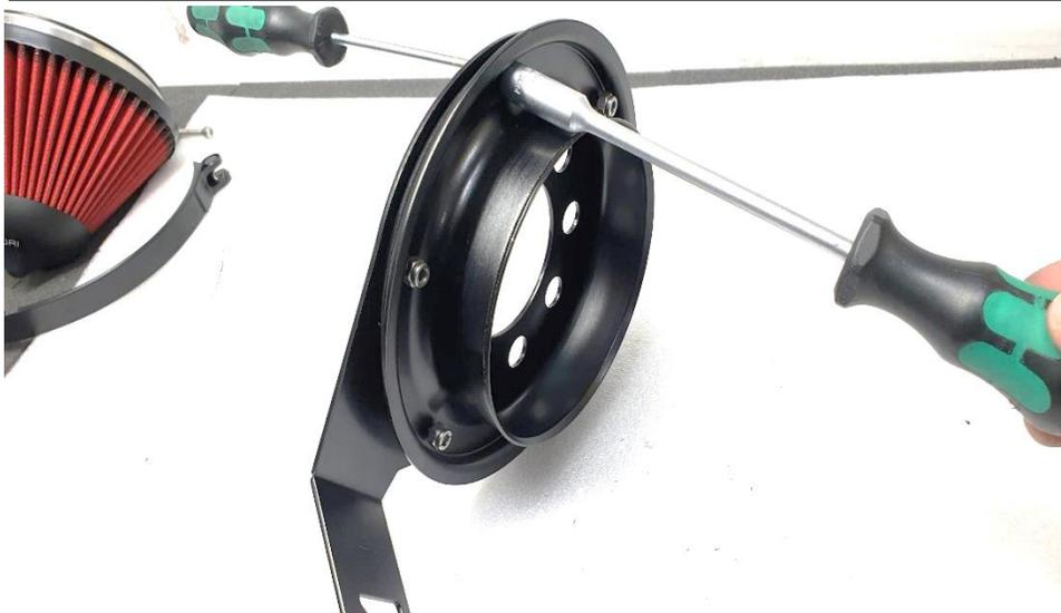
11. Secure the M5x16 counter sunk crews with 8mm socket and 3mm Hex screwdriver
