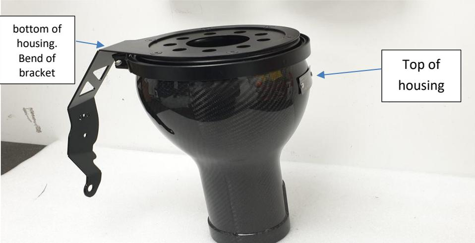
15. Insert the filter assembly into the housing make sure that the bend of the housing bracket is at the bottom of the housing. (The side where the Eventuri plaque is located is the Top of the housing, so it should be opposite this)
