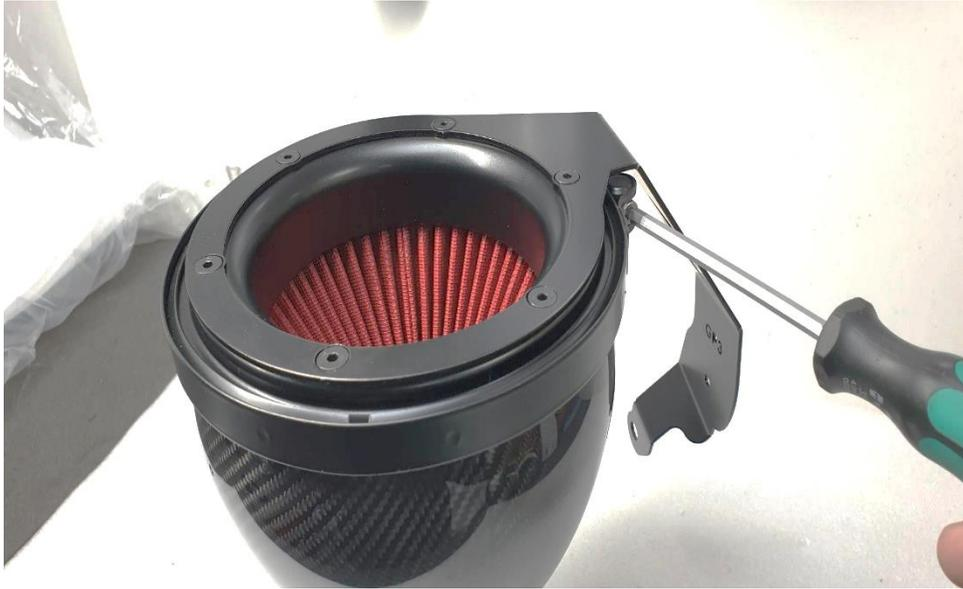
2. Unscrew and remove the V-band which is holding the filter to housing with a 4mm
