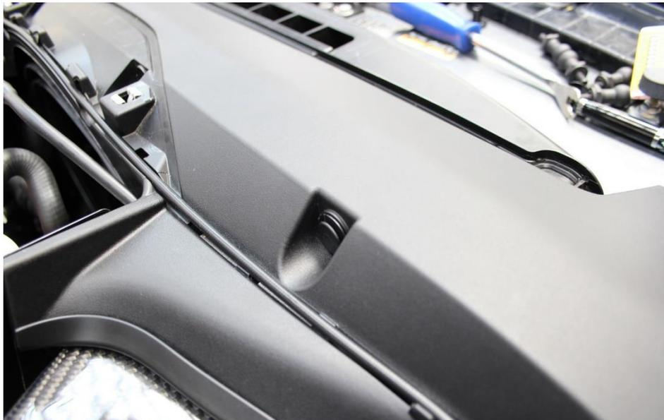
39. Push the bonnet cable back into place and secured the panel with the OEM push clips.
