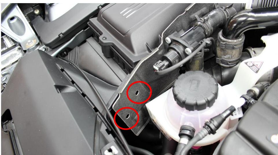
1. We will start by removing the left side stock airbox. Remove the plastic centre cover. Remove the 2 plastic push clips in the heat shield.
