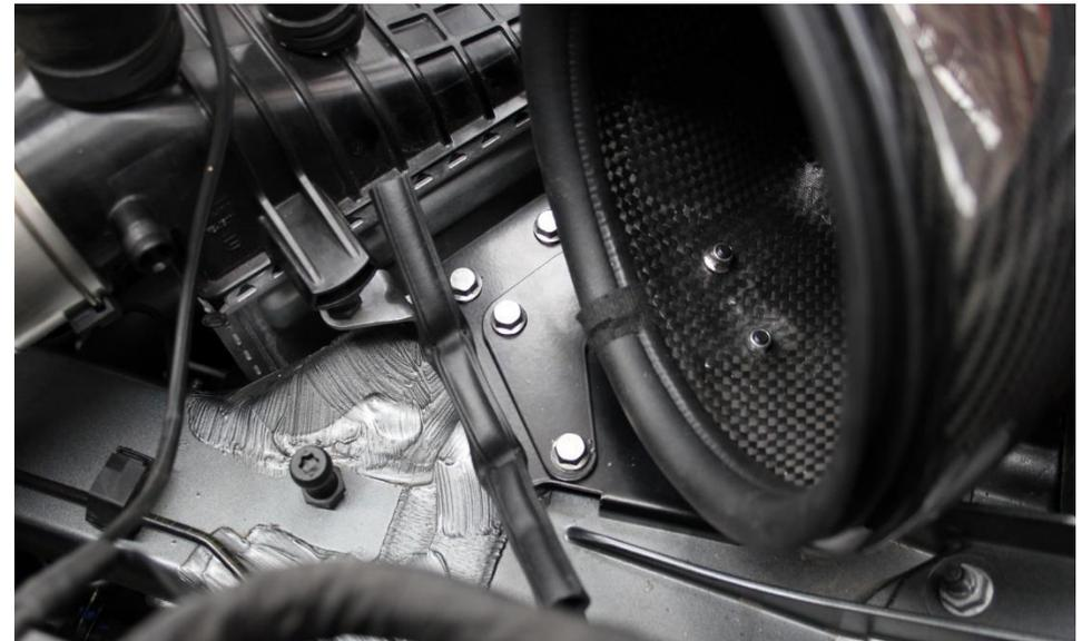
20. Secure the front of the duct onto the base bracket using the 2 M6x12 bolts.
