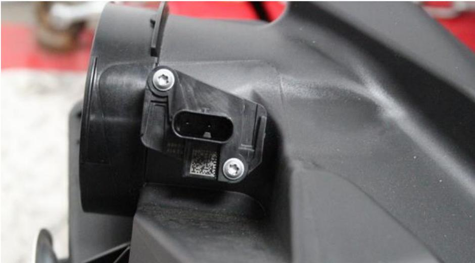
7. Remove the temperature sensor from the airbox.
