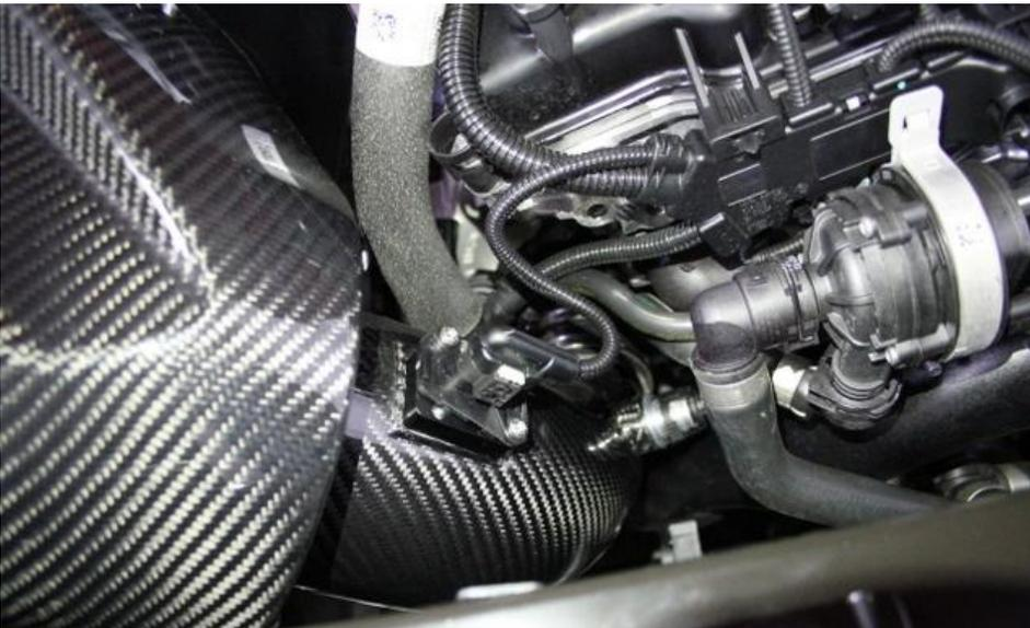
23. Connect the temperature sensor plug.
