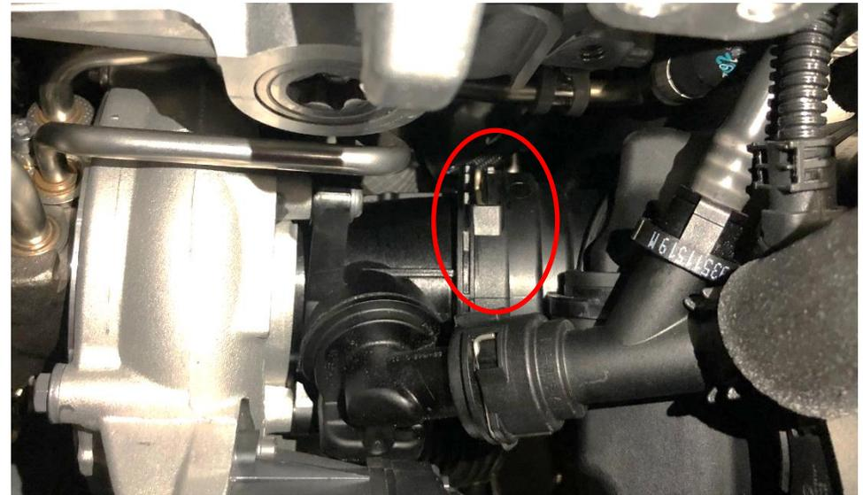
4. Pull the spring clip away from the tube flange and this will allow you to pull the tube away from the turbo. There is also a breather connector to remove – see next step.
