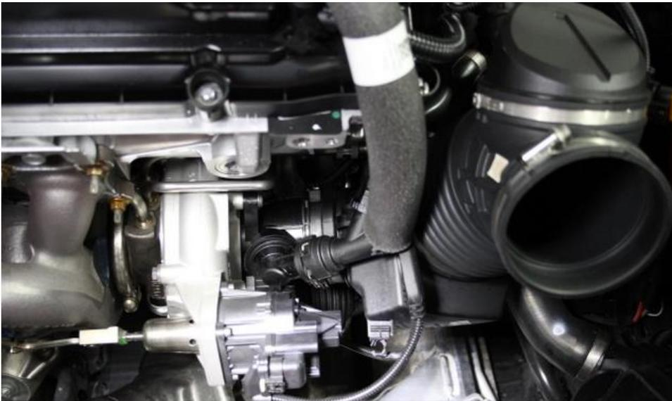
3. To remove the rubber intake tube – firstly pull out the spring clip around the tube at the turbo inlet end. The next photo shows a close up.
