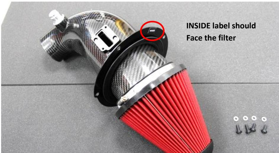
11. Push the sealing plate onto the tube – ensure the **INSIDE** label is facing the filter side. Now push the filter fully onto the tube and secure with the attached clamp.
