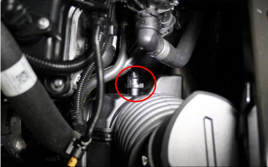
5. Remove the breather connector from the tube.
