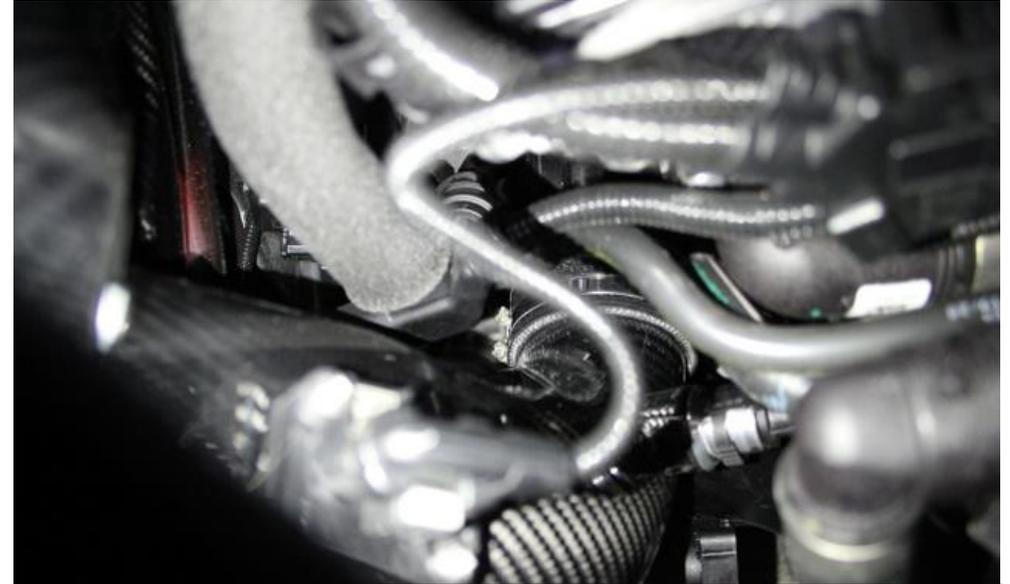
22. Secure the remaining hose clamp around the carbon tube – DO NOT overtighten.
