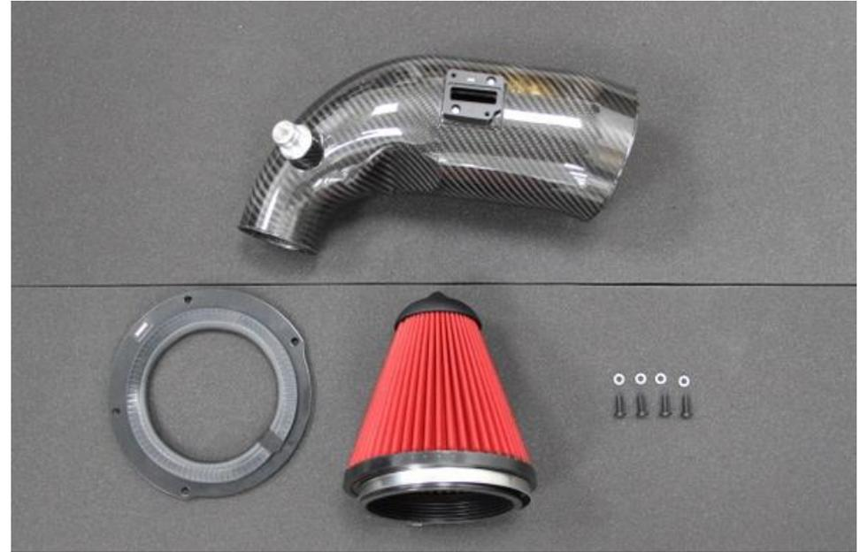
10. Take the inlet tube, filter, sealing plate and the M5 screws with lock washers.
