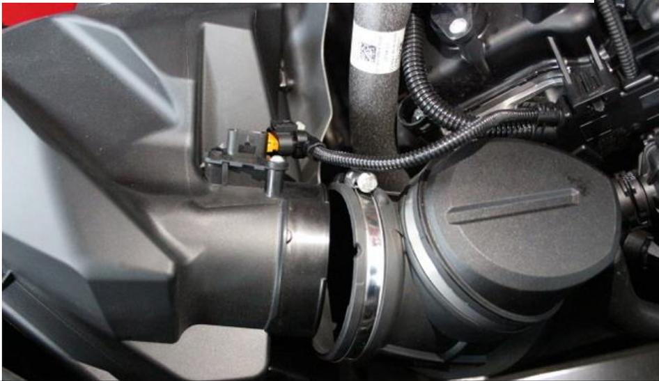
1. We will start by removing the stock airbox. Loosen and remove the rubber inlet tube and disconnect the temperature sensor plug.
