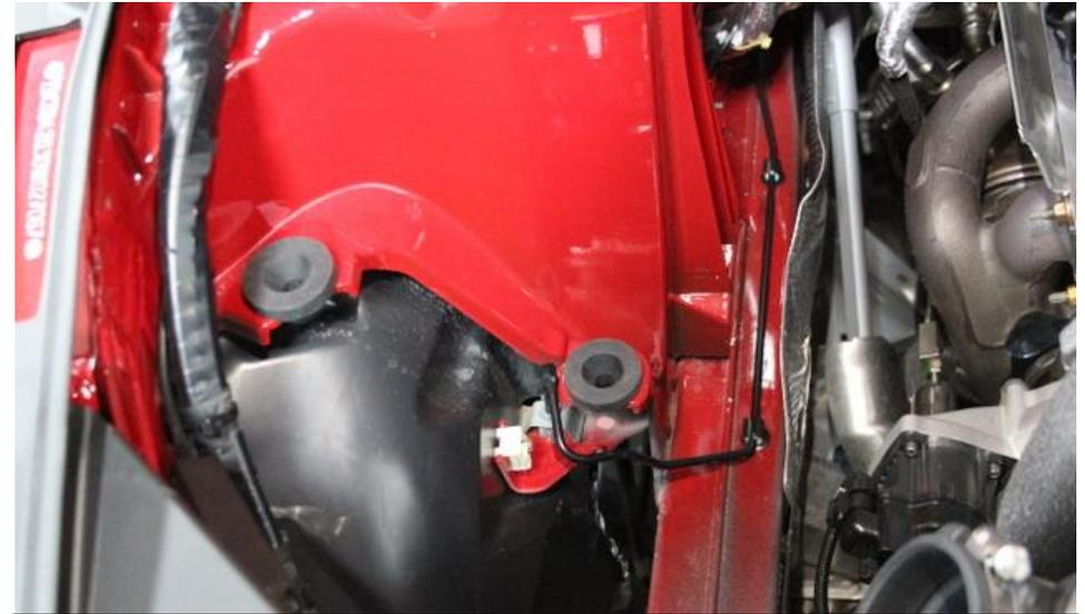
2. The airbox can now be pulled out. Make sure the rubber mounting bushes are still on the car – if not, remove from the airbox and install back onto the chassis.
