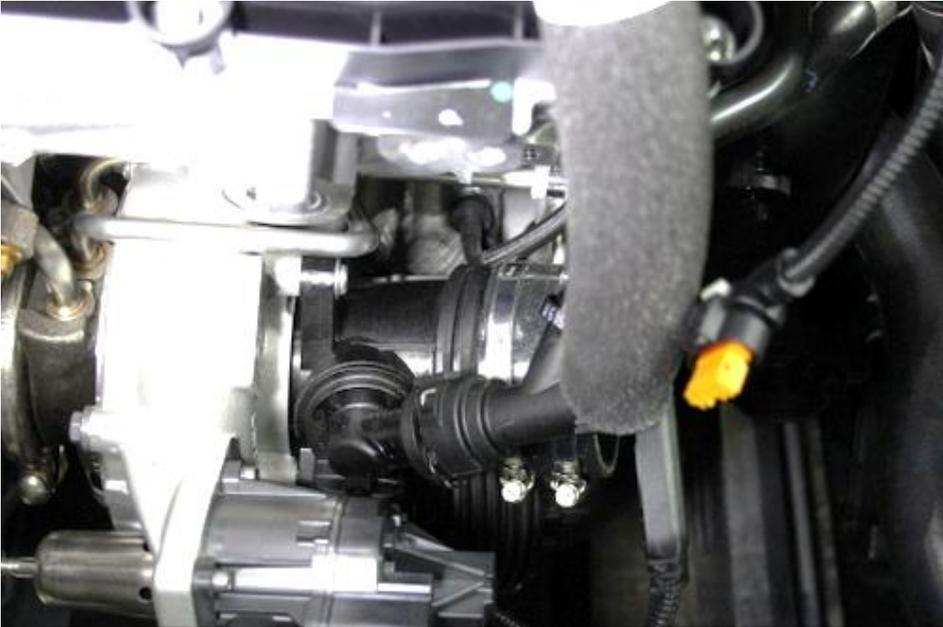
9. Hose clamps accessible from the side. Tighten the clamp around the turbo side. Leave the other one loose.
