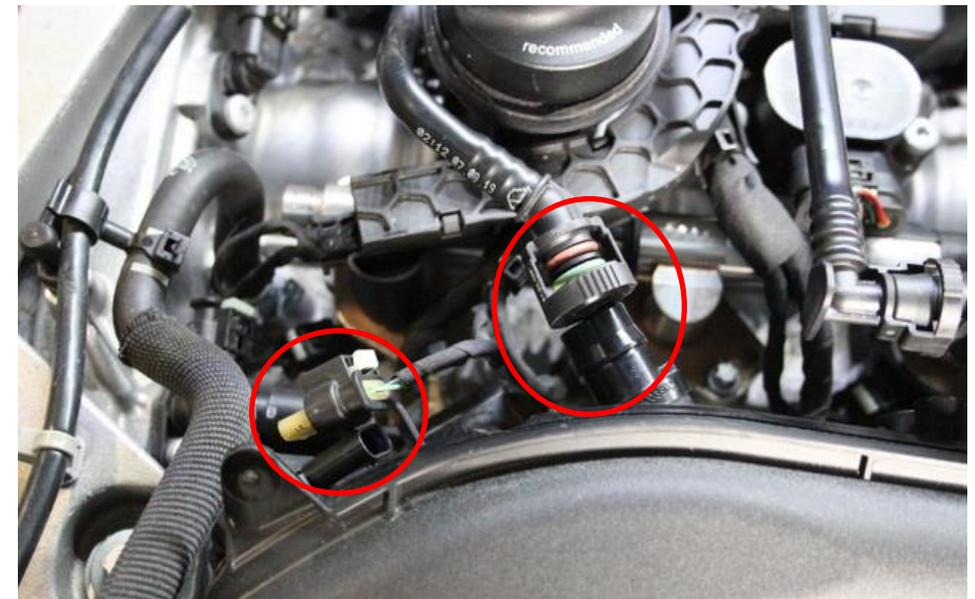
4. Remove the remaining single breather pipe and unplug the MAP sensor plug.
