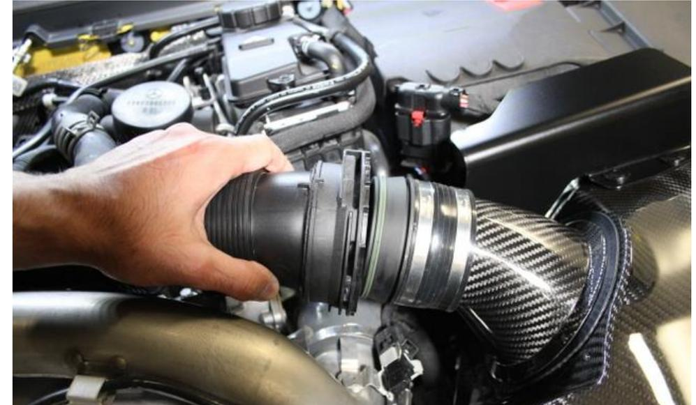
12. Remove the tube from the airbox side.
