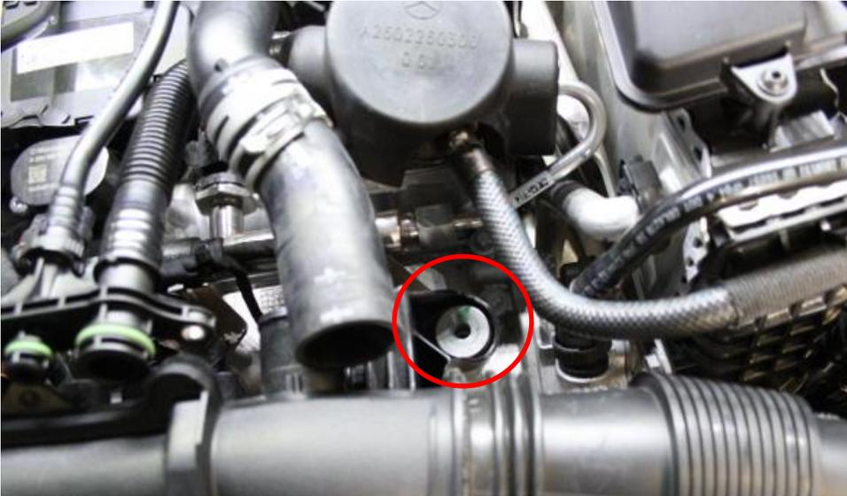
5. Remove the bolt on the mount as shown.
