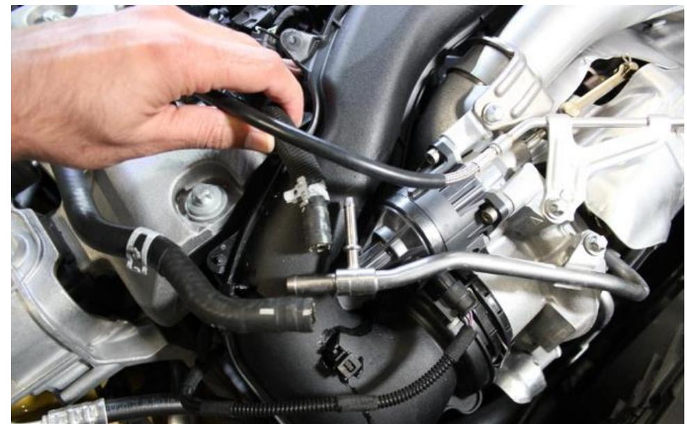
8. Remove the coolant lines as shown.
