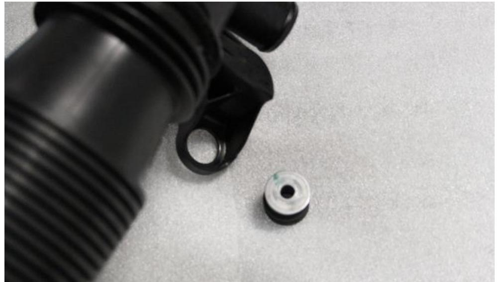
28. Remove the second rubber mount from the original tube.
