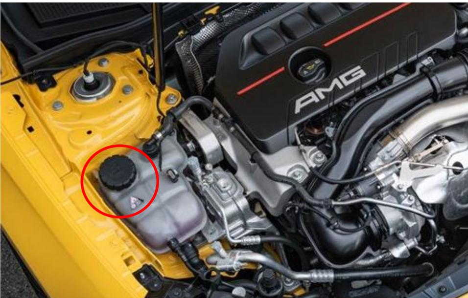
7. **MAKE SURE THE ENGINE IS COLD.** Release any pressure in the coolant system by removing the coolant cap.
