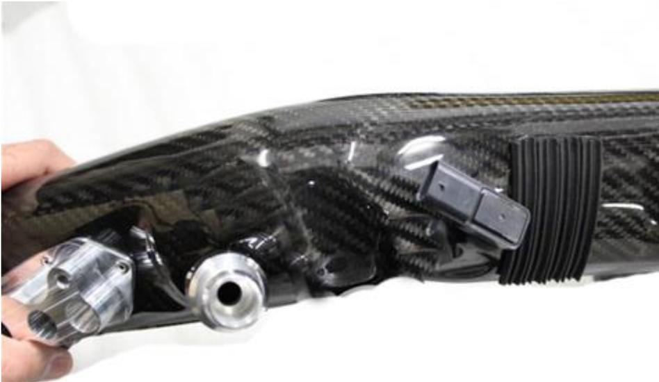
17. Install the MAP sensor and angle it as shown.
