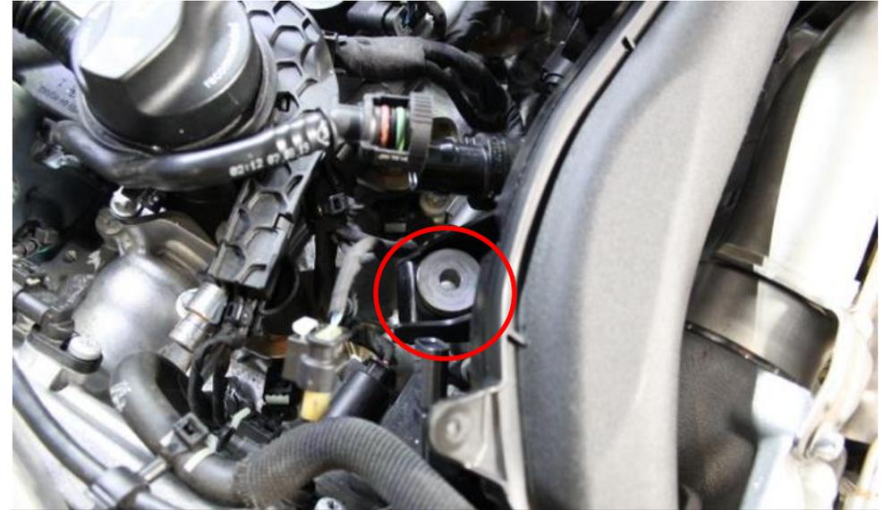
6. Remove the remaining bolt on the other side.
