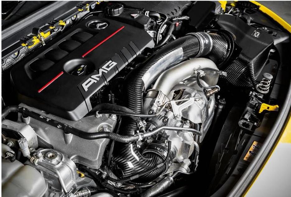
**You have now completed the installation of the Eventuri A35S intake system.**
