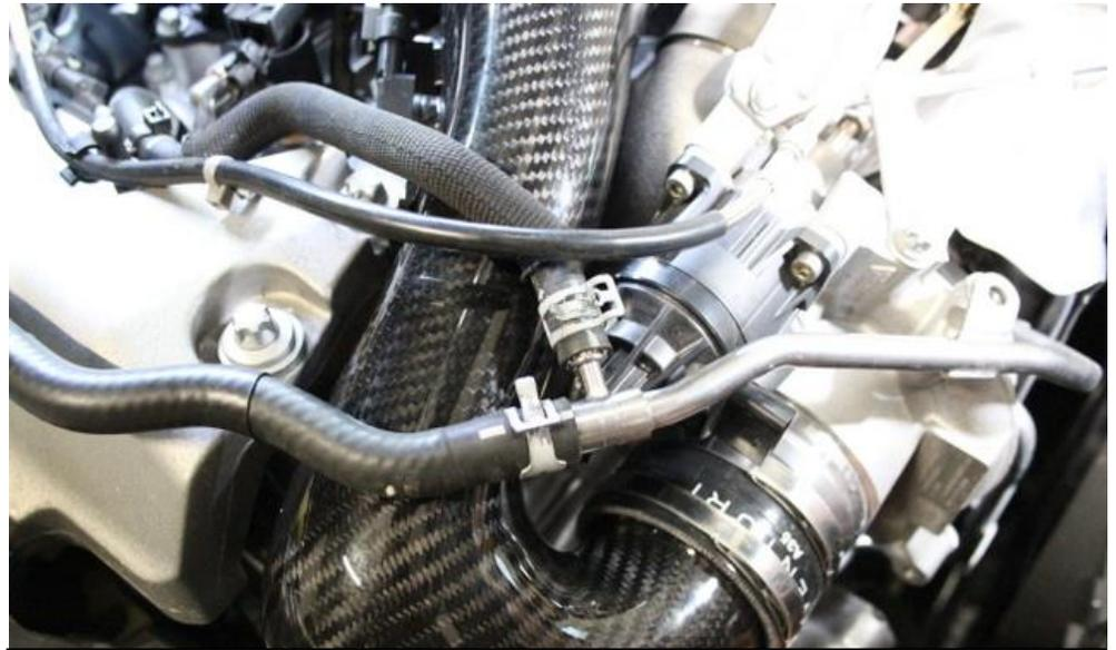
30. Re-connect the coolant hoses and the clamps.
