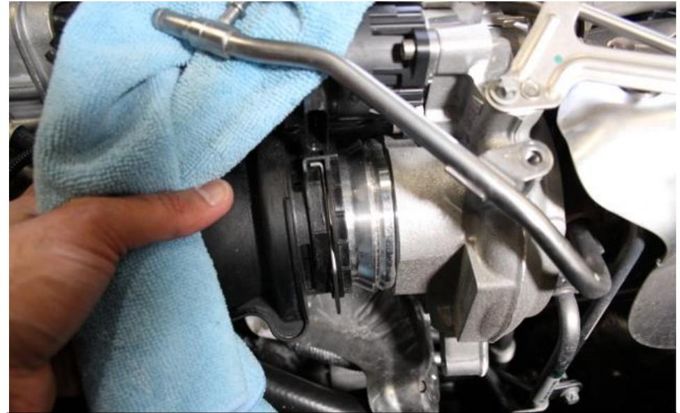
14. Remove the tube from the turbo.
