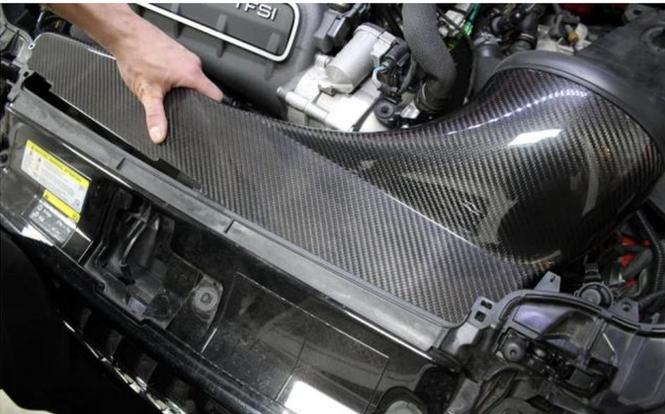
19. Keep lowering carefully positioning the carbon into the mounting area.
