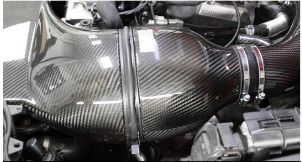
34. Rubber cushion should be evenly compressed. There will be some movement in the silicon hoses to allow correct orientation before tightening the 2 lock nuts ensure hose clamps are loose.
