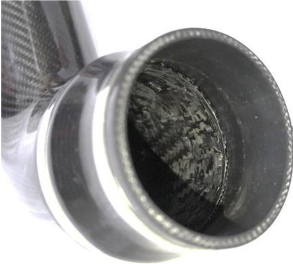
25. Push the tube down into the silicon so that it meets the start of the reduction part of the silicon. Make sure it is even all the way around and secure the clamp around the tube only.
