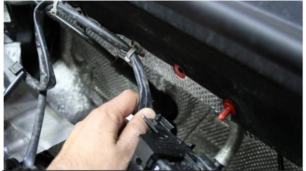
10. We need a bit more slack in the wiring – carefully pull the wiring through the cable ties to allow the pugs to drop down a little more. You only need a few centimetres extra.
