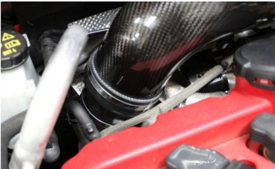
27. Ensure the hose clamps are evenly positioned around the silicon on both sides. It is easier to position the screw parts at the back facing the right – you have access behind the tube. Do NOT secure the clamp around the turbo yet.
