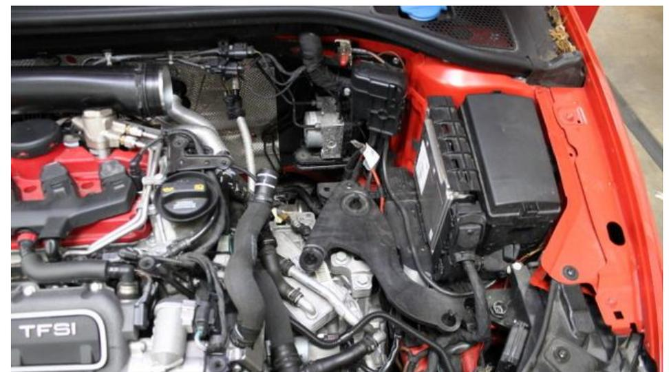
4. Remove entire airbox by pulling upwards. It is held in place with rubber push mounts.
