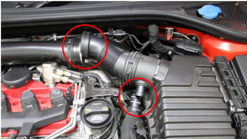
3. Remove spring clamp from flexi hose at the turbo pipe connection – use an appropriate spring clamp tool. Pull out the flexi hose from the turbo tube. Also remove the small engine cover and breather hose from the airbox.
