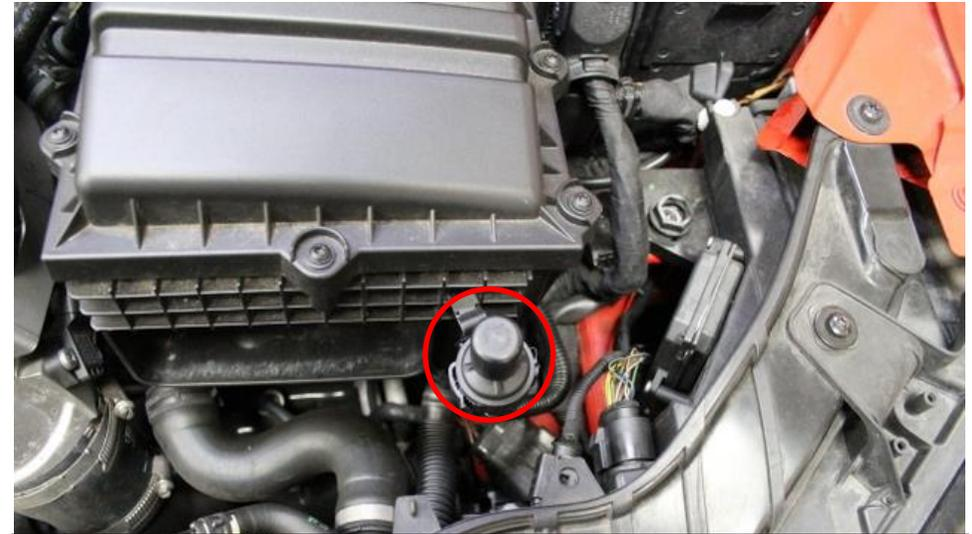
2. Remove the sensor pot from the airbox – it is held in place with a panel clip – use a small flat head screwdriver to prise the clip open if required.
