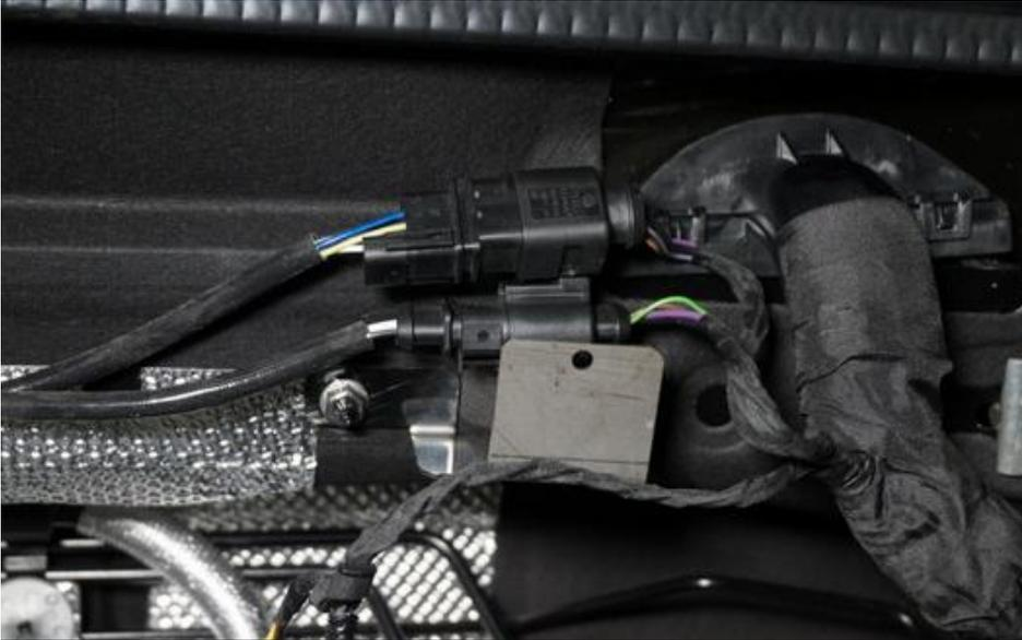
13. Install the new bracket onto the threaded stud as shown and secure with the supplied M6 Nut.
