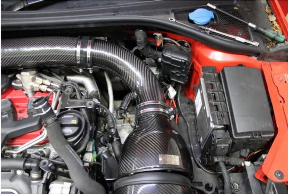
29. Insert the lower tube into the silicon on the turbo tube. Ensure the hose clamp is loose enough. Position the housing so that it sits behind the duct.
