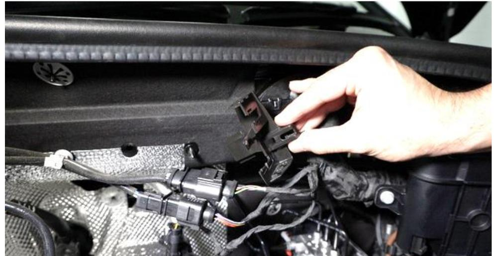
12. Remove the plastic bracket completely.
