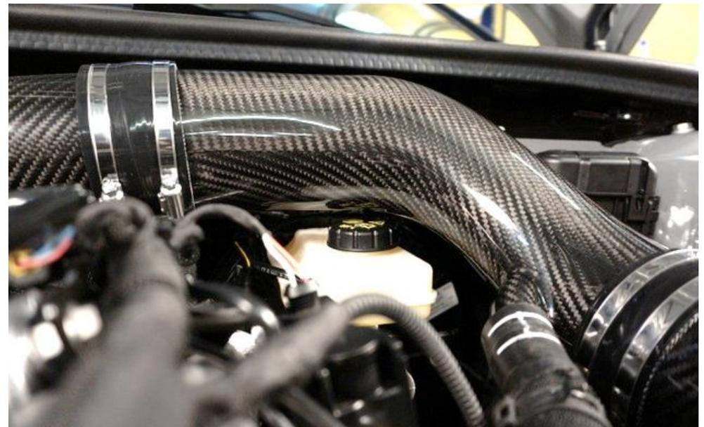
36. Check the clearance above the reservoir again (LHD only) and then tighten the hose clamps on both sides of this lower tube. Do not overtighten.
