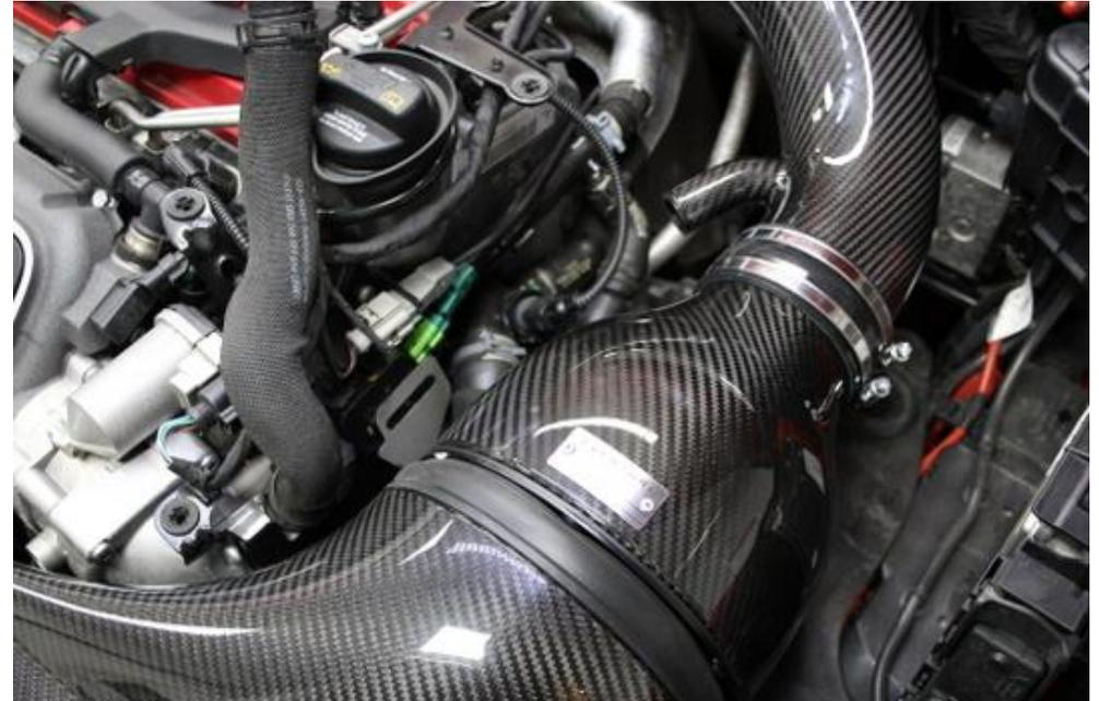
30. Rotate the housing so that the brackets line up – see next step. Ensure the rubber cushion on the duct is sitting squarely on the housing.
