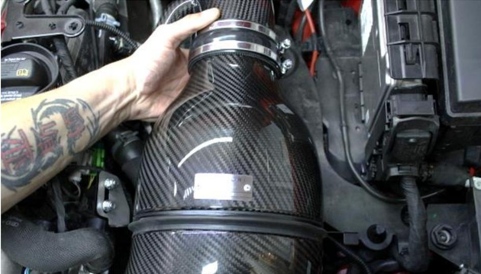
33. Pull the housing towards you so that the rubber cushion on the duct compresses. Ensure it is compressed evenly all around and while maintaining pressure – tighten the 2 lock nuts on the bracket.
