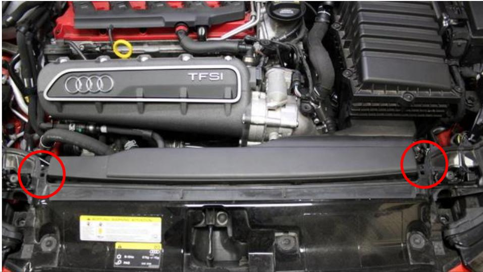
1. We will start by removing the stock airbox system. Remove the 2 screws holding the inlet duct in place. Then push the duct into the airbox to release the mounting points and remove duct from engine bay.
