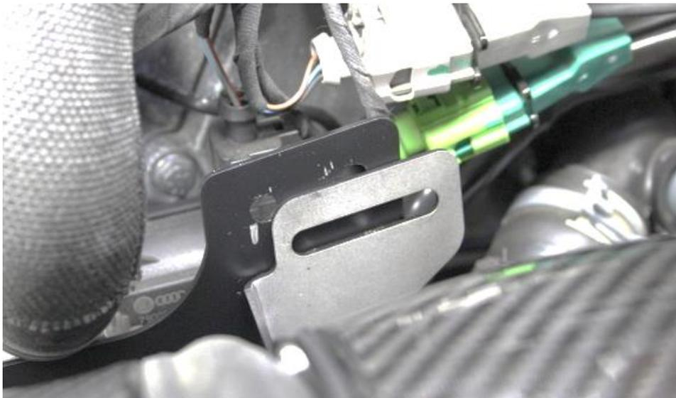
31. Rotate and position the housing so that the slot on the housing bracket lines up with the holes on the bracket previously installed.
