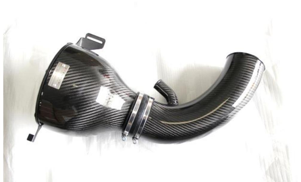
28. Assemble the remaining tube (LOWER TUBE) with the filter housing as shown. Do NOT secure the hose clamps yet. They must be loose enough to allow rotation of the housing.
