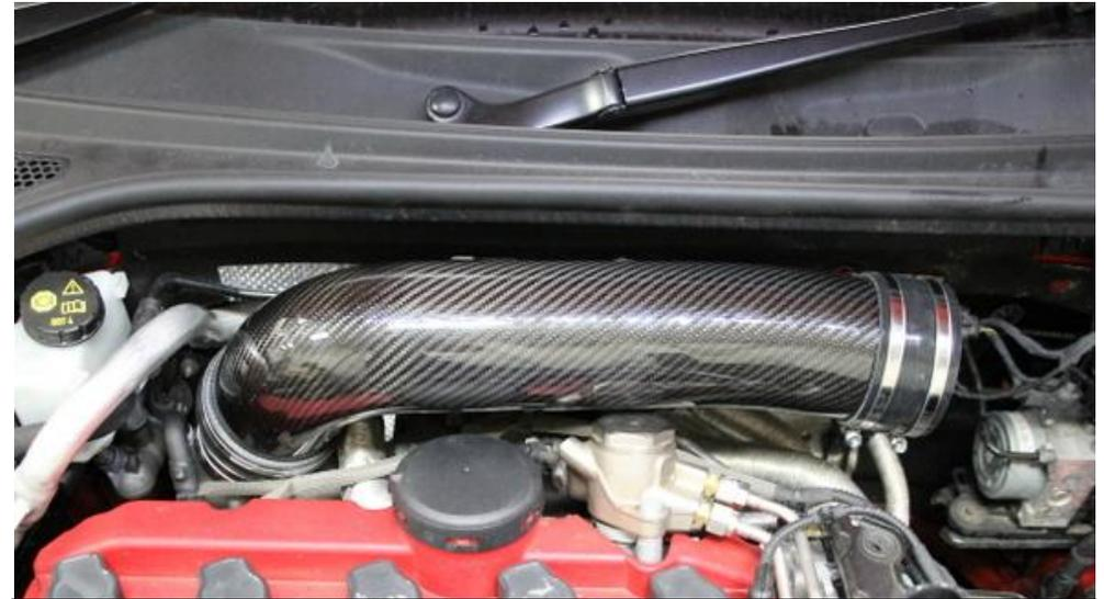
26. Push the silicon reducer onto the turbo – make sure it is pushed all the way down and the silicon is even around the turbo.
