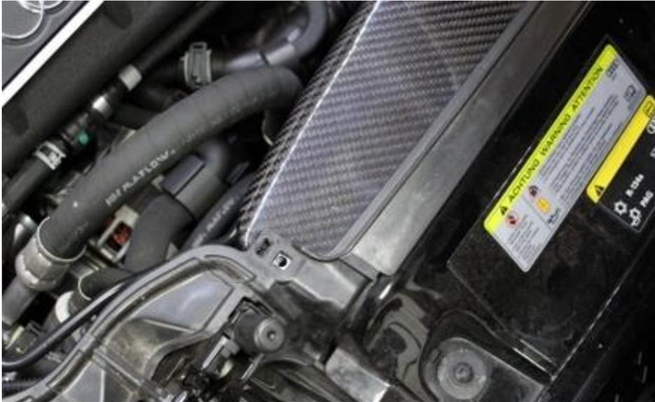
21. This is the final position of the duct – line up the hole on the panel with the threaded insert on the carbon. Secure with a supplied M5 Screw DO NOT use the original screws.
