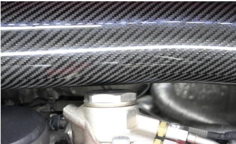
35. Orient the turbo tube so that there is approximately a 10mm clearance gap above this engine component as shown. Now ensure the silicon reducer is still squarely on the turbo and tighten the hose clamp around the turbo.
