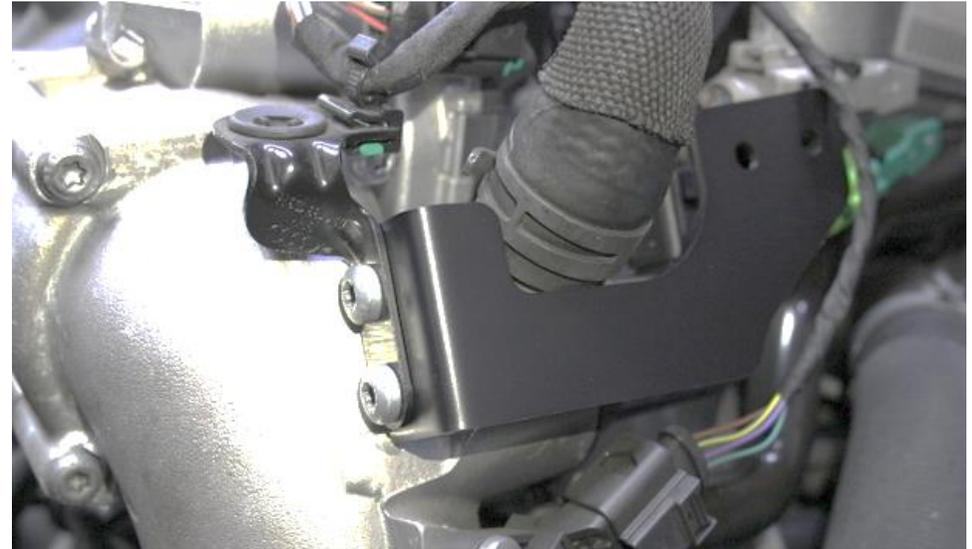
16. Install the new bracket for the intake as shown. Put the original bracket from the previous step on TOP of the new bracket and secure with the same 2 Torx screws.
