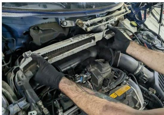
16. Release clamps. Release clean air pipe from intake silencer housing.
