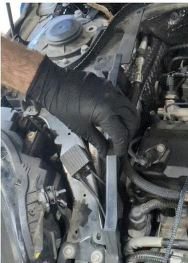
13. Release expanding rivets (1). Remove mounting for engine compartment lid gasket.
