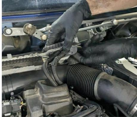
11. Release expansion rivet and release screw.
