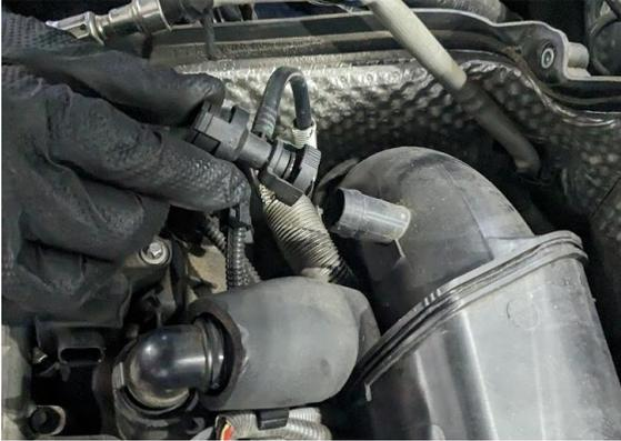
20. Unlock clamp at the turbo inlet.
