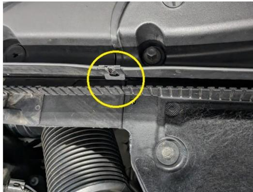
34. Install top bulkhead cover. Reinstall seal.
