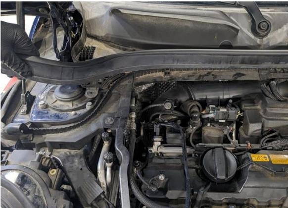
4. Remove clip (1). Loosen 2 Cap nuts (2). Open 4 Locks (3) by turning them counter-clockwise.
