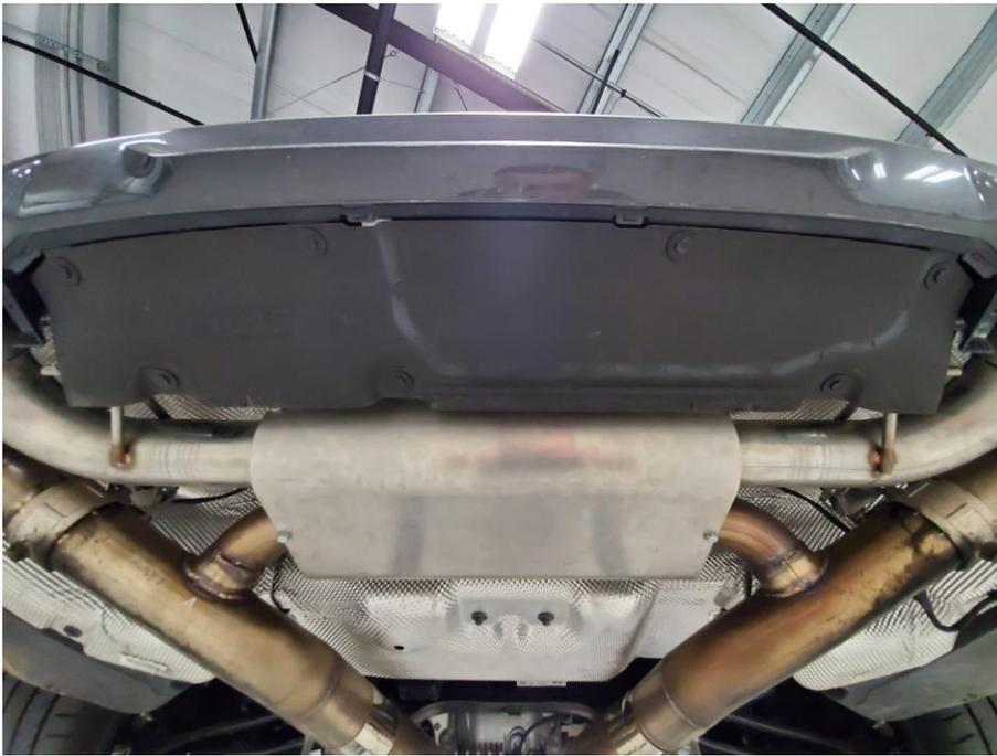
16) Push the muffler up and forward then torque the clamps. If the muffler contacts any part of the car, twist the inlet pipes to adjust. Allow for the pipe clearances as pictured below.
