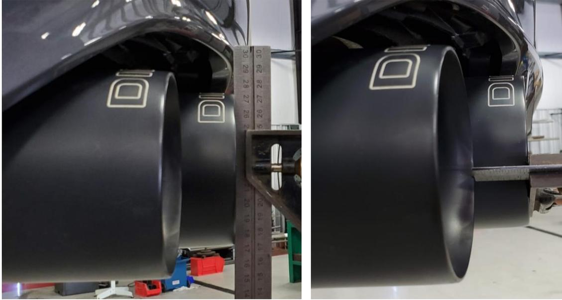
18) After adjusting the tip length and alignment, make sure the second vertical line of the N in the Dinan logo is facing straight up on all 4 tips.
