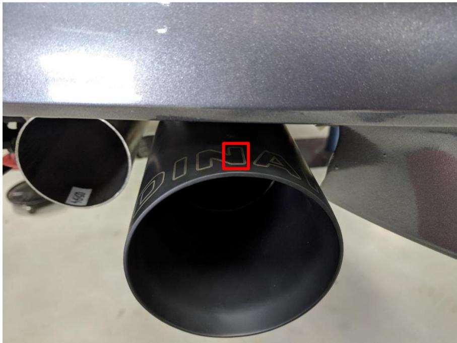
19) The exhaust tips should fit on both sides as pictured below. Torque the exhaust tip clamps to 45 ft-lbs.
