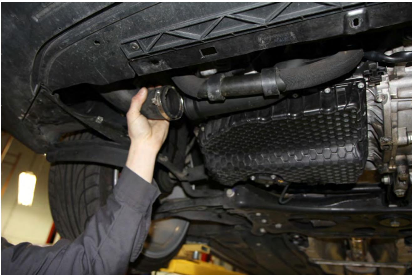
**Step 4 - Unclip the coolant hose**
