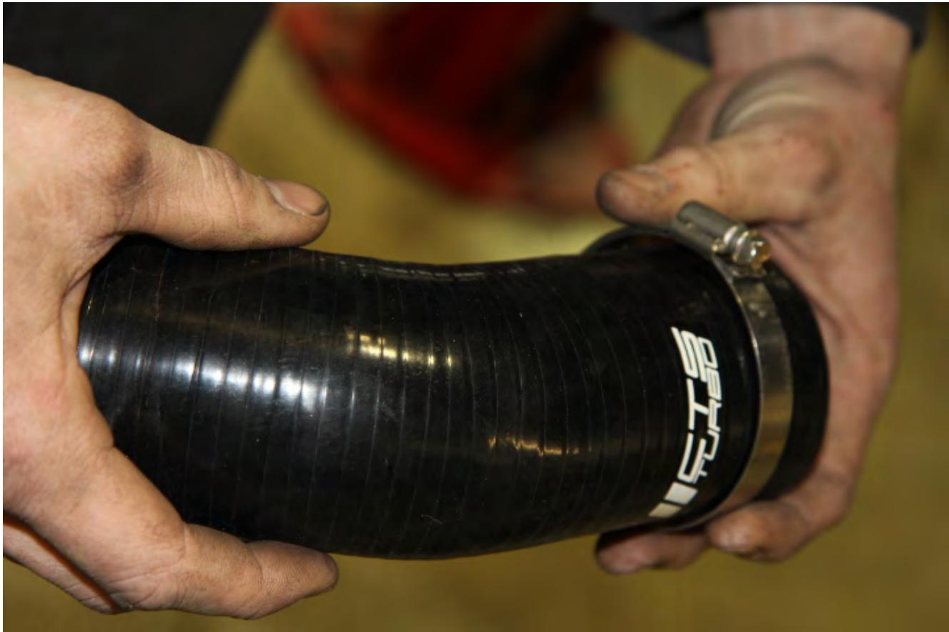
**Step 11 - Slide the silicon over the throttle body**
