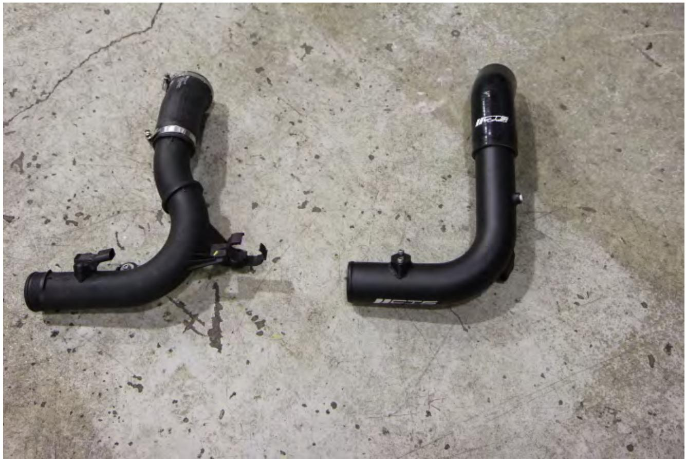
**Step 9** - Remove the map from the throttle pipe using T20 and transfer map to the new pipe
