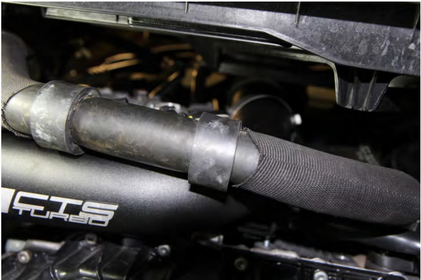
**Step 14** - Slide the bracket over the bolt
