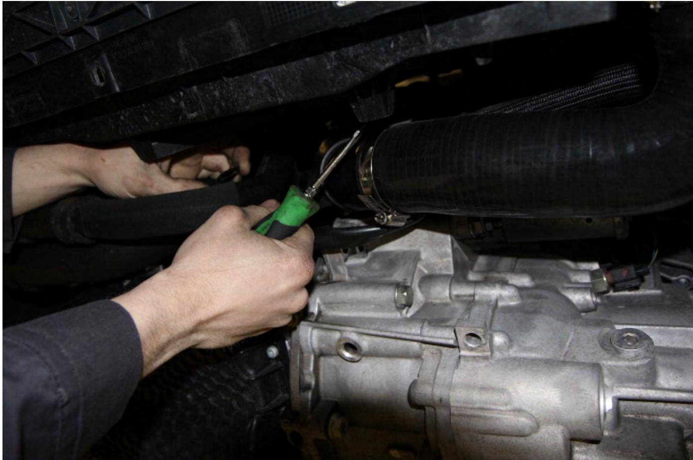
**Step 5 - Undo undo both brackets T30**
