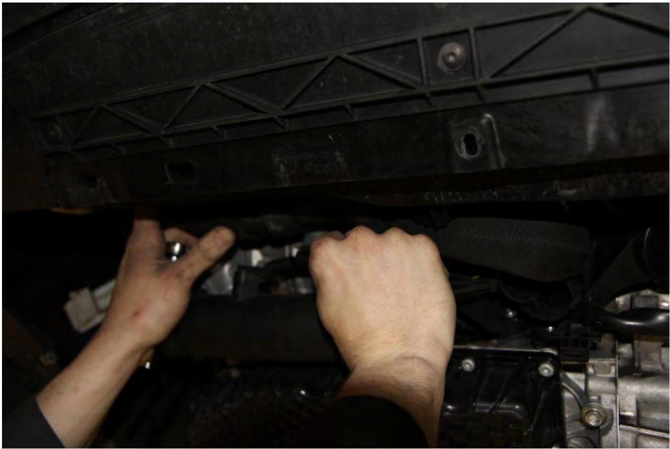
**Step 7 - Undo the silicon from throttle body**
