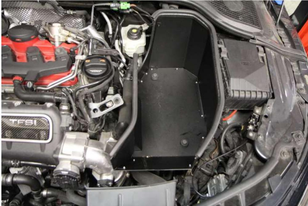
**Step 10:** Install the supplied M6x16 bolt and tighten using your 5mm socket allen.
