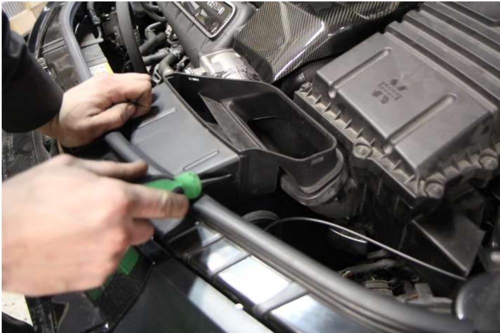
**Step 3:** Pull upwards on the engine cover to remove.
