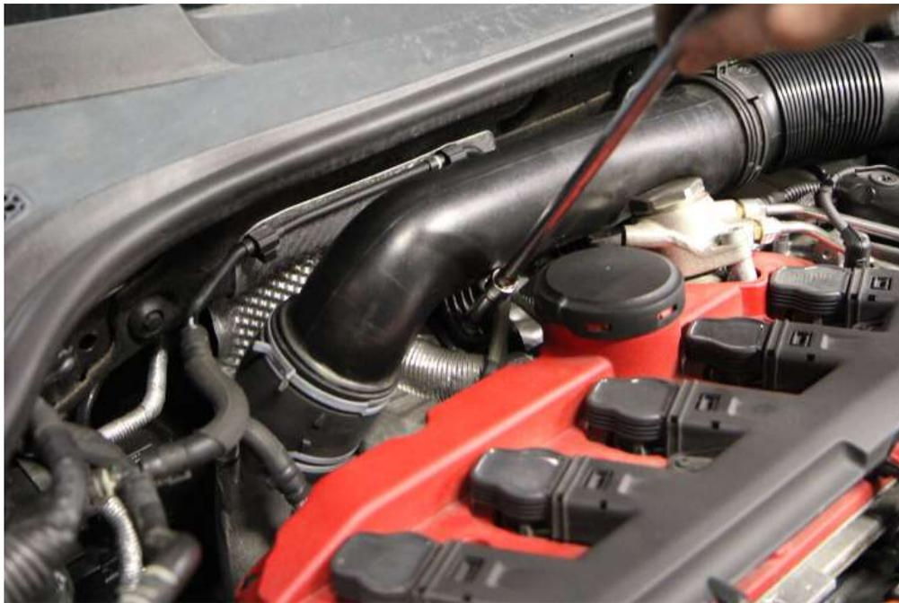
**Step 7:** Use your pipe clamp removal tool to release the OEM pipe from the stock silicone.
