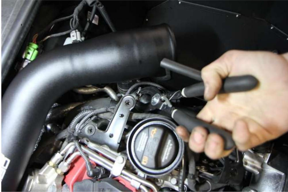
**Step 14:** Use your 5mm allen socket to install the M6x16 bolt securing the pipe to the engine.
