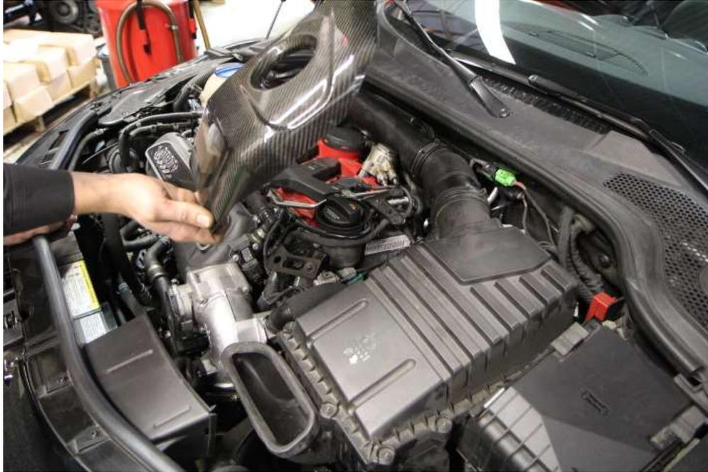
**Step 4:** Use your pipe clamp removal tool to release the rubber diverter valve outlet hose from the OEM pipe. Pull the rubber hose free.
