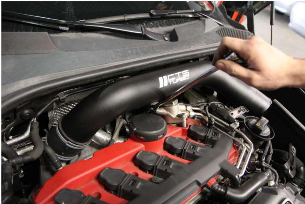
**Step 15:** Assemble the air filter assembly as shown. Tighten down all three gear clamps.
