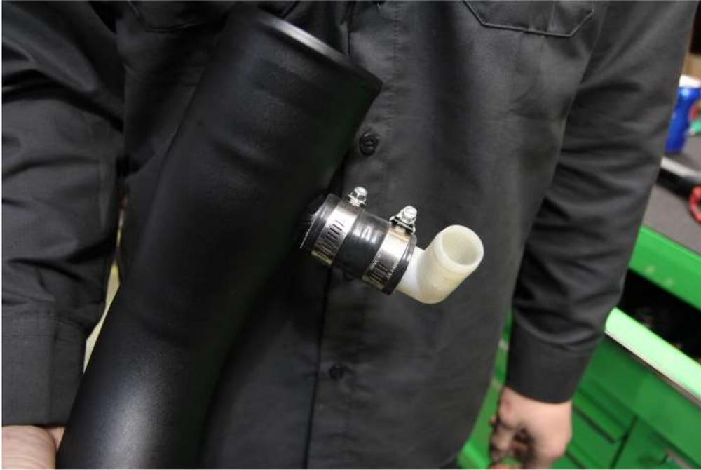
**Step 12:** Install the pipe into the car. Seat the left side of the CTS pipe into the OEM silicone. Reinstall the diverter valve outlet hose to the 90 degree elbow.
