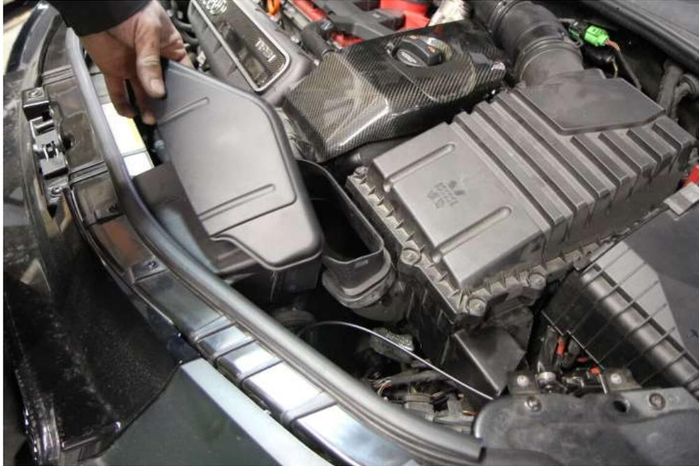
**Step 2:** Use your flat head screwdriver to pop the 2 clips on the left and right side holding the air inlet to the front assembly. Pull free.
