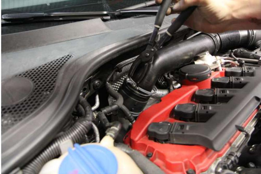
**Step 8:** Pull the entire airbox assembly out of the engine bay.
