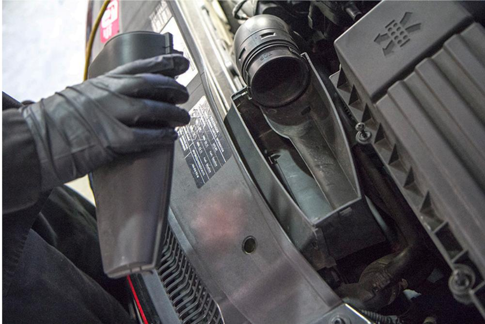
**Step 2:** Remove the MAF sensor cable by carefully undoing the clip. Using a pair of pliers, undo the spring clamp holding the MAF housing to the intake hose.
