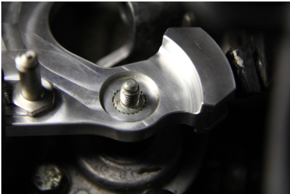
**Step 9:** Tighten the 13mm nut and confirm everything is connected. Inside the car, check the short shifter by shifting through ALL the gears. Make sure you are happy with the reduction in throw, change the pin position and test again.
