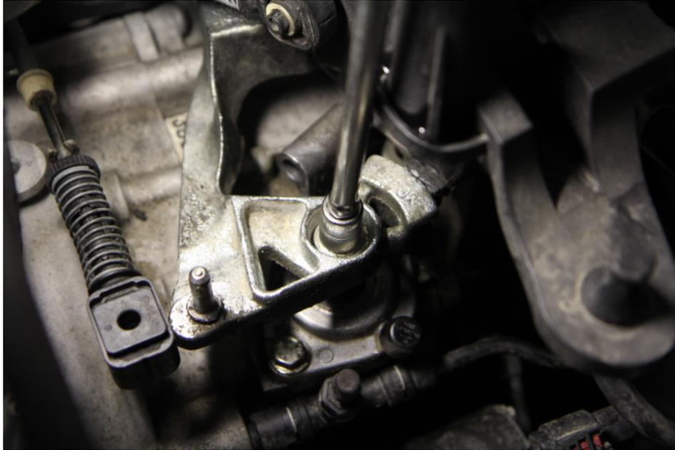
**Step 8:** Install the cable pin in the desired position. Outside bolt hole is 20% reduction. Inner bolt hole is 35% reduction. Align the splines of the weight with the transmission shaft spline.
