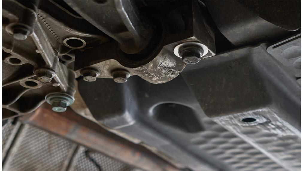
Control Arm Bracket Bolts M12 x 90 ----- 70 Nm (51 Ft-lbs) + 90 degrees
