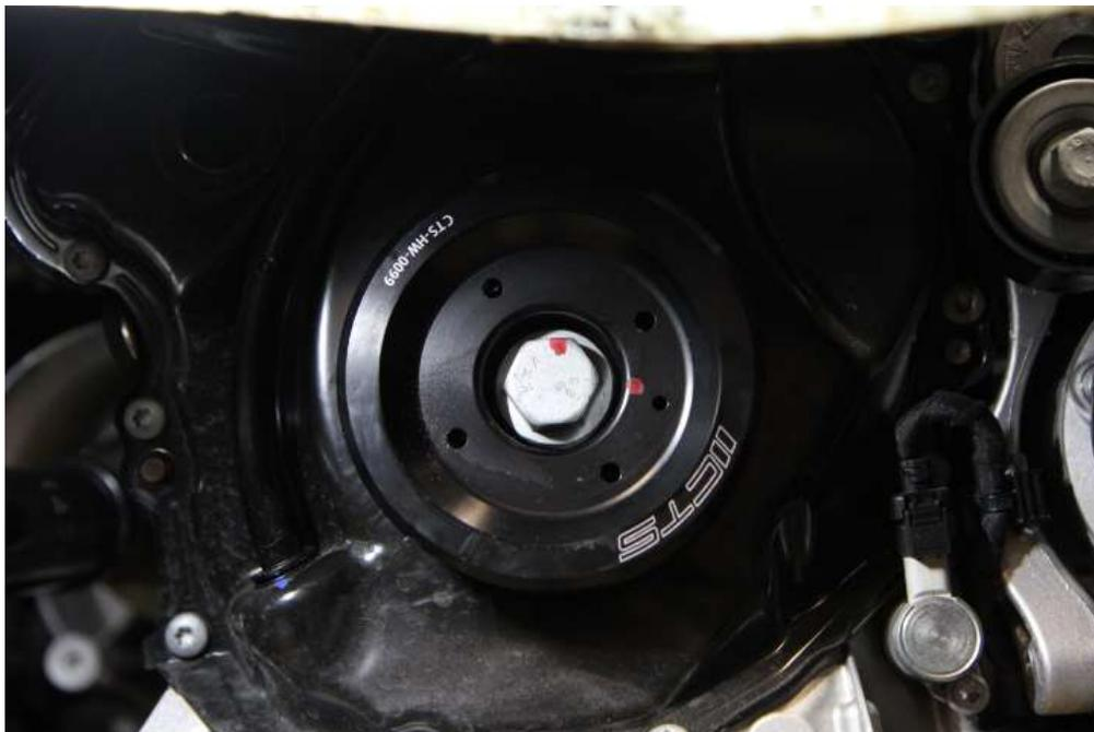
**Step 7:** Utilize your counter holder tool and long handle breaker bar with the 24mm socket to torque the bolt a ¼ turn further. With your two marks aligned, the pulley is installed.
