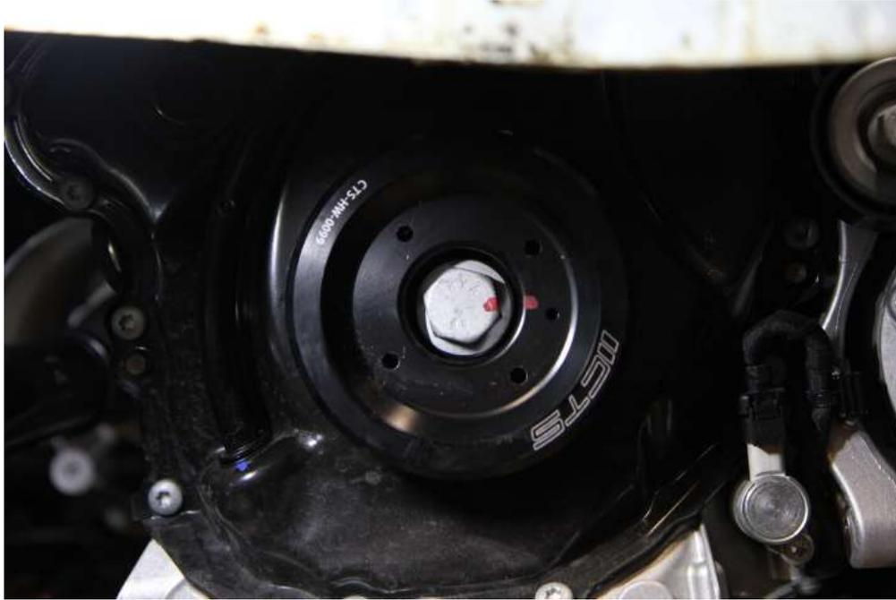
**Step 8:** Use your 16mm socket to release pressure on the belt tensioner and install the supplied shorter belt. Ensure the belt is sitting correctly in the pulley grooves.
