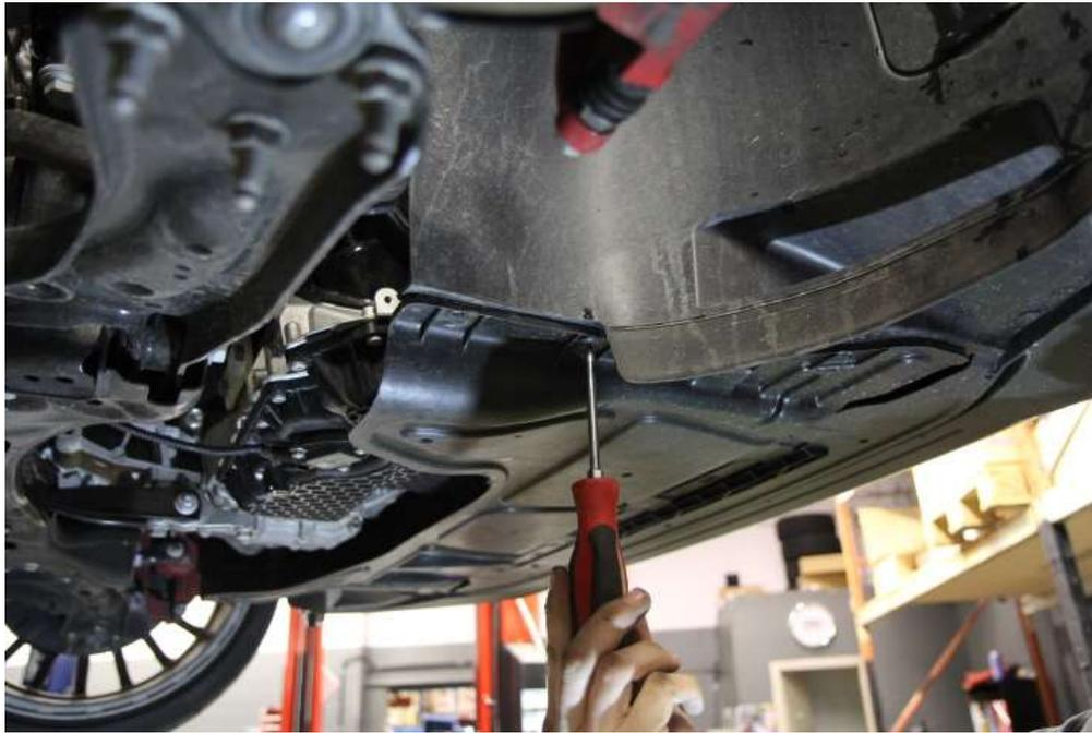
**Step 2:** Remove the passenger side wheel then remove the 6x T25 torx screws holding the passenger side lower inner fender liner to the car. Pull the liner free of vehicle.
