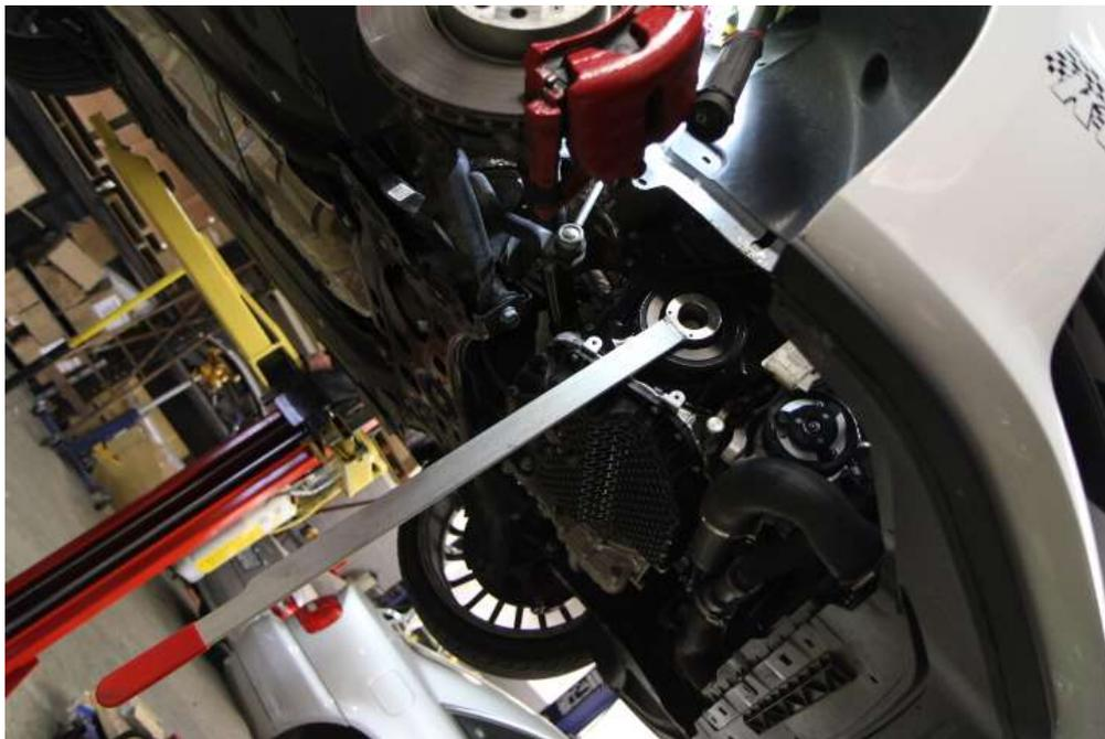
**Step 5:** Using your 24mm socket and breaker bar, loosen and remove the OEM crank pulley bolt. Remove pulley.
