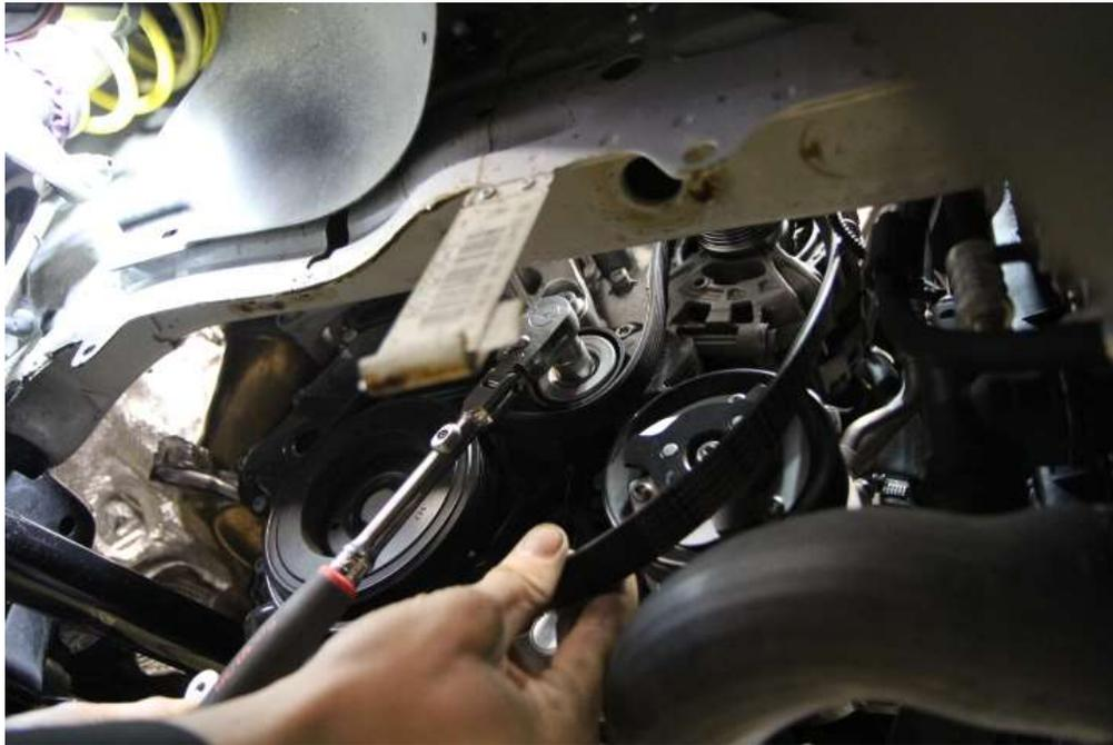
**Step 4:** Insert the counter holder tool T10355 into the 4 holes in the OEM pulley.
