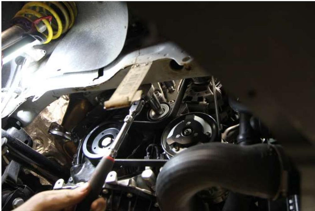
**Step 9:** Reverse steps 1 and 2 to reinstall the fender liner, passenger side wheel and belly pan. Start the vehicle and inspect the pulley while the engine is running to ensure it is running true.
