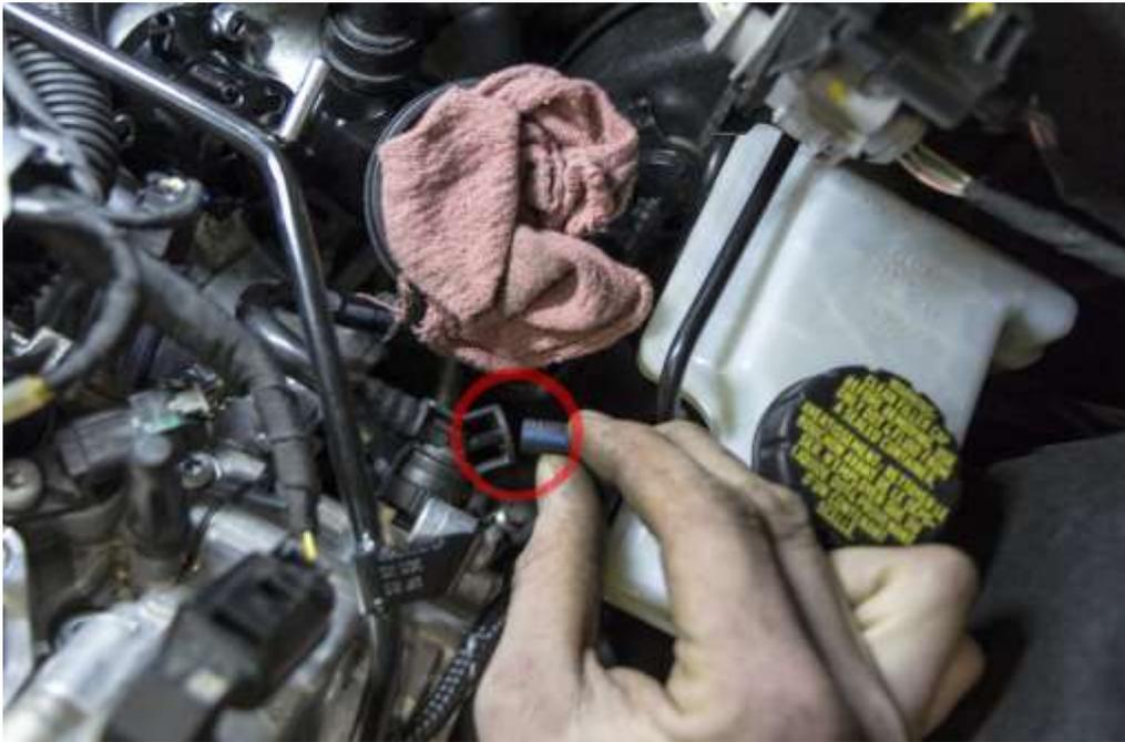
**Step 6:** Cut the included silicone line to the appropriate length and run the lines as shown. Install the diverter valve plug into the solenoid. Use a tie wrap to mount the control solenoid to the location shown. (shown in yellow)
