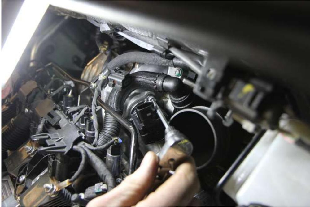
**Step 4:** Install the replacement CTS Turbo diverter valve assembly and tighten the 3x 5mm bolts.
