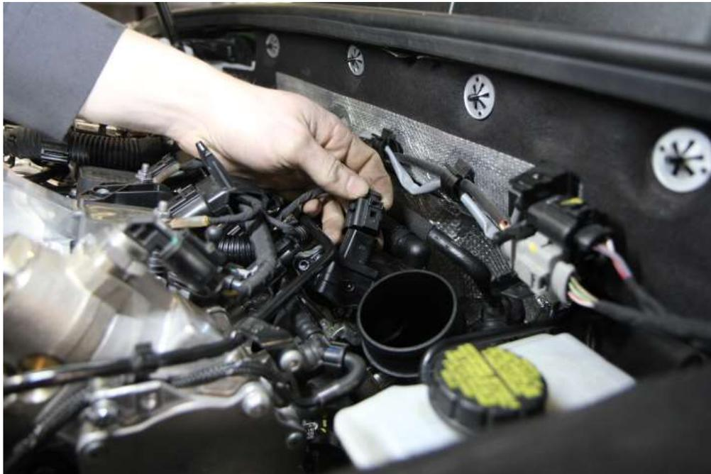
**Step 3:** Unscrew the 3x 5mm bolts holding the diverter valve to the engine. Pull the diverter valve out of the car. Ensure that no bolts fall into the intake.
