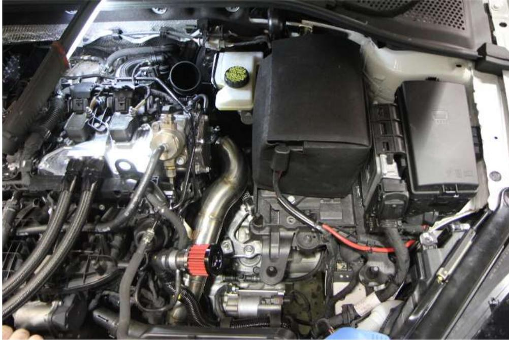
**Step 2:** Undo the OEM diverter valve plug.
