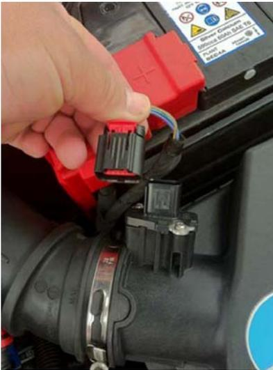
The first step in fitting your induction kit is to remove the stock air-box. Gently disconnect the MAF sensor, remembering to depress the red safety latch. This will allow the plug to be removed correctly, before loosening off the hose clip that connects the air-box lid to the inlet.
