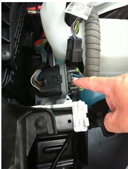
Down on the chassis leg, there is a large wiring loom connector attached to a plastic moulding. This is fixed on with a one-way catch and is awkward to remove. There is no need to split the loom at the connector, just remove it from the chassis leg.
