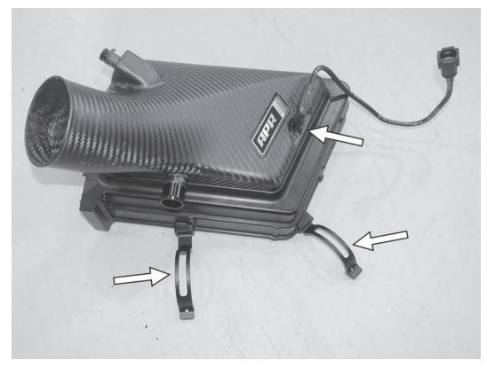
29) Install the factory vacuum line from the top of the airbox onto the APR airbox top in the same orientation. Install the supplied charge pipe brackets onto the APR airbox top as shown, with the longer bracket on the bottom and the shorter bracket on the side. Repeat on the other side of the car.
