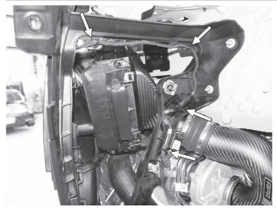
43) Reconnect the electrical connector for the oxygen sensor and then reattach it to the airbox frame. Connect the clips from the harness to the airbox frame. Repeat this on the other side of the car.
