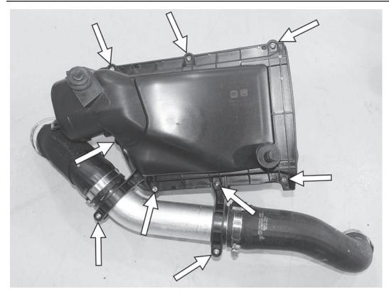
31) Assemble the APR airbox lid to the factory airbox base along with the charge pipe. Secure the APR airbox lid to the base with the seven supplied, short T25 screws and torque to 2Nm (18 in-lbs). Orient the charge pipe so it will connect with the turbo outlet and intercooler inlet, and then secure the charge pipe with the APR charge pipe brackets with the two supplied, long T25 screws and torque to 1Nm (9 in-lbs). Repeat on the other side of the car.
