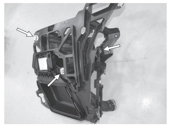
25) Disconnect the three clips holding the airbox to the airbox frame, and then separate the airbox from the frame. Repeat on the other side of the car.
