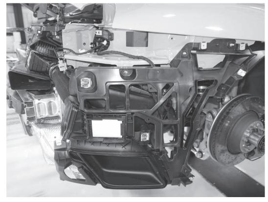
39) Reinstall the airbox frame and airbox assembly on the car, reconnecting all hoses to their original locations. Make sure the wiring harness is routed the same way as before and is not pinched. Repeat on the other side of the car.
