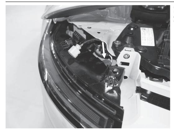
55) Reinstall both rear side taillights. Reconnect the electrical connectors on the lights before pushing them forward into their mounting locations.
