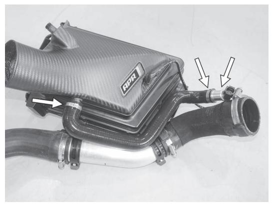
33) Install the APR silicone DV hose to the airbox with the supplied clamp, routing the hose as shown on the airbox. Install the supplied coupler on the other end of the DV hose, and secure with the other supplied clamp. Repeat on the other side of the car.
