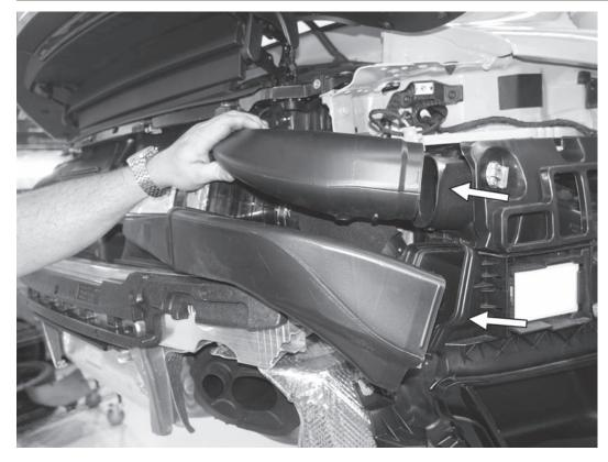
15) Pull off the two air guides, one for the airbox and one for the intercooler ducting. Separate from the airbox frame first, and then remove them from the car. Repeat on the other side of the car.
