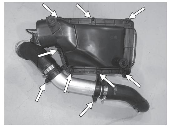
27) Remove the seven T25 screws holding the two halves of the airbox together. Note the orientation of the charge pipe on the airbox, and then remove the two T25 screws holding the charge pipe brackets to the charge pipe. Repeat on the other side of the car.
