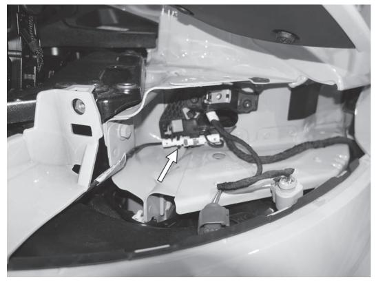
49) Reconnect the electrical connector from the right side of the rear bumper wiring harness to the area where the right taillight was. Some cars may have more or less electrical connectors depending on the vehicle options.
