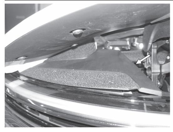
59) Snap back in the plastic panels on both sides of the rear decklid spoiler.
