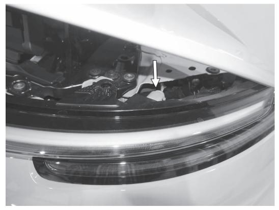
5) Pull the center taillight straight back a few inches from the car, exposing the electrical connectors. Disconnect both electrical connectors from either side of the center taillight and remove the taillight from the car.
