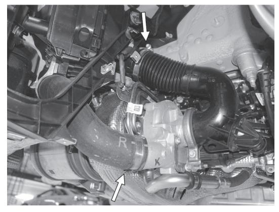
17) Loosen the 7mm clamps from the top of the turbo inlet pipe and the turbo outlet pipe. Separate the hose from both connections. Repeat this step on the other side of the car.
