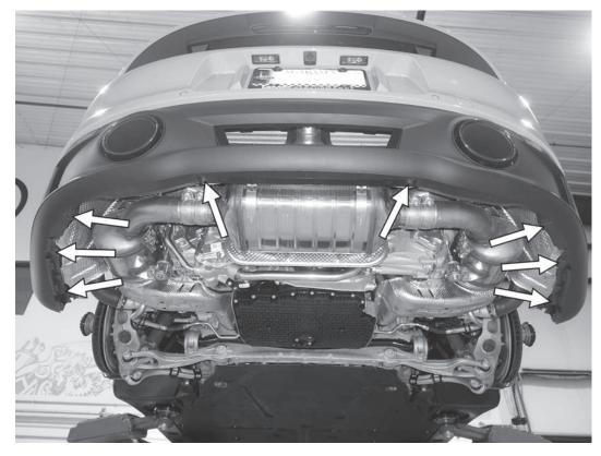
51) Reinstall the eight T30 screws from the bottom of the rear bumper. Make sure to put the correct screws in the same locations they were removed from. Tighten the screws to 3.2Nm (28 in-lbs).
