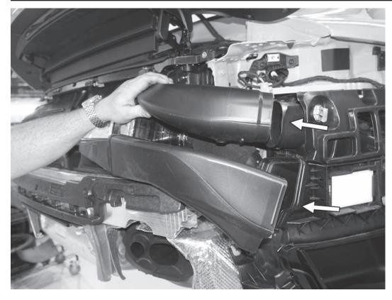
47) Install the two air guides back onto the car, one for the airbox and one for the intercoller ducting. Repeat on the other side of the car.
