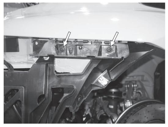
21) Remove the two T30 screws from the bumper guide clip, and remove the bumper guide clip from the car. Repeat on the other side of the car.
