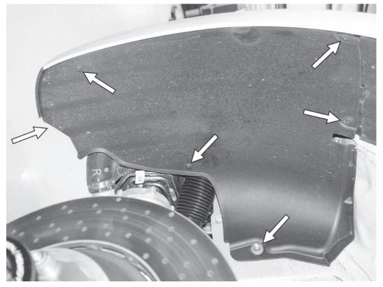
53) Reinstall the rear lower fender liner. Secure with the four T25 screws, the one T30 screw (underneath), and the one 10mm nut. Tighten the 10mm nut to 2.5Nm (22 in-lbs). Tighten the T30 screw underneath to 2Nm (18 in-lbs). Tighten the four T25 screws to 3.2Nm (28 in-lbs). Repeat on the other side of the car.
