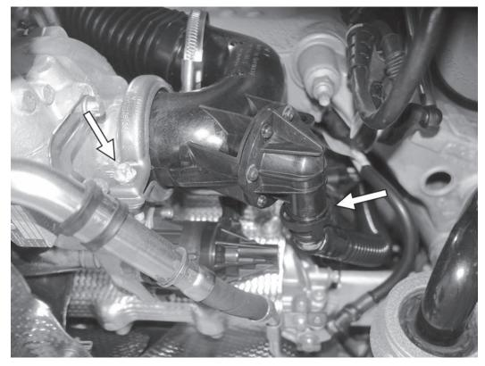
35) Loosen the clamp on the turbo inlet pipe by remove the E10 external torx fastener. Repeat on the other side of the car. On the right turbo, disconnect the PCV line on the turbo inlet pipe.
