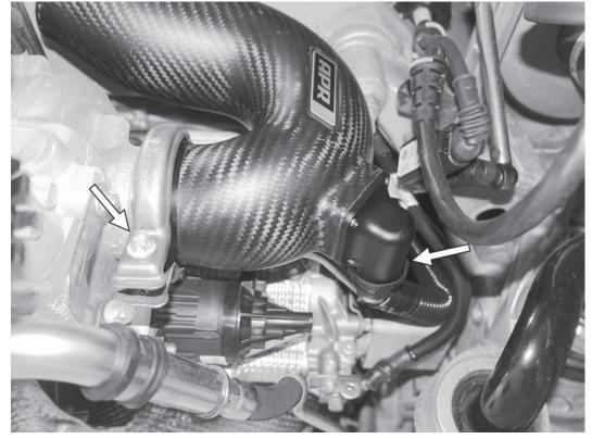
37) Install the APR turbo inlet pipe onto the turbocharger, and secure with the factory clamp. Loosely tighten the E10 external torx screw so the pipe can be adjusted. Repeat on the other side of the car. On the right turbo, reconnect the PCV line to the port on the APR turbo inlet pipe.
