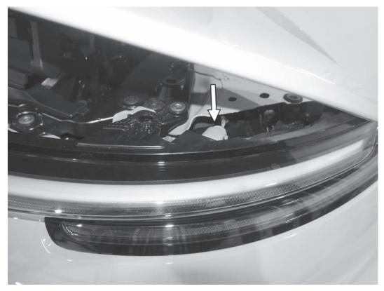
57) Place the center taillight back onto the car, and then reconnect the electrical connectors on both sides of the light. Push the taillight forward into its mounting location.
