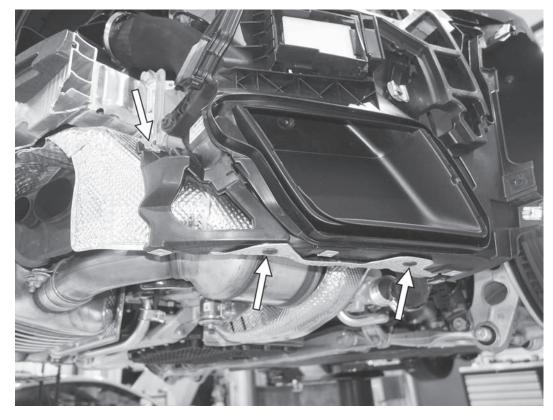
45) Reinstall the four T30 screws (two shown) holding the heat shield to the bottom of the airbox frame. Tighten the screws to 2.5Nm (22 in-lbs). Repeat on the other side of the car.
