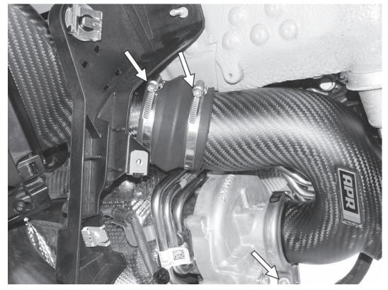
41) Connect the coupler from the APR turbo inlet pipe to the APR airbox lid. Once centered, tighten the two 7mm clamps to 2Nm (18 in-lbs). Tighten the E10 external torx screw on the APR turbo inlet pipe to 5.5Nm (49 in-lbs). Repeat on the other side of the car.
