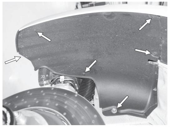
9) On the rear lower fender liner, remove the four T25 screws, the one T30 screw (underneath), and the one 10mm nut. Remove the rear lower fender liner from the car. Repeat on the other side of the car.
