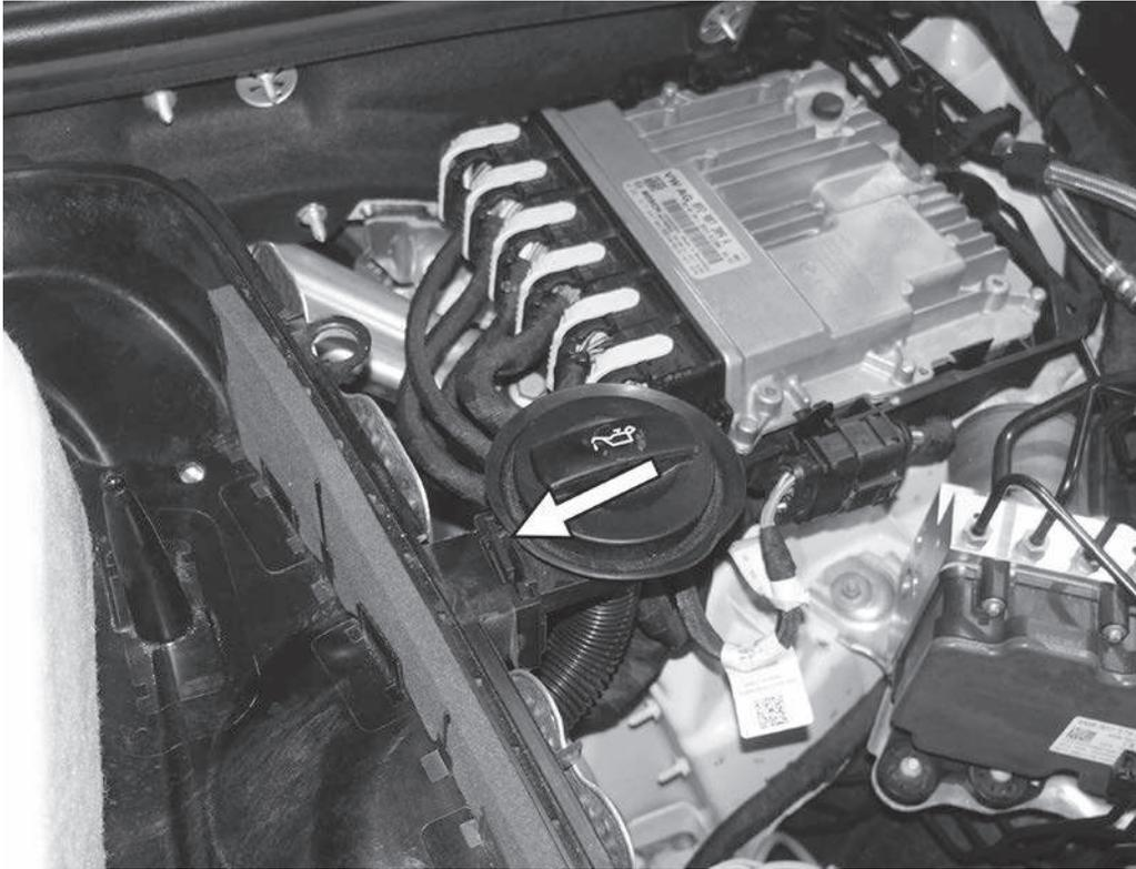
3) Push in the tab next to the oil fill cap, and then lift the oil fill tube and cap assembly up and away from the airbox base.
