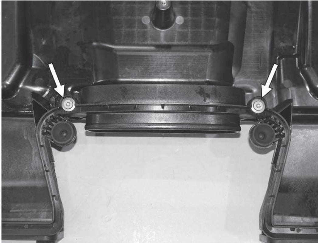
31) Install the APR airbox adapter to the factory airbox base with the two original T25 screws. Tighten both screws to 5Nm (44 in-lbs).
