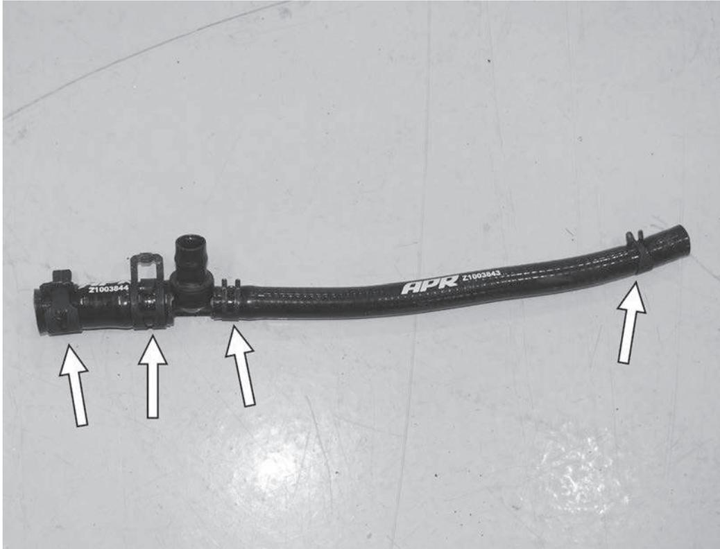
21) Build two of the shown hose assemblies with the APR EVAP suction jet, two large and two small hose clamps and hose.
