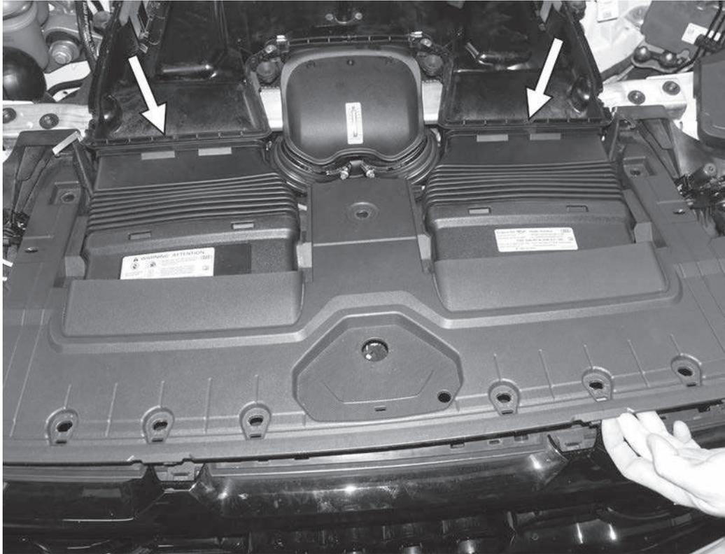
7) Lift up on the front of the front cover, then pull the cover forward. Separate the cover where the accordion ducts meet the bottom of the airbox.
