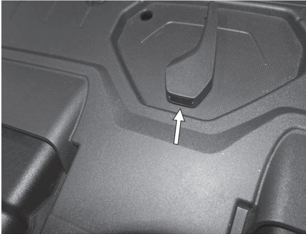
5) Press in on the button on the back of the hood latch, and then lift up on the hood latch to remove it from the car. Make sure to NOT close the hood without reinstalling the hood latch again!
