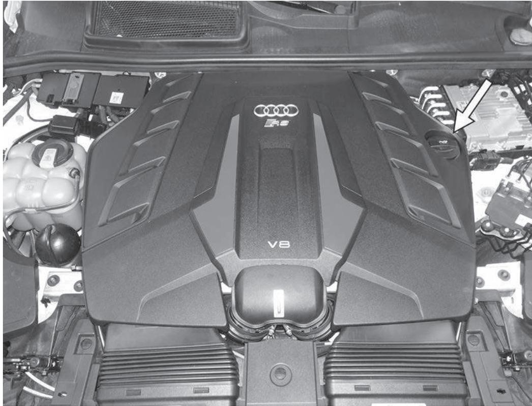
1) Raise the hood, then remove the oil fill cap.
