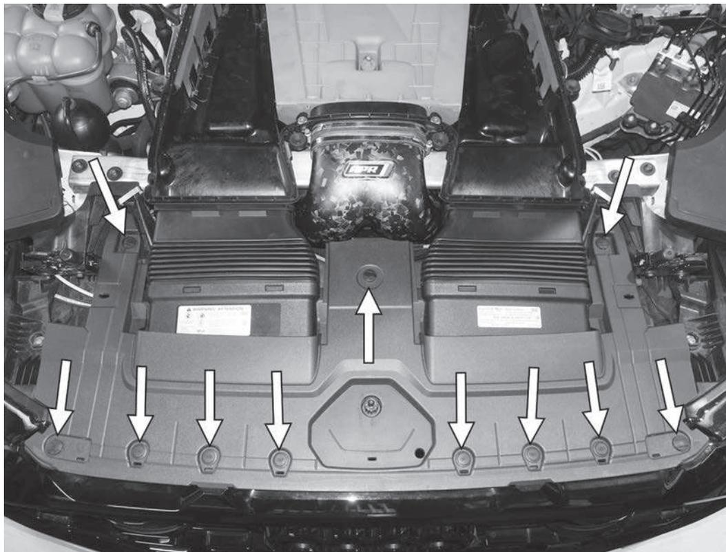
37) Reinstall the eleven push pin connectors holding the front panel to the car. Make sure to install the pins in the same location as they were originally.
