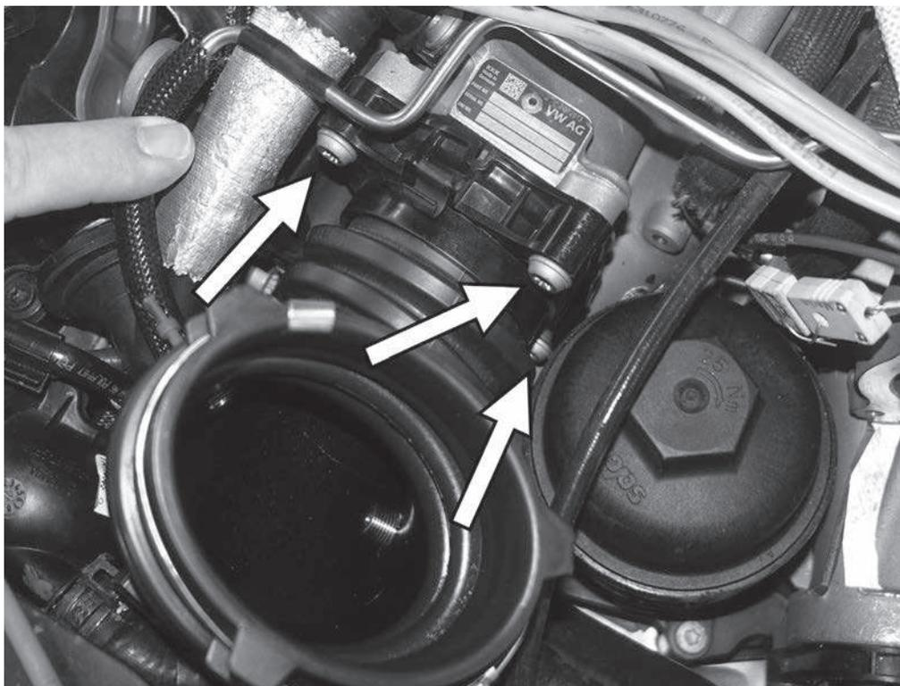
19) Remove the three T30 screws from the right inlet flange to the right turbo.
