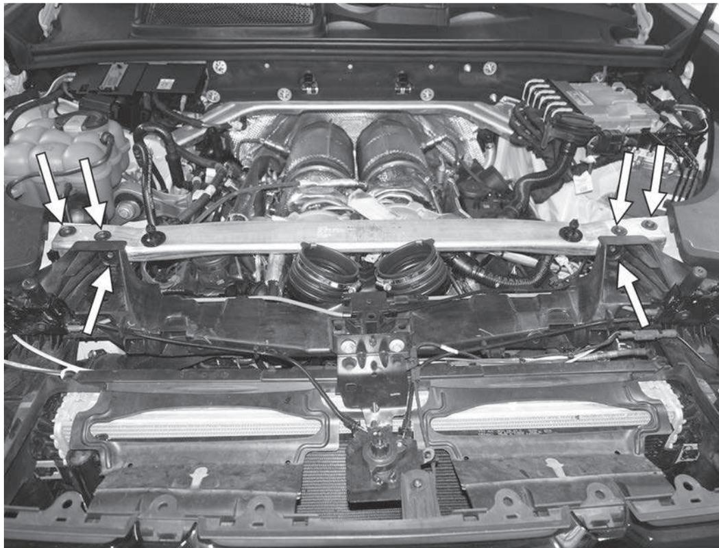
11) Remove the six T30 screws holding the front crossbrace in the engine compartment.
